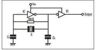
IC(MG,MT):1/6TC4069UBPx 2 (MX) :1/6TC74HCU04x2 C1C2(MG,MT):30pF (MX) :30pF(13.01~20.0MHz) 15pF(20.01~25.99MHz) 5pF(26.00~50.00MHz) X: Ceramic Resonator Vpo(MG,MX): +5V (MT) : +12V
