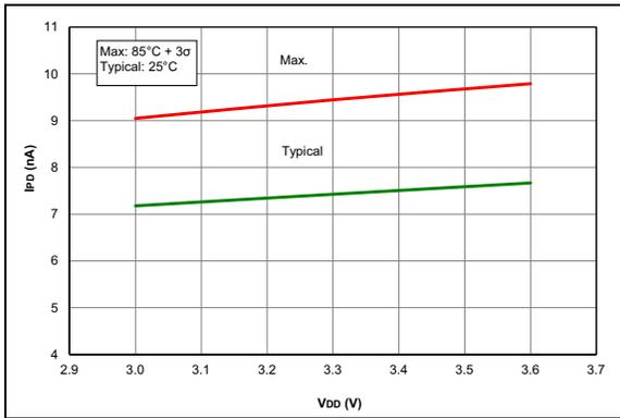
**FIGURE 36-31:**  $I_{PD}$ , Brown-Out Reset (BOR),  $BORV = 1$ , PIC16LF1615/9 Only.
