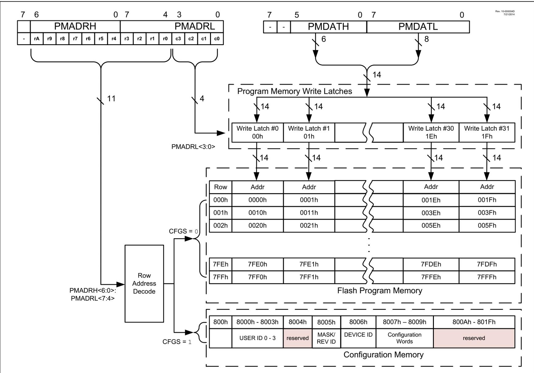
FIGURE 10-6: FLASH PROGRAM MEMORY WRITE FLOWCHART
