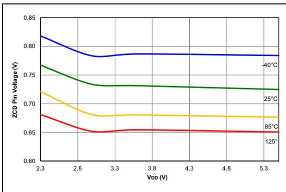
**FIGURE 36-105:** ZCD Pin Voltage, Typical Measured Values.
