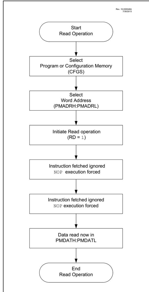
**FIGURE 10-2: FLASH PROGRAM MEMORY READ CYCLE EXECUTION**
