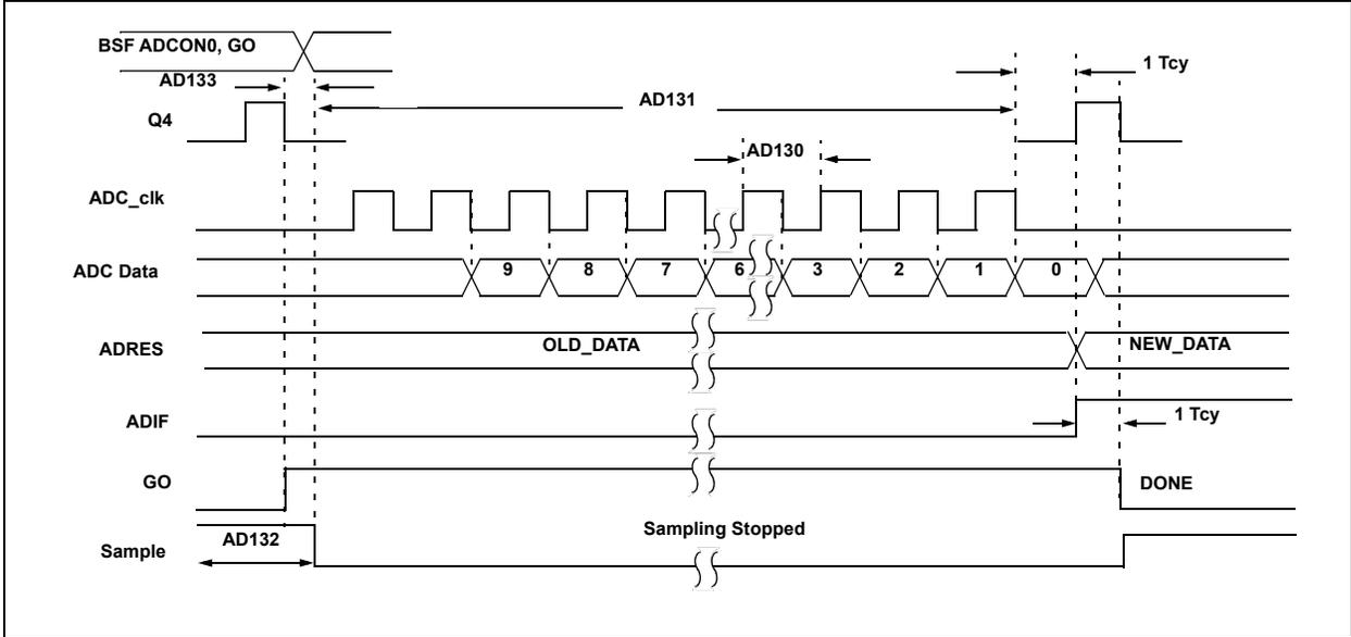
FIGURE 35-12: ADC CONVERSION TIMING (ADC CLOCK FROM FRC)
