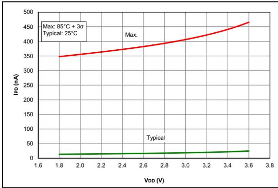
**FIGURE 36-37:**  $I_{PD}$ , ADC Non-Converting, PIC16LF1615/9 Only.
