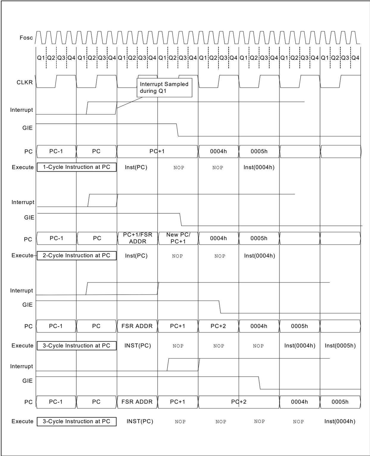
**FIGURE 7-3: INT PIN INTERRUPT TIMING**
