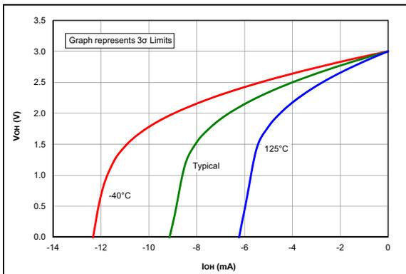
**FIGURE 36-45:**  $V_{OH}$  vs.  $I_{OH}$  Over Temperature,  $V_{DD} = 3.0V$ .
