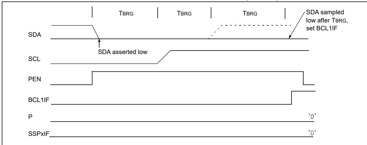
**FIGURE 24-39: BUS COLLISION DURING A STOP CONDITION (CASE 2)**
