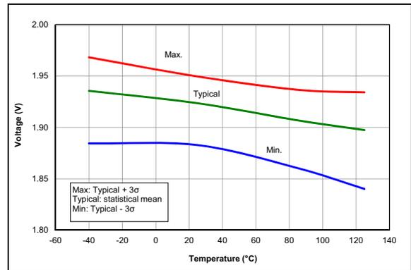
**FIGURE 36-53:** Brown-Out Reset Voltage, Low Trip Point ( $BORV = 1$ ), PIC16F1615/9 Only.
