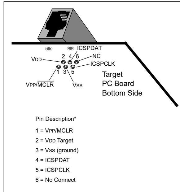
Another connector often found in use with the PICKit™ programmers is a standard 6-pin header with 0.1 inch spacing. Refer to [Figure 33-2](#).
