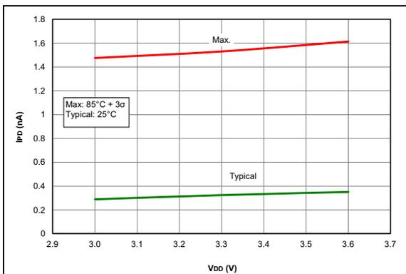
**FIGURE 36-33:**  $I_{PD}$ , LP Brown-Out Reset ( $LPBOR = 0$ ), PIC16LF1615/9 Only.
