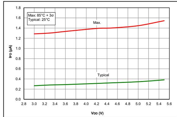
**FIGURE 36-34:**  $I_{PD}$ , LP Brown-Out Reset ( $LPBOR = 0$ ), PIC16F1615/9 Only.
