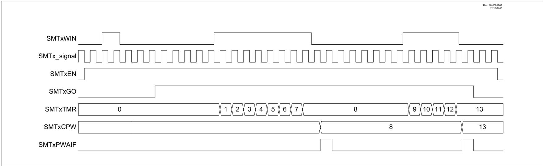
**FIGURE 29-20: GATED COUNTER MODE SINGLE ACQUISITION TIMING DIAGRAM**
