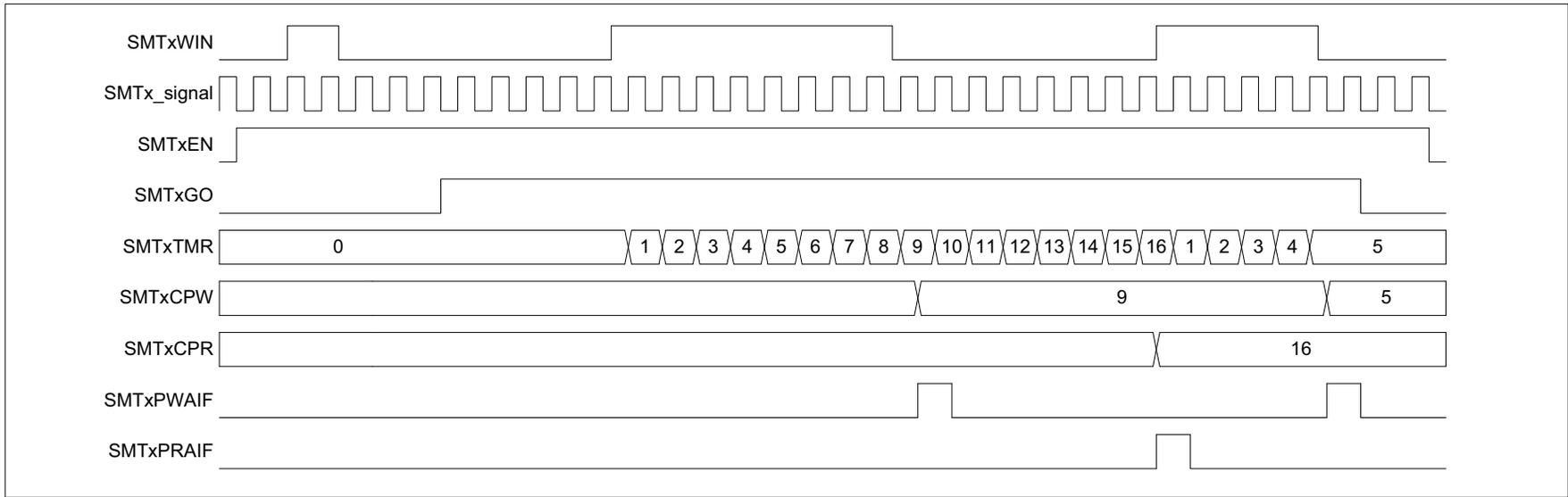
**FIGURE 29-22: WINDOWED COUNTER MODE SINGLE ACQUISITION TIMING DIAGRAM**
