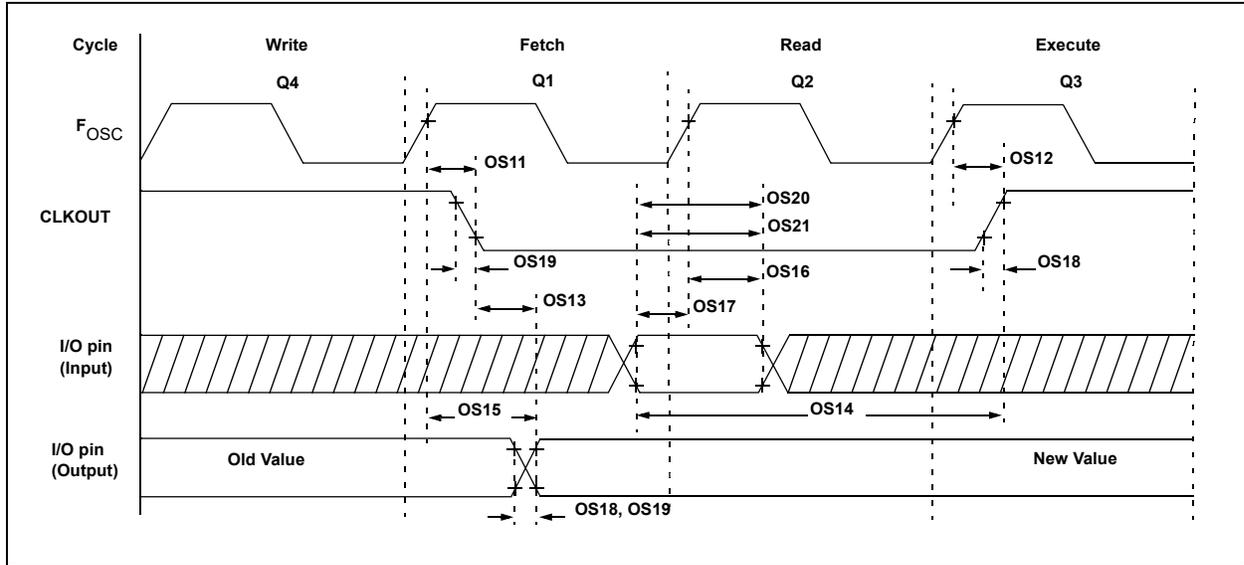
**TABLE 35-10: CLKOUT AND I/O TIMING PARAMETERS**
