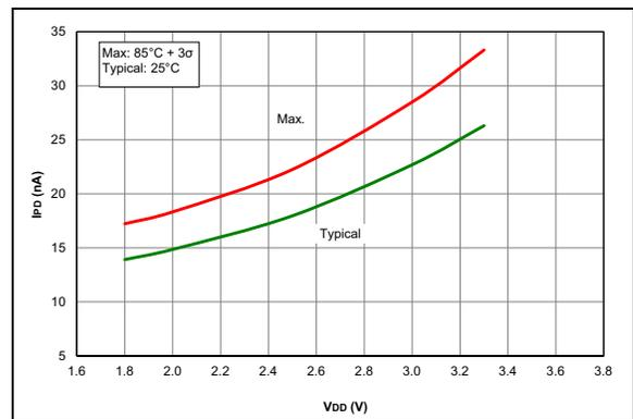
**FIGURE 36-29:**  $I_{PD}$ , Fixed Voltage Reference (FVR), PIC16LF1615/9 Only.
