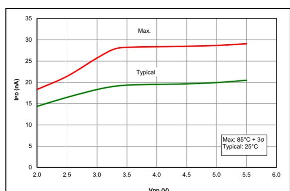
**FIGURE 36-30:**  $I_{PD}$ , Fixed Voltage Reference (FVR), PIC16F1615/9 Only.
