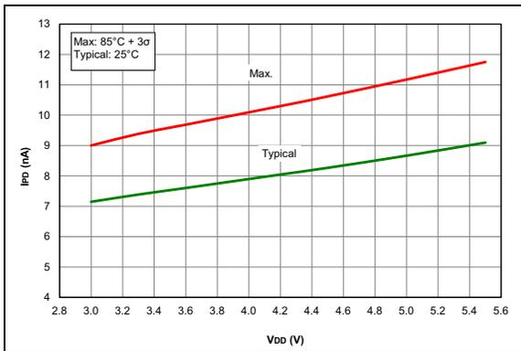
**FIGURE 36-32:**  $I_{PD}$ , Brown-Out Reset (BOR),  $BORV = 1$ , PIC16F1615/9 Only.
