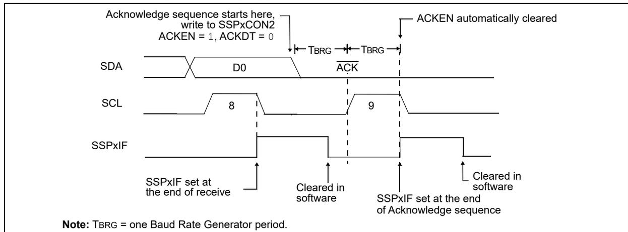
**FIGURE 24-31: STOP CONDITION RECEIVE OR TRANSMIT MODE**
