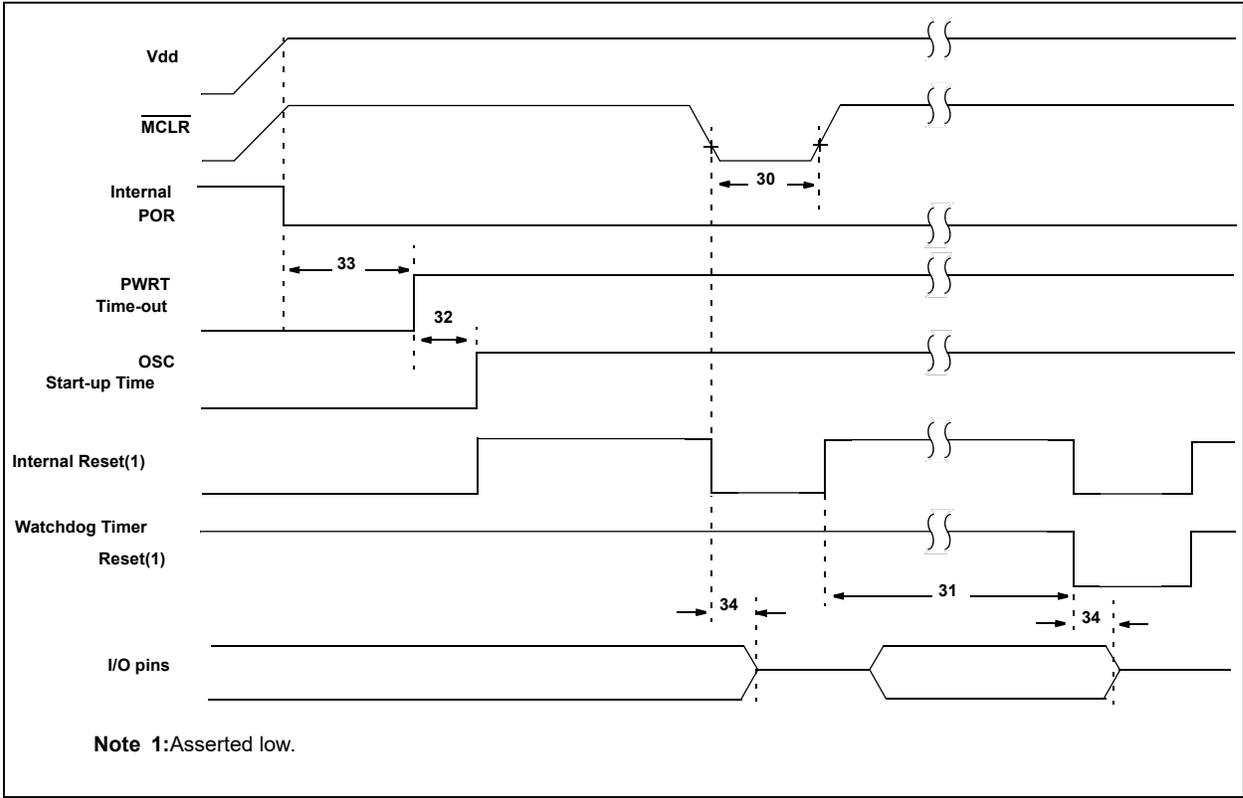
**TABLE 35-11: RESET, WATCHDOG TIMER, OSCILLATOR START-UP TIMER, POWER-UP TIMER AND BROWN-OUT RESET PARAMETERS**
