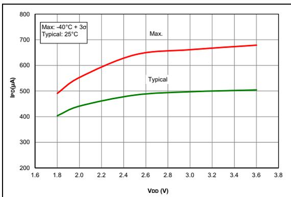
**FIGURE 36-39:**  $I_{PD}$ , Comparator, NP Mode ( $CxSP = 1$ ), PIC16LF1615/9 Only.
