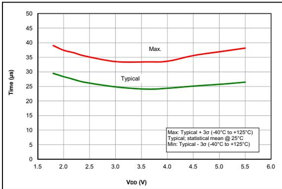
**FIGURE 36-67:** Wake From Sleep,  $V_{REGPM} = 1$ .
