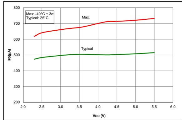
**FIGURE 36-40:**  $I_{PD}$ , Comparator, NP Mode ( $CxSP = 1$ ), PIC16F1615/9 Only.
