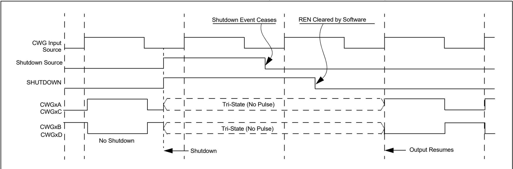
**FIGURE 28-14: SHUTDOWN FUNCTIONALITY, AUTO-RESTART ENABLED (REN = 1, LSAC = 01, LSBD = 01)**
