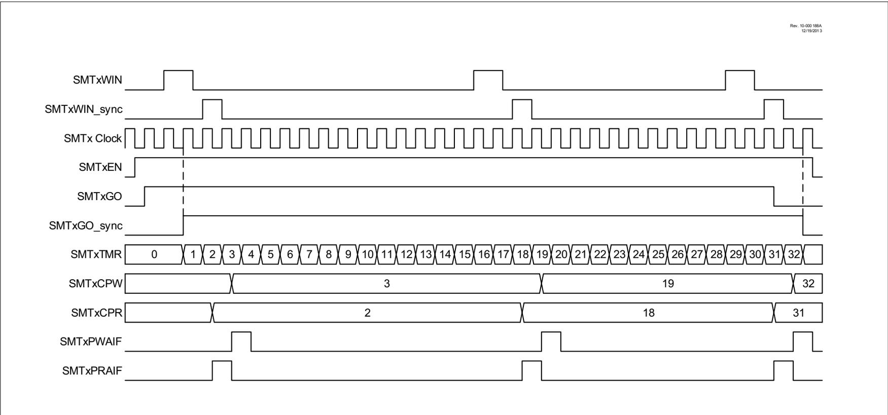
**FIGURE 29-17: CAPTURE MODE SINGLE ACQUISITION TIMING DIAGRAM**
