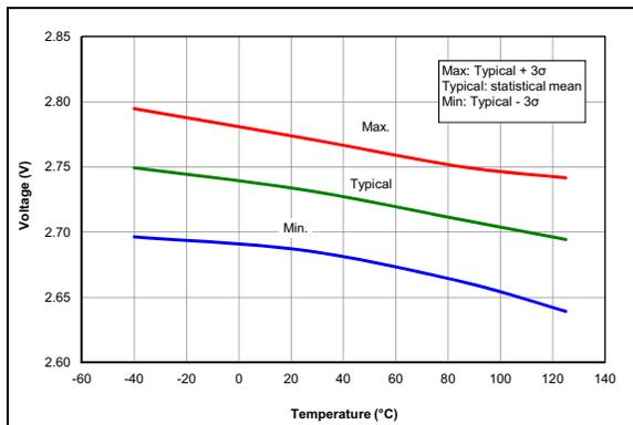
**FIGURE 36-57:** Brown-Out Reset Voltage, High Trip Point ( $BORV = 0$ ).
