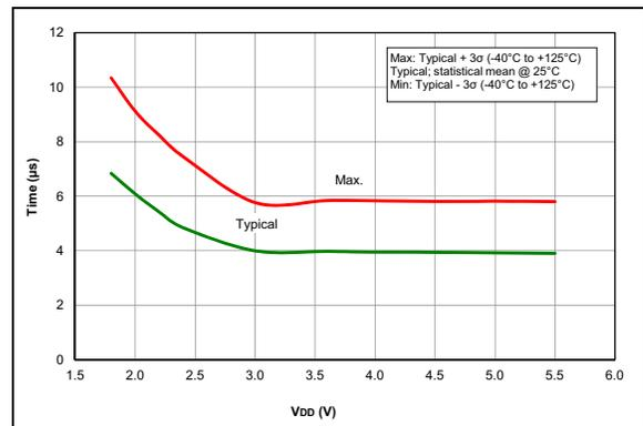
**FIGURE 36-66:** Wake From Sleep,  $V_{REGPM} = 0$ .
