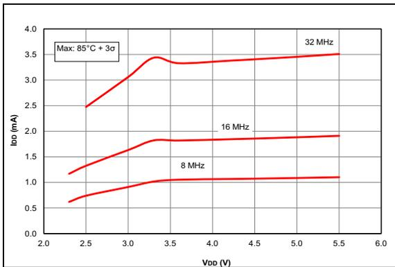
**FIGURE 36-20:**  $I_{DD}$  Maximum, HFINTOSC Mode, PIC16F1615/9 Only.
