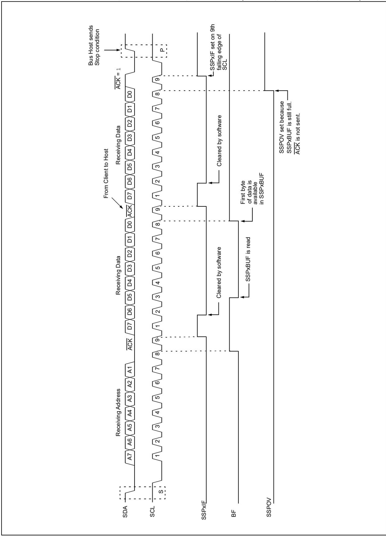
FIGURE 24-15: I<sup>2</sup>C CLIENT, 7-BIT ADDRESS, RECEPTION (SEN = 1, AHEN = 0, DHEN = 0)
