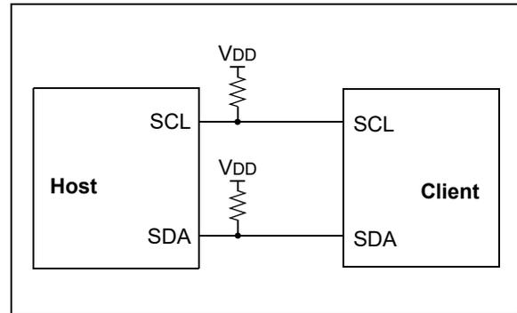
The Acknowledge bit (ACK) is an active-low signal, which holds the SDA line low to indicate to the transmitter that the client device has received the transmitted data and is ready to receive more.
