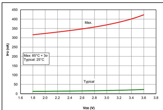
**FIGURE 36-27:**  $I_{PD}$  Base, LP Sleep Mode, PIC16LF1615/9 Only.
