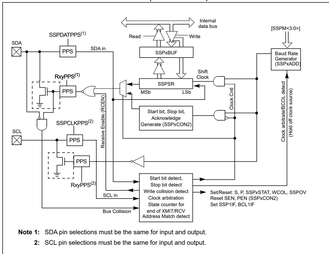
FIGURE 24-3: MSSP BLOCK DIAGRAM (I<sup>2</sup>C CLIENT MODE)
