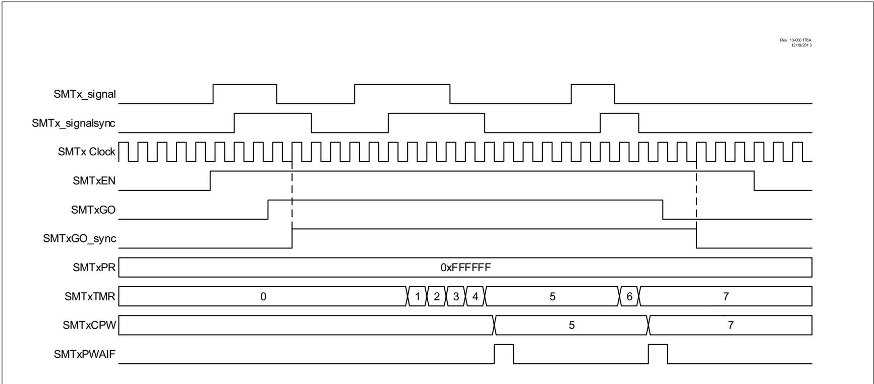
**FIGURE 29-5: GATED TIMER MODE SINGLE ACQUISITION TIMING DIAGRAM**
