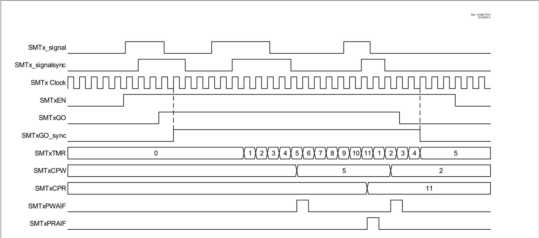
**FIGURE 29-7: PERIOD AND DUTY-CYCLE SINGLE ACQUISITION TIMING DIAGRAM**
