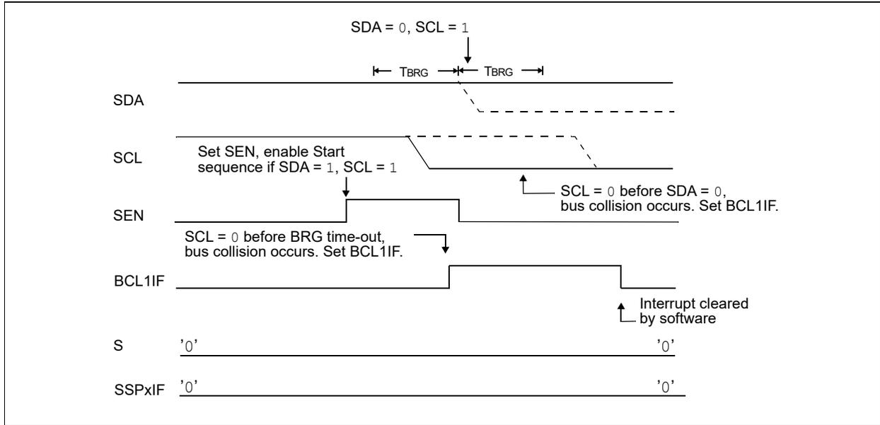
**FIGURE 24-35: BRG RESET DUE TO SDA ARBITRATION DURING START CONDITION**
