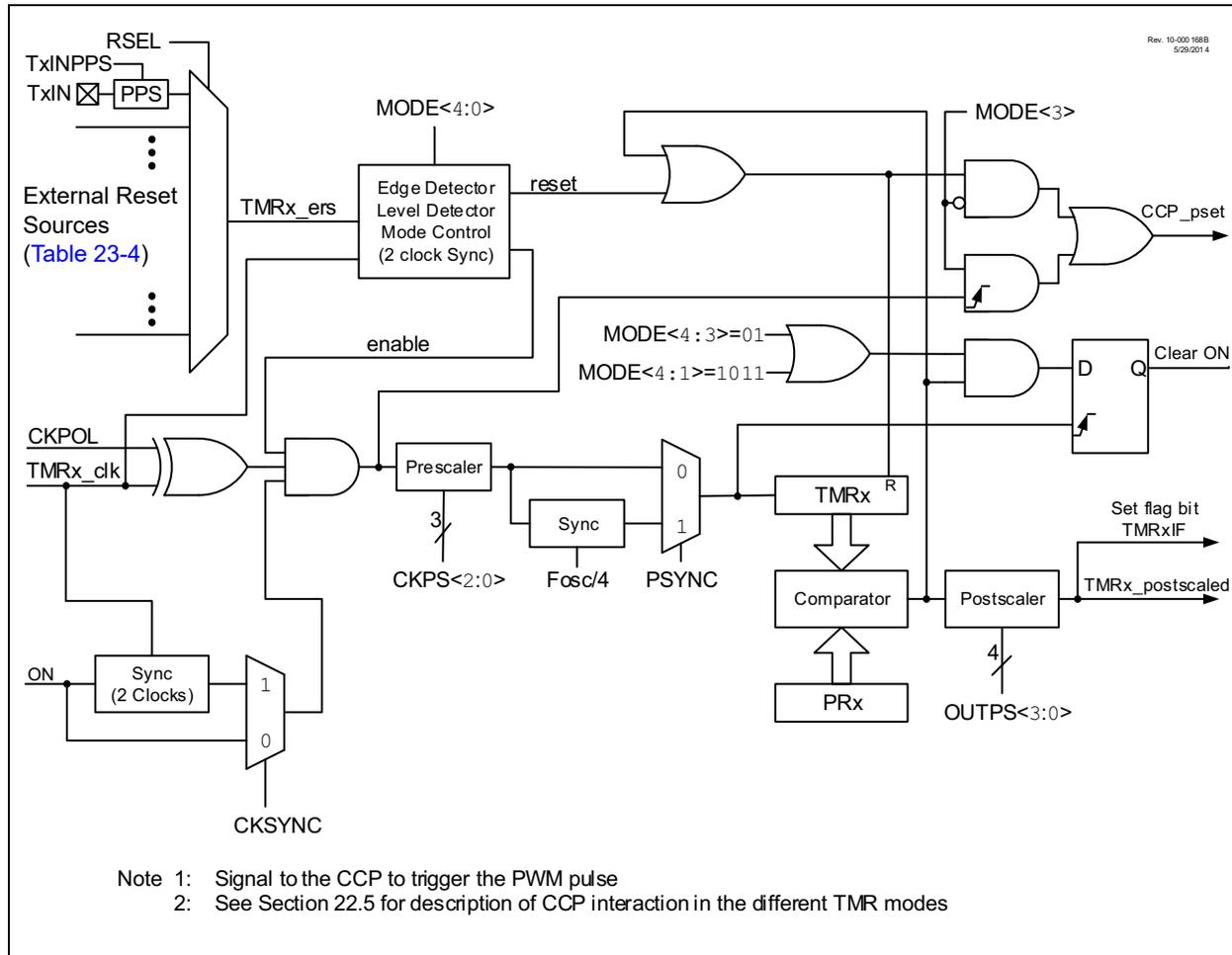
**FIGURE 23-2: TIMER2 CLOCK SOURCE BLOCK DIAGRAM**
