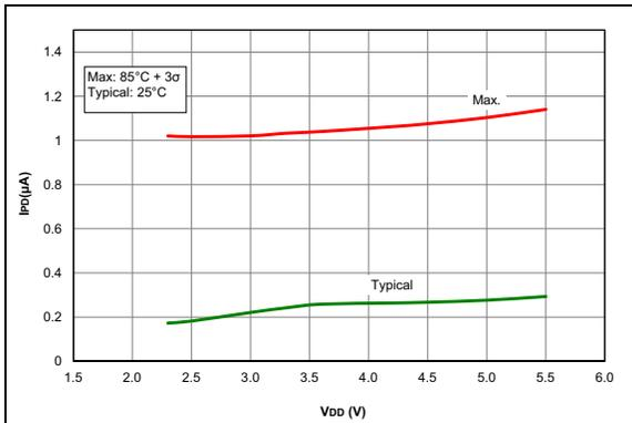
**FIGURE 36-38:**  $I_{PD}$ , ADC Non-Converting, PIC16F1615/9 Only.
