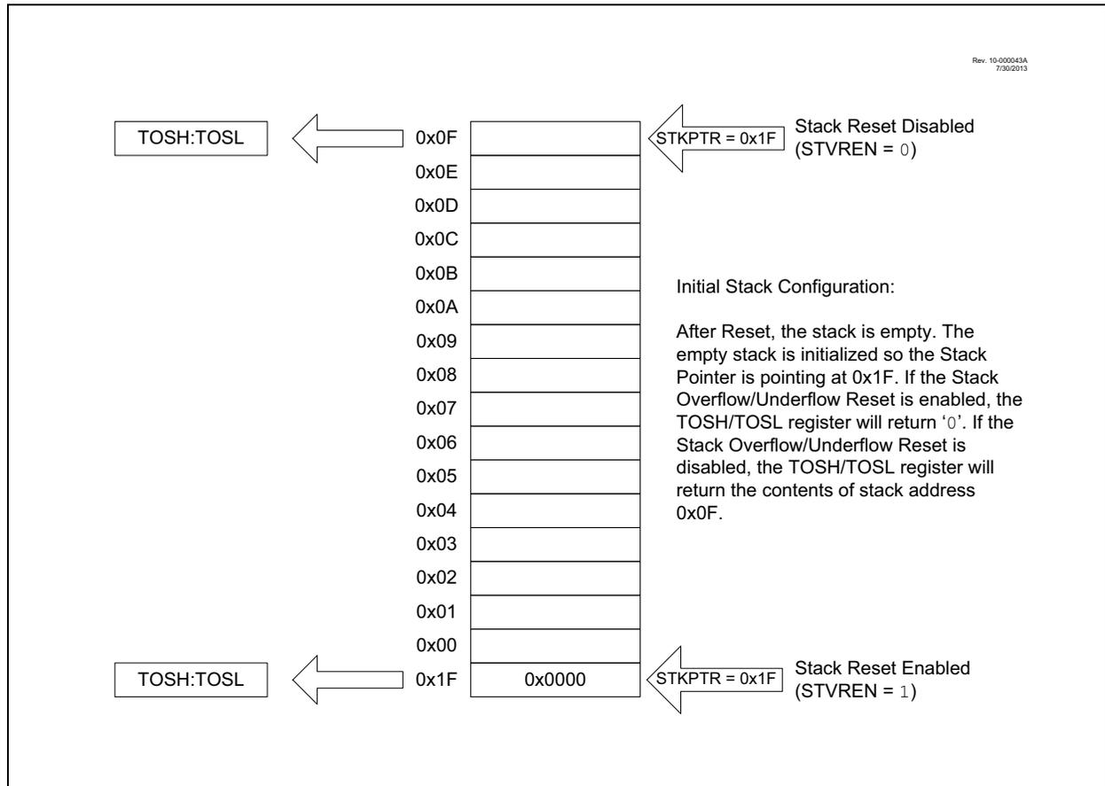
FIGURE 3-5: ACCESSING THE STACK EXAMPLE 2
