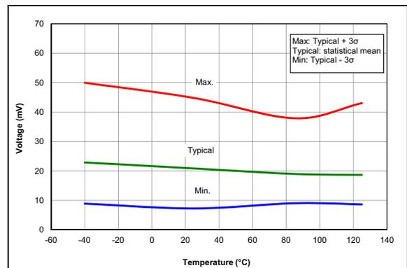
**FIGURE 36-54:** Brown-Out Reset Hysteresis, Low Trip Point ( $BORV = 1$ ), PIC16F1615/9 Only.
