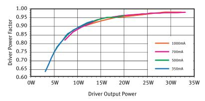
NB. Low power driver available at 350mA & 700mA to improve efficiency for output loading of 10W and below.
