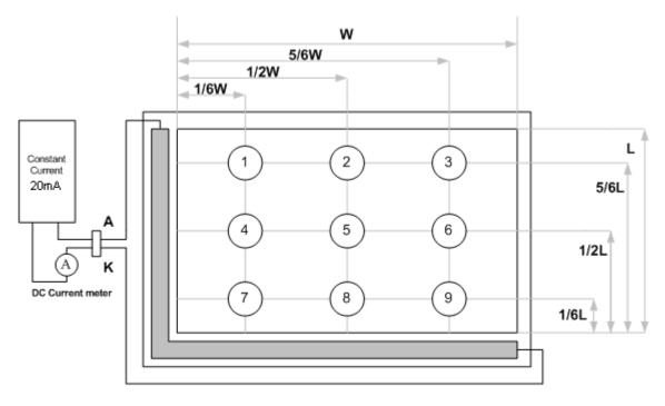
Note3: The Uniformity definition (Min Brightness / Max Brightness) x 100%
