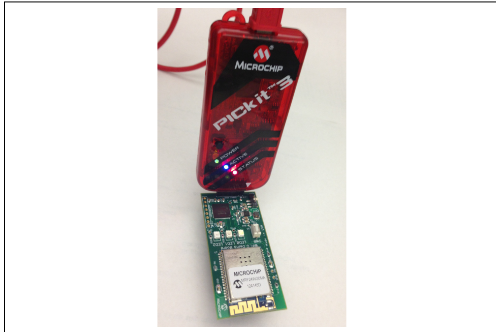
FIGURE 5-3: Wi-Fi® G DEMO BOARD – PICKit™ 3 HARDWARE INTERFACE
