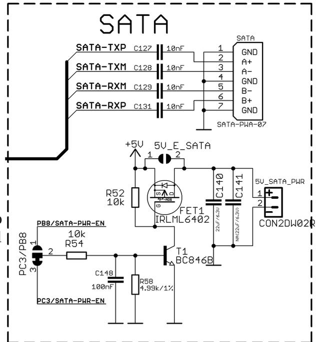
To keep the low form factor we have placed the small JST connector.
