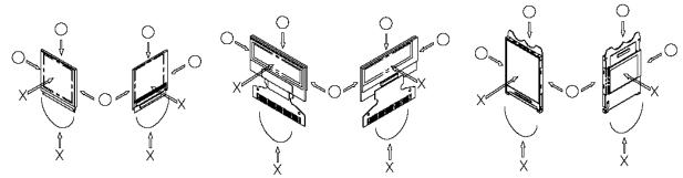
(7) Do not apply stress to the LSI chips and the surrounding molded sections.
