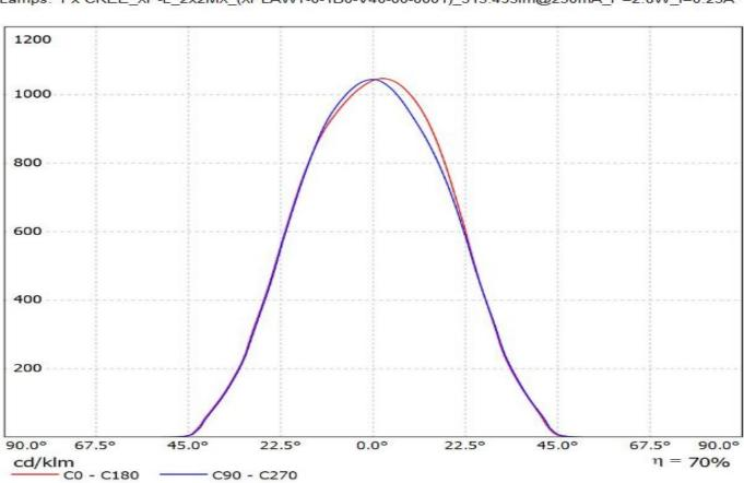
Luminaire: Ledil FC14975\_FLORENTINA-2X2-W\_(XP-L) Lamps: 1 x CREE\_XP-L\_2x2MX\_(XPLAWT-0-1B0-V40-00-0001)\_515.493Im@250mA\_P=2.8W\_I=0.25A
