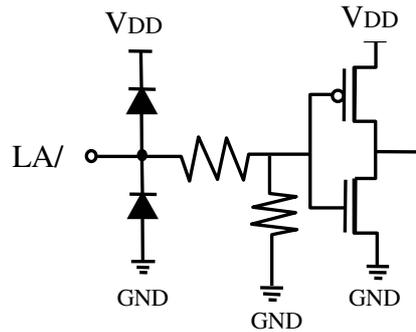
**Equivalent Circuits of Inputs (2)**
