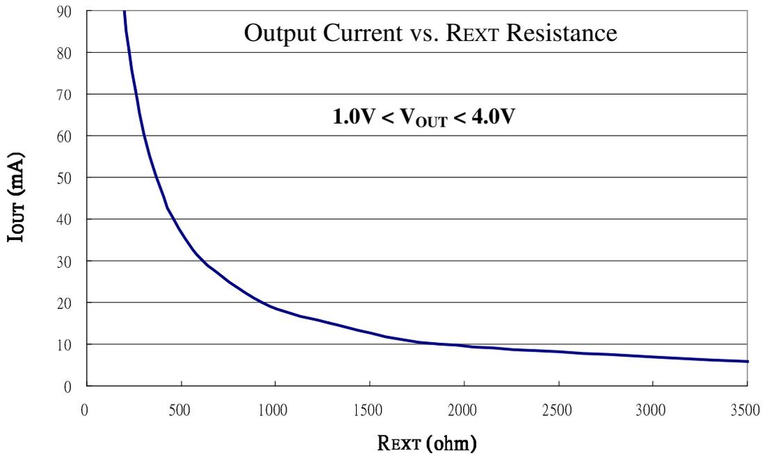
Also, when SCT2026's output voltage is set between 1V and 4V, the output current  $I_{OUT}$  can be set by the formula:  $I_{OUT} = 30(630 / R_{EXT})$  mA. Thus the output currents are all set to 21mA ( $\pm 6\%$ ) by set the reference value  $R_{EXT} = 900\Omega$ .
