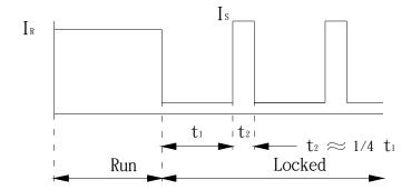
3rd wire signal Run : Square Wave Locked :  $V_{\text{H}}$  or  $V_{\text{L}}$
