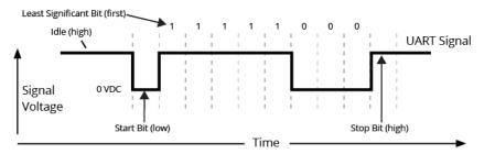
Serial communications depend on the two UARTs (the microcontroller's and the RF Module's) to be configured with compatible settings (baud rate, parity, start bits, stop bits, data bits).
