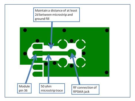
PCB Layer 2 of RF layout example
