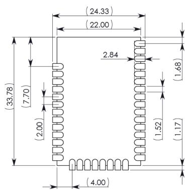
The solder footprint should be matched to the copper pads, but may need to be adjusted depending on the specific needs of assembly and product standards.
