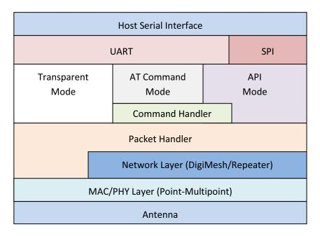
The command handler is the code that processes commands from AT Command Mode or API Mode; see AT commands on page 99. The command handler can also process commands from remote radios; see Remote AT commands on page 100.
