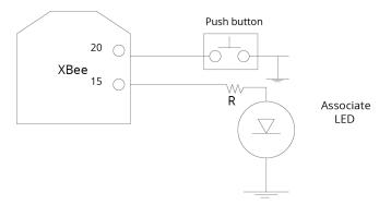
A pushbutton and an LED can be connected to module pins 20 and 15 respectively to support the commissioning pushbutton and associated LED functionalities
