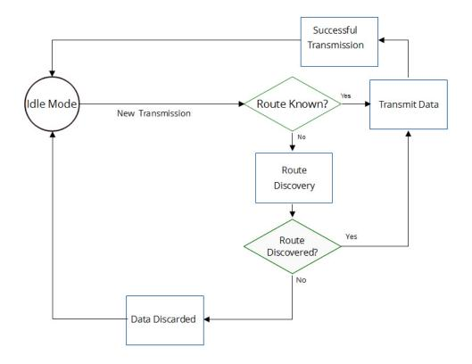
When DigiMesh data is transmitted from one node to another, a network-level acknowledgment is transmitted back across the established route to the source node. This acknowledgment packet indicates to the source node that the data packet was received by the destination node. If a network acknowledgment is not received, the source node will re-transmit the data.
