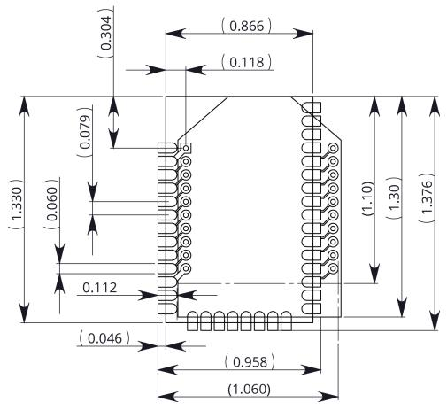
The round holes in the diagram are for the XBee through-hole design, and the semi-oval pads are for the XBee SMT design. Pin 1 of the through-hole design is lined up with pin 1 of the SMT design, but the pins are actually offset by one pad (see Pin Mapping above). By using diagonal traces to connect the appropriate pins, the layout will work for both modules.
