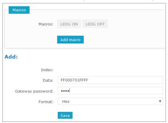
• Using the macros or by modification of commands in *IQRF Tx* field and the *Send* button you can control LEDs in individual or all nodes similarly as before (by using IQRF IDE).
