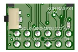
Caution: The KON-RASP-01 shield can be connected to Raspberry PI board while the board is powered off only.
