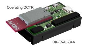
USB connector is intended just for accumulator charging but not for USB connectivity.
