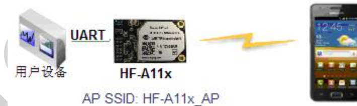
Figure 34. Wireless Control Application
