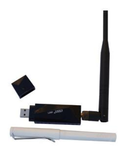
AR9271 chipset uses free software drivers and firmware. Both the driver and the firmware of this adapter are free under the GNU GPL v2 and the 3-clause BSD licenses, respectively, and thus you can use it with a completely free GNU/Linux distribution, which has the kernel Linux-libre, clean of the nonfree
