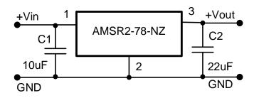
C1: A low ESR capacitor is required to keep the noise of the converter to a minimum. Ceramic capacitors are recommended with typical value is  $10\mu$ F / 25V.
