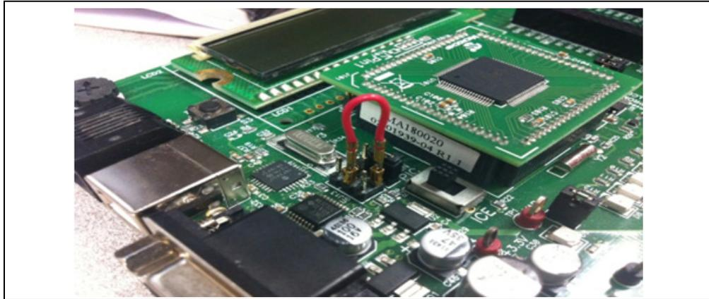
2. Use the MPLAB X IDE and the available programmer to load the `SampleTelnetApp.hex` file demo application into the PIC18F87J11.
