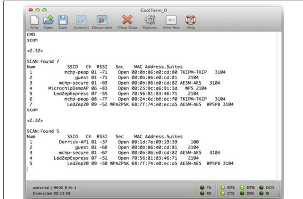
5. Store the NETWORK\_SSID and NETWORK\_PASS parameters from step 3 if required into the RN131/171 module's non-volatile memory to enable the use of these parameters in the next application to run on the PIC18F87J11.
