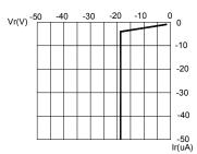
FIG.3 REVERSE CURRENT VS. REVERSE VOLTAGE.
