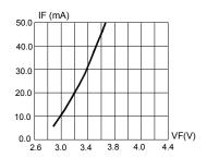
FIG.1 FORWARD CURRENT VS. FORWARD VOLTAGE.
