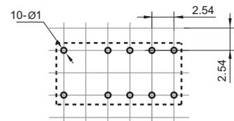
**OUTLINE DIMENSIONS, WIRING DIAGRAM AND PC BOARD LAYOUT**
