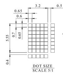
The non-specified tolerance of dimension is  $\pm 0.3$  mm.
