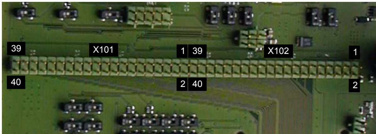
Figure 5: Overview of B2B connector pins and the corresponding test points
