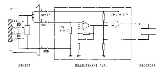
imes MEASUREMENT AMP.: NON-INVERTED TYPE, GAIN 72.5 dB AT 1 Hz 0.4 $\sim$ 2.7 Hz/-3 dB
