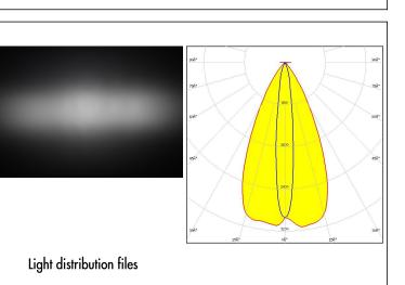
LED XP-G2 FWHM / FWTM 52.0 + 12.0° / 78.0 + 33.0° Efficiency 91 % Peak intensity 3.3 cd/lm LEDs/each optic 1 Light colour/type White Required components: Light distribution files
