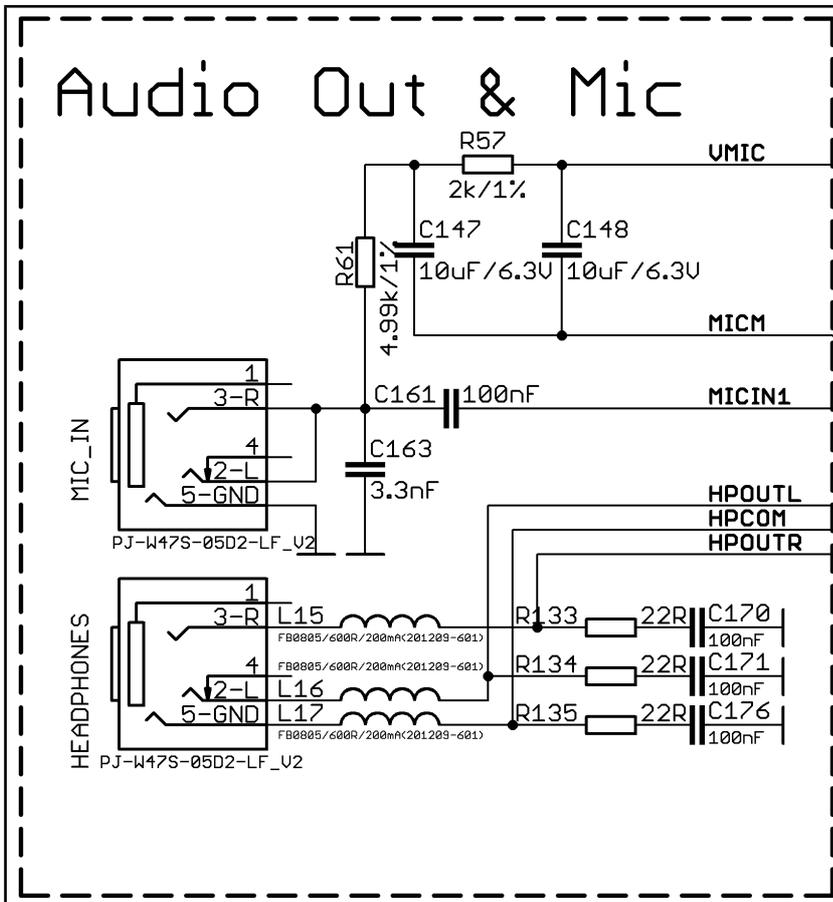
Standard MIC\_IN jack is mounted for audio input to the board. Note that it is a single channel
