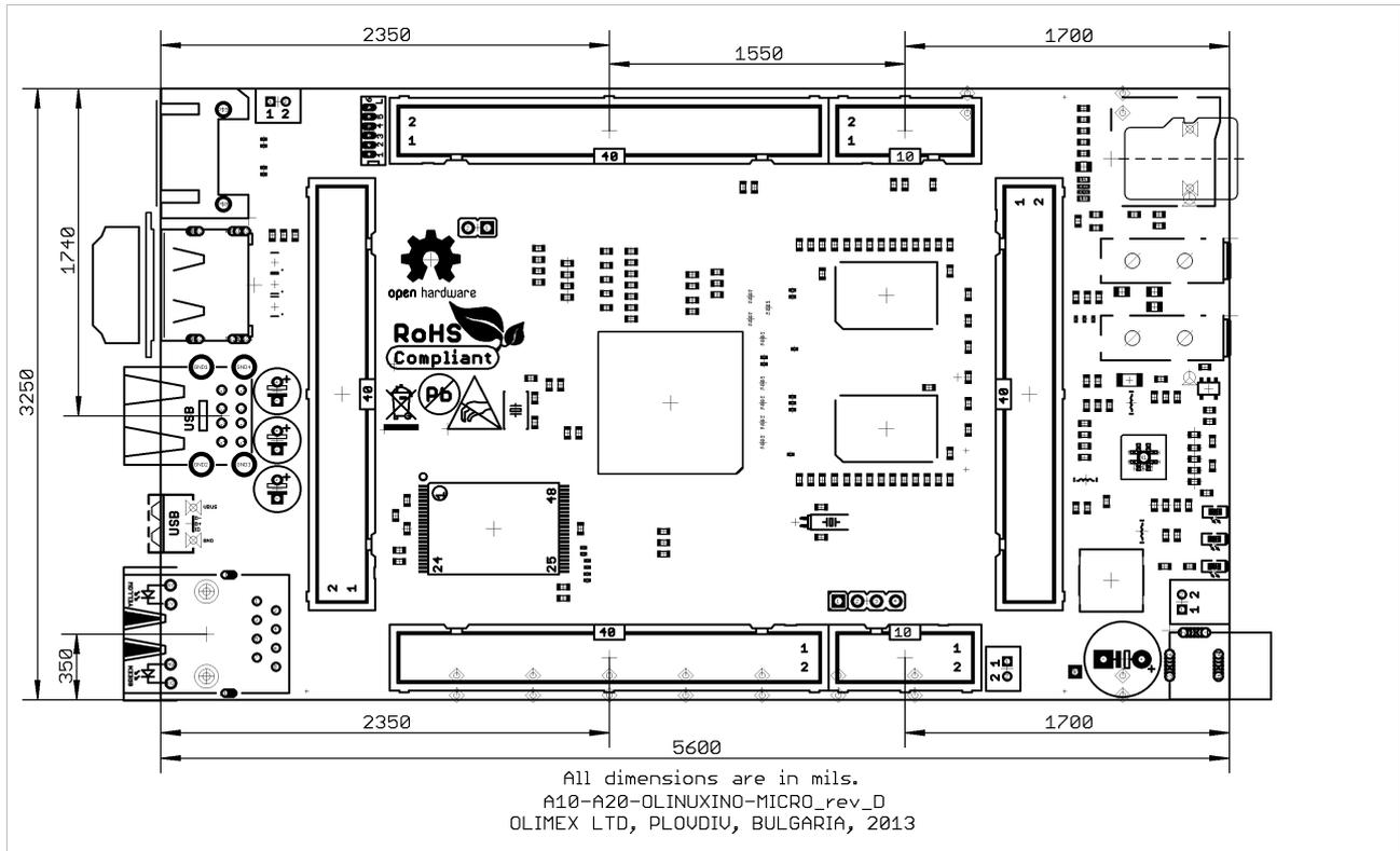
The three highest elements on the board in order from the tallest to the shortest are: USB\_HOST connector – 700mils, capacitors C202 – 650mils, the Ethernet connector – 600mils.
