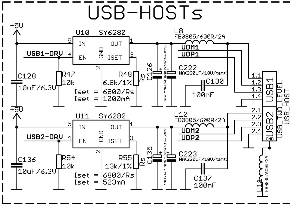
The USB\_HOST connector features two levels – called USB1 and USB2 in the schematic. The connector is situated between the USB\_OTG and the HDMI connector. Each of slots them features a low loss power distribution switch SY6280 which protects the board in case the devices you have plugged to each level USB\_HOST try to draw more than the allowed current.
