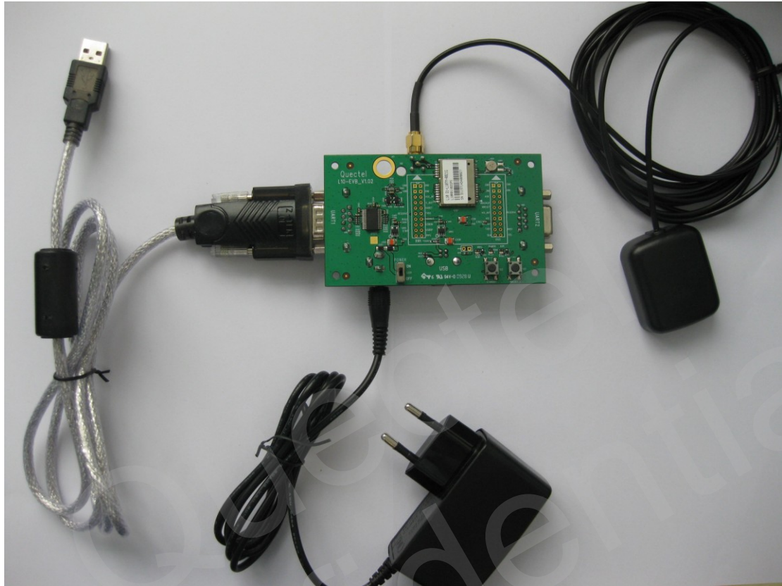
Figure 12: EVB and accessory equipments with serial cable
