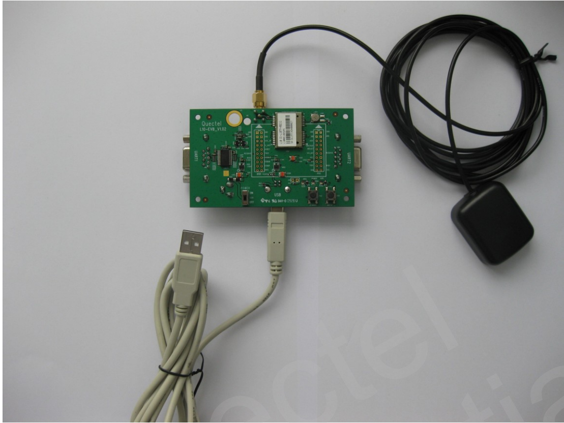
Figure 13: EVB and accessory equipments with USB cable
