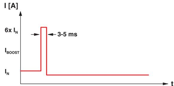
Tripping time of the circuit breaker = 3 - 5 ms, typically
