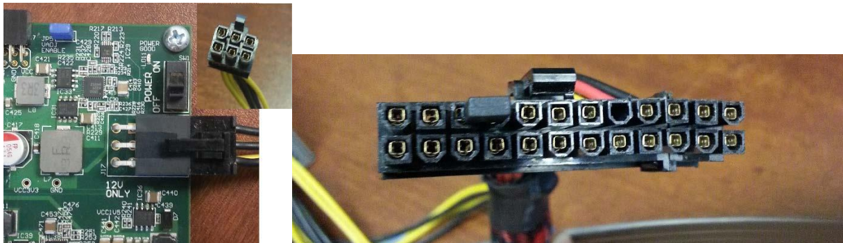
Figure1. Left: NetFPGA-1G can be powered by plugging the 6-pin PCIe power connector in J17; Right: Pin 16 and 17 are shorted using a jumper to power on a standard ATX power supply when used standalone.
