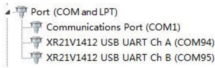
Figure 5: UART Ports Displayed on PC
