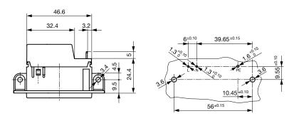
1) with cover 2) without cover For grounding additional quick connect terminal 4.8 x 0.8 mm
