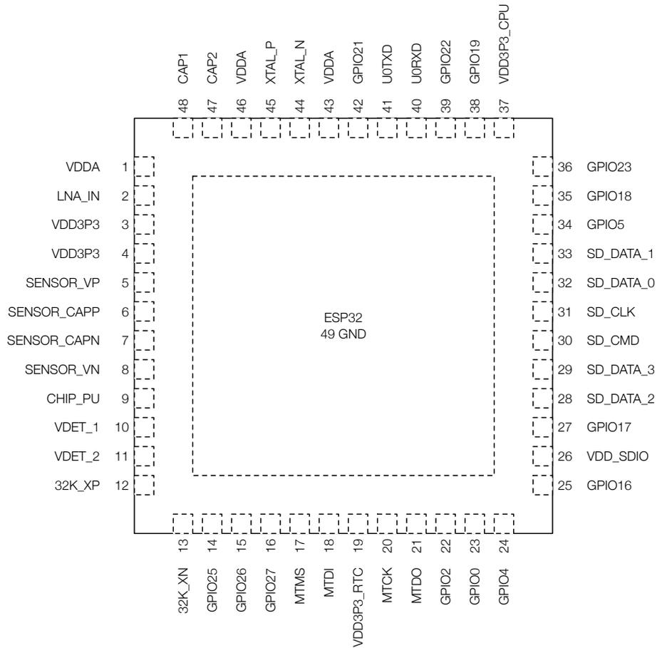
Figure 2: ESP32 Pin Layout (QFN 6\*6, Top View)
