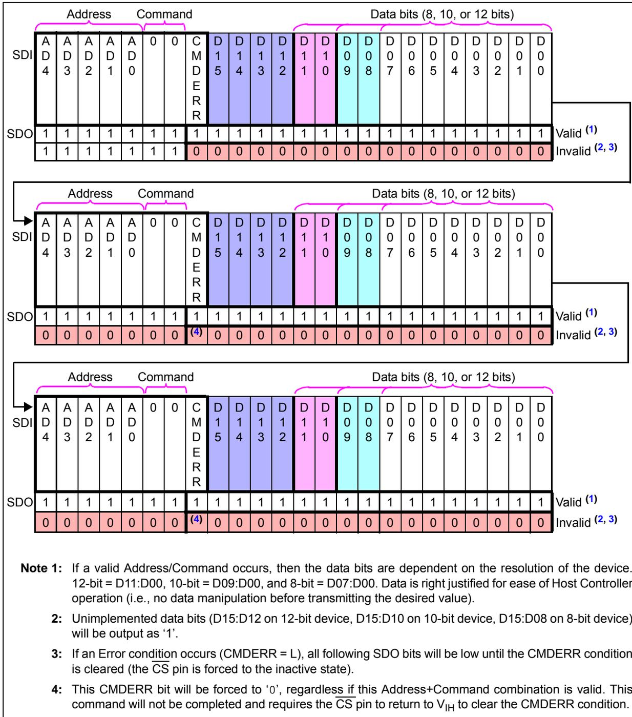
**FIGURE 7-4:** Continuous Write Sequence (Volatile Memory only).
