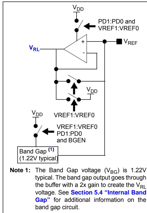
**Note 1:** The Band Gap voltage ( $V_{BG}$ ) is 1.22V typical. The band gap output goes through the buffer with a 2x gain to create the  $V_{RL}$  voltage. See Section 5.4 "Internal Band Gap" for additional information on the band gap circuit.
