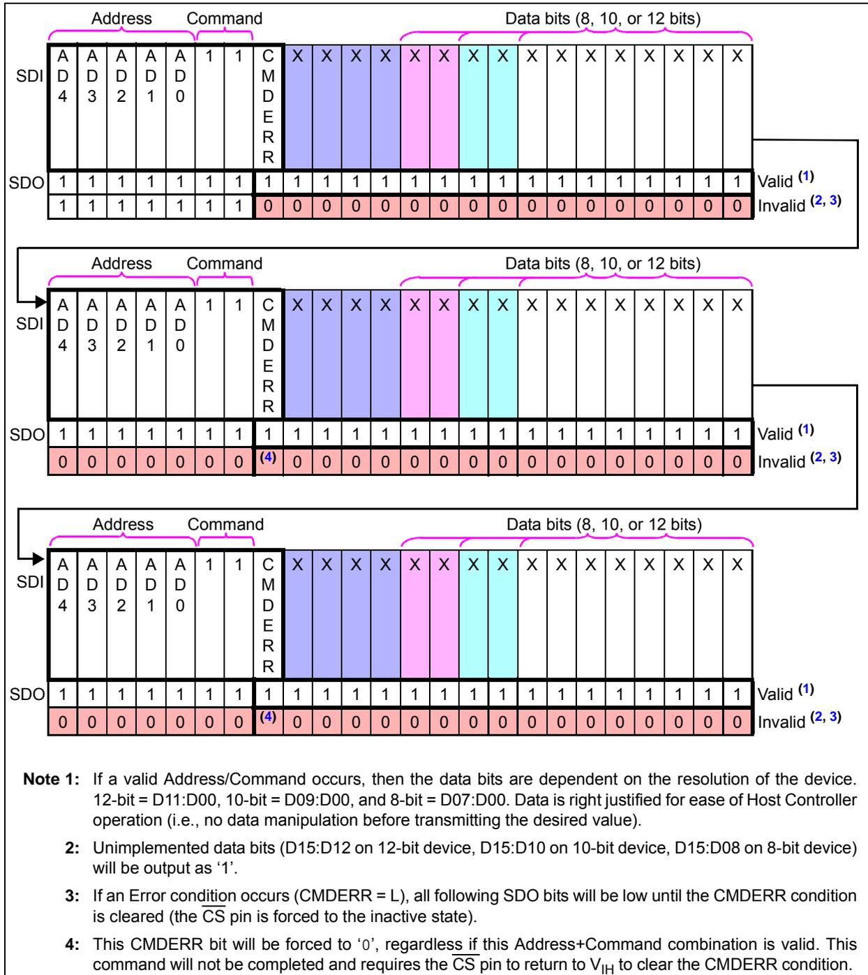
**FIGURE 7-8:** Continuous-Reads Sequence.
