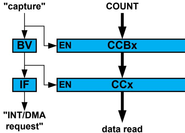
For input capture, the buffer register and the corresponding CCx act like a FIFO. When CCx is empty or read, any content in CCBUFx is transferred to CCx. The buffer valid flag is passed to set the CCx interrupt flag (IF) and generate the optional interrupt, event or DMA request. The CCBUFx register value can't be read, all captured data must be read from the CCx register.
