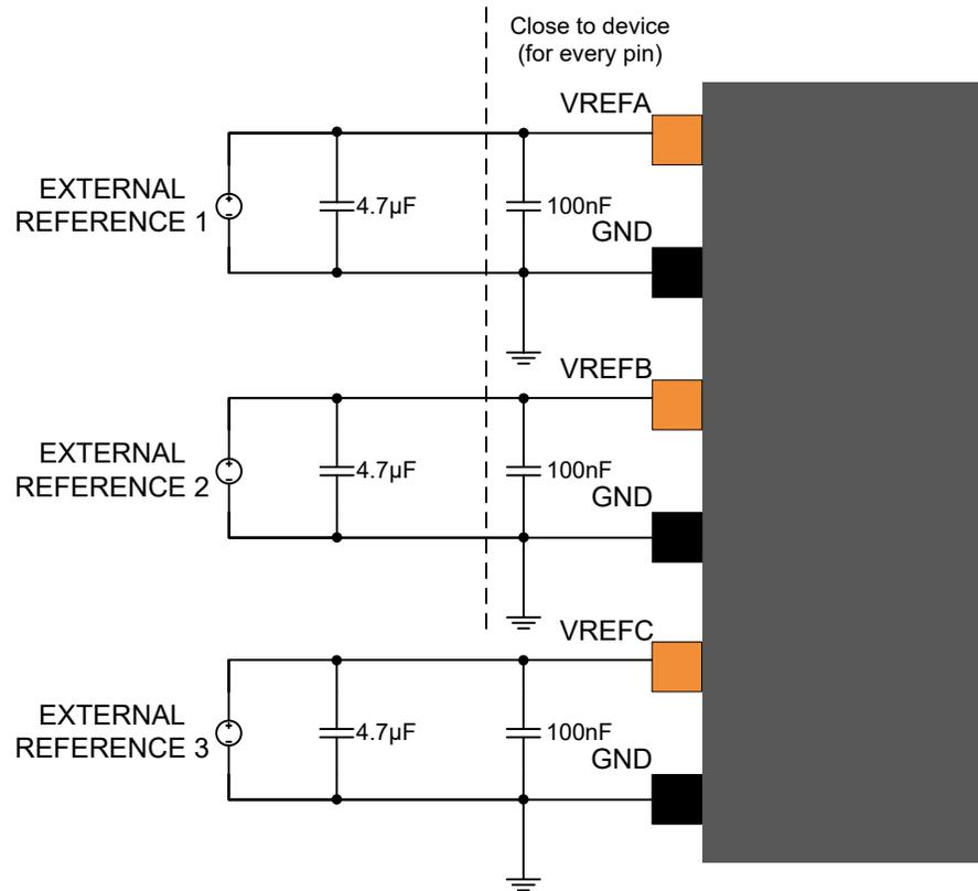
Figure 60-5. External Analog Reference Schematic With Two References
