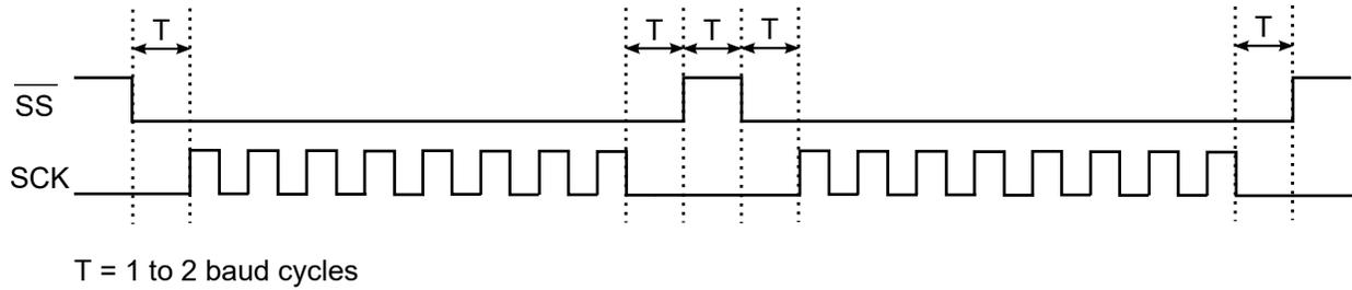
When CTRLB.MSSEN=0, the  $\overline{SS}$  pin(s) is/are controlled by user software and normal GPIO.
