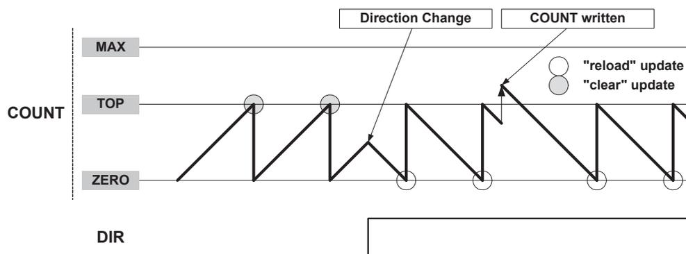
Users can change the counter value (by writing directly in the COUNT register) even when the counter is running. The COUNT value will always be ZERO or TOP, depending on direction set by CTRLBSET.DIR or CTRLBCLR.DIR, when starting the TCC, unless a different value has been written to it, or the TCC has been stopped at a value other than ZERO. The write access has higher priority than count, clear, or reload. The direction of the counter can also be changed during normal operation.
