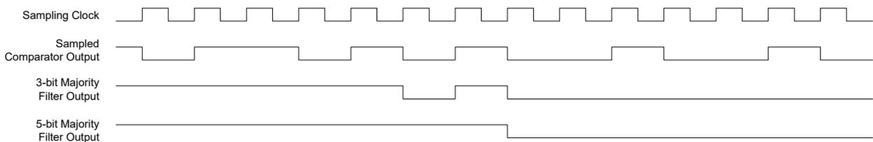
**Figure 46-7. Single-Shot Filtering**
