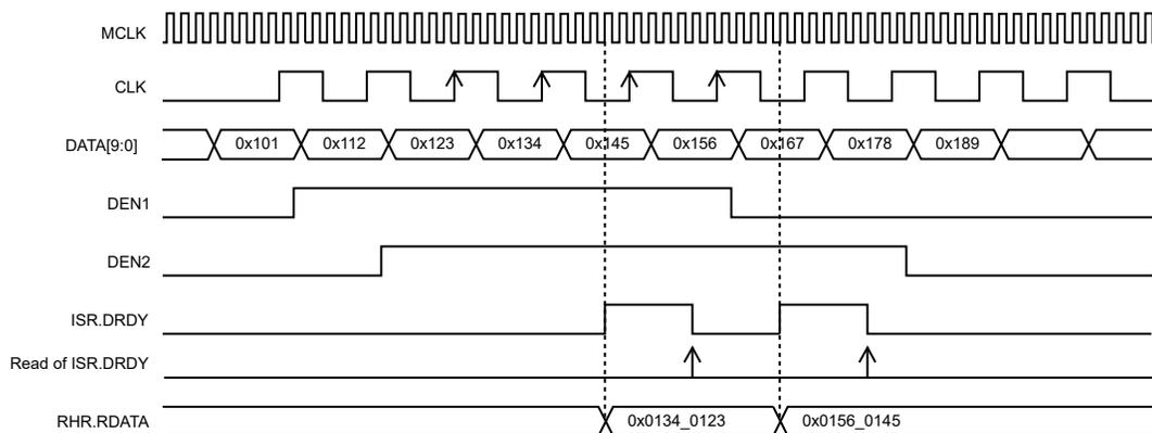
**Figure 52-5.** PCC Waveforms (ISIZE=10\_BITS, DSIZE=2\_DATA, ALWAYS = 0, HALFS = 0, SCALE = 1)
