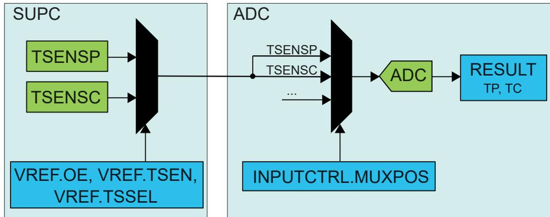
The state of the MUX input selection bit fields in the ADC Input Control register (ADC.INPUTCTRL.MUXPOS and MUXNEG) does not affect the sensor selection.
