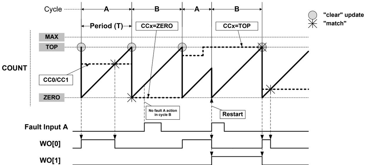
**Capture Action** Several capture actions can be selected by writing the Fault n Capture Action bits in the Fault n Control register (FCTRLn.CAPTURE). When one of the capture operations is selected, the counter value is captured when the fault occurs. These capture operations are available:
