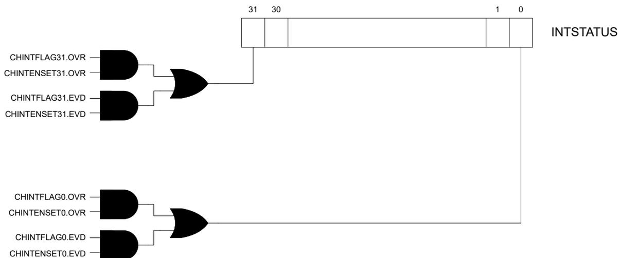
The Event System can arbitrate between all channels with pending interrupts. The arbiter can be configured to prioritize statically or dynamically the incoming events. The priority is evaluated each time a new channel has an interrupt pending, or an interrupt has been cleared. The Channel
