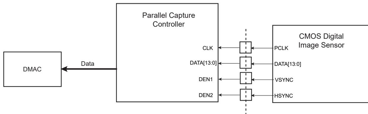
The PCC must be configured first, and is enabled by writing a '1' to the Parallel Capture Enable bit in the Mode Register (MR.PCEN).
