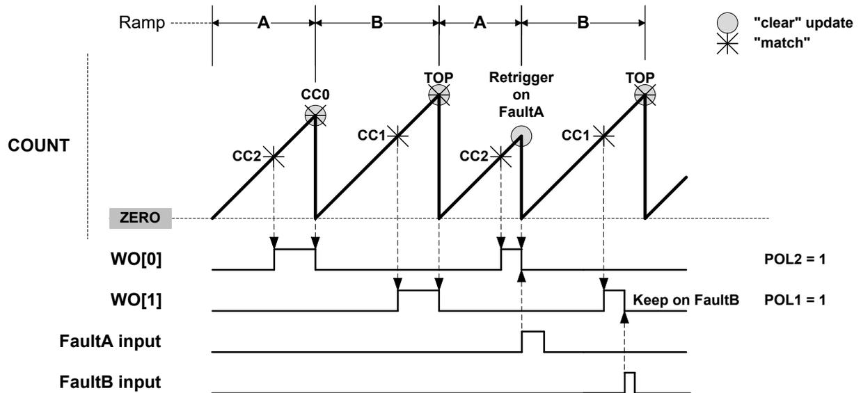
Figure 49-21. RAMP2 Critical Operation With 2 Channels
