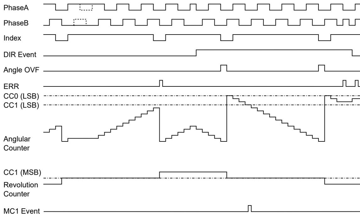
in Q4 and Q4S configuration, a valid index is detected when the three inputs (PhaseA, PhaseB and Index) are at low level.
