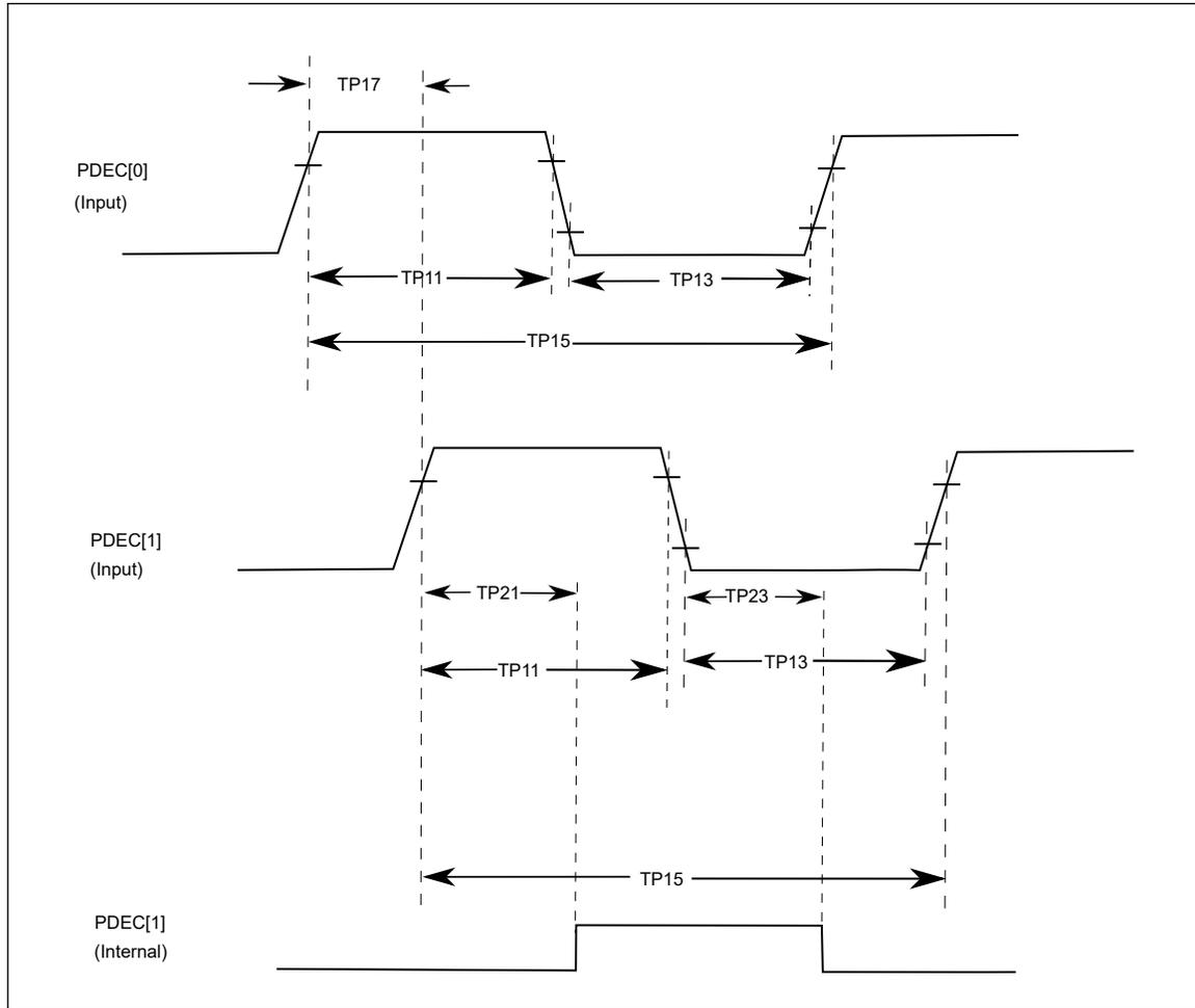
Table 54-67. Quadrature Encoder Interface Electrical Specifications <sup>(1)</sup>
