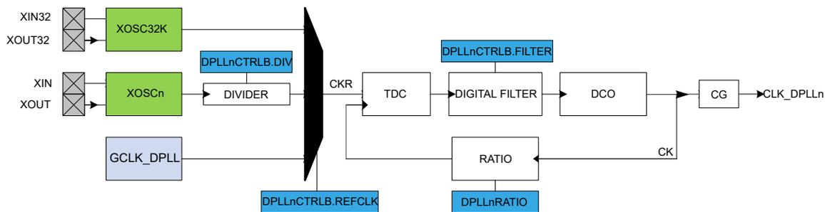
When the controller is disabled, the output clock is low. If the Loop Divider Ratio Fractional part bit field in the DPLL Ratio register (DPLLnRATIO.LDRFRAC) is zero, the DPLL works in Integer mode. Otherwise, the fractional mode is activated. The fractional part has a negative impact on the jitter of the DPLL.
