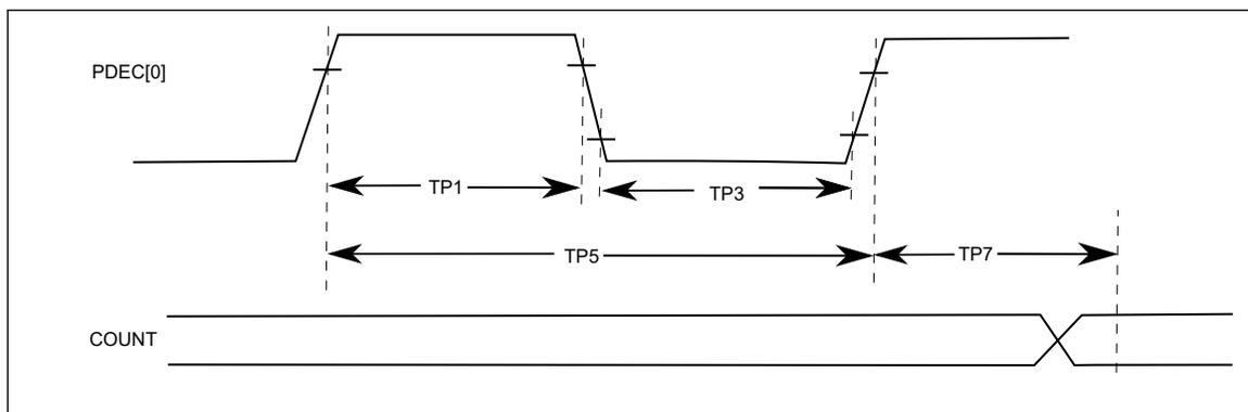
Figure 54-30. PDEC[0]/PDEC[1] Input Characteristics
