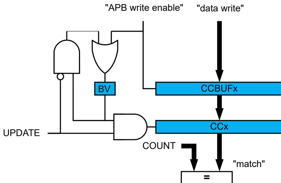
Both the registers (PATT/PER/CCx) and corresponding Buffer registers (PATTBUFPERBUF/CCBUFx) are available in the I/O register map, and the double buffering feature is not mandatory. The double buffering is disabled by writing a '1' to CTRLSET.LUPD.
