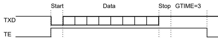
The Transmit Complete interrupt flag (INTFLAG.TXC) will be raised after the guard time is complete and TE goes low.
