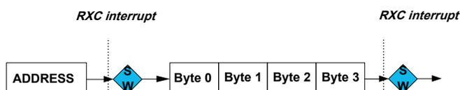
When utilizing the length counter, the LENGTH register must be written before the frame begins. If the frame length while  $\overline{SS}$  is low is not a multiple of LENGTH.LEN Bytes, the Length Error Status bit (STATUS.LENERR) is raised. If LENGTH.LEN is not a multiple of 4 Bytes, the final INTFLAG.RXC interrupt will be raised when the last Byte is received.
