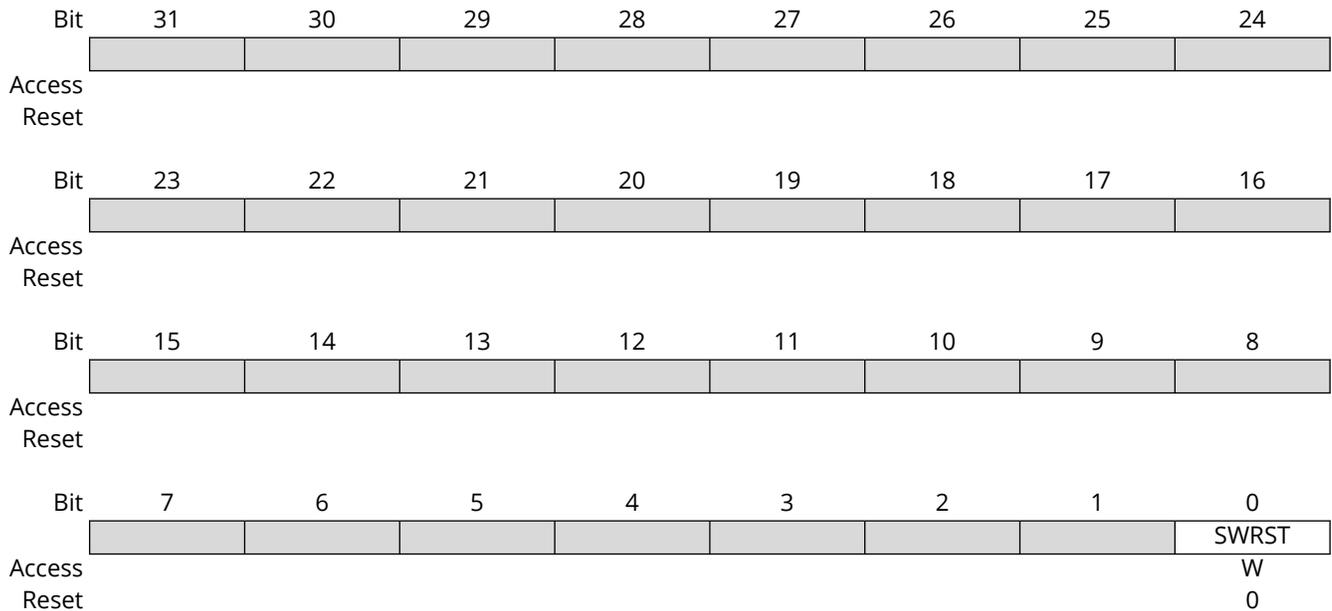
**Bit 0 - SWRST** Cache Controller Software Reset
