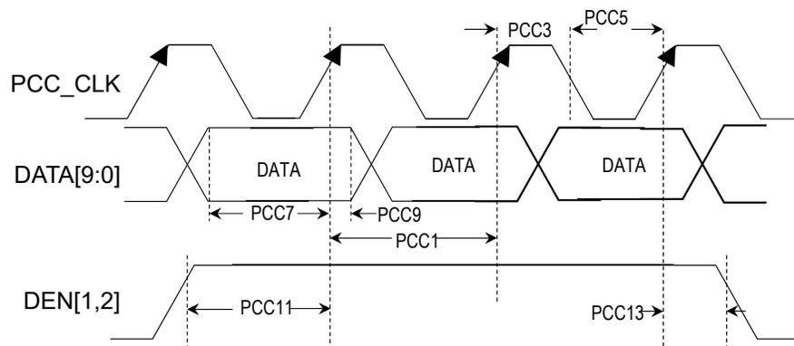
**Table 54-64.** PCC - Peripheral Capture Controller Electrical Specifications <sup>(4)</sup>
