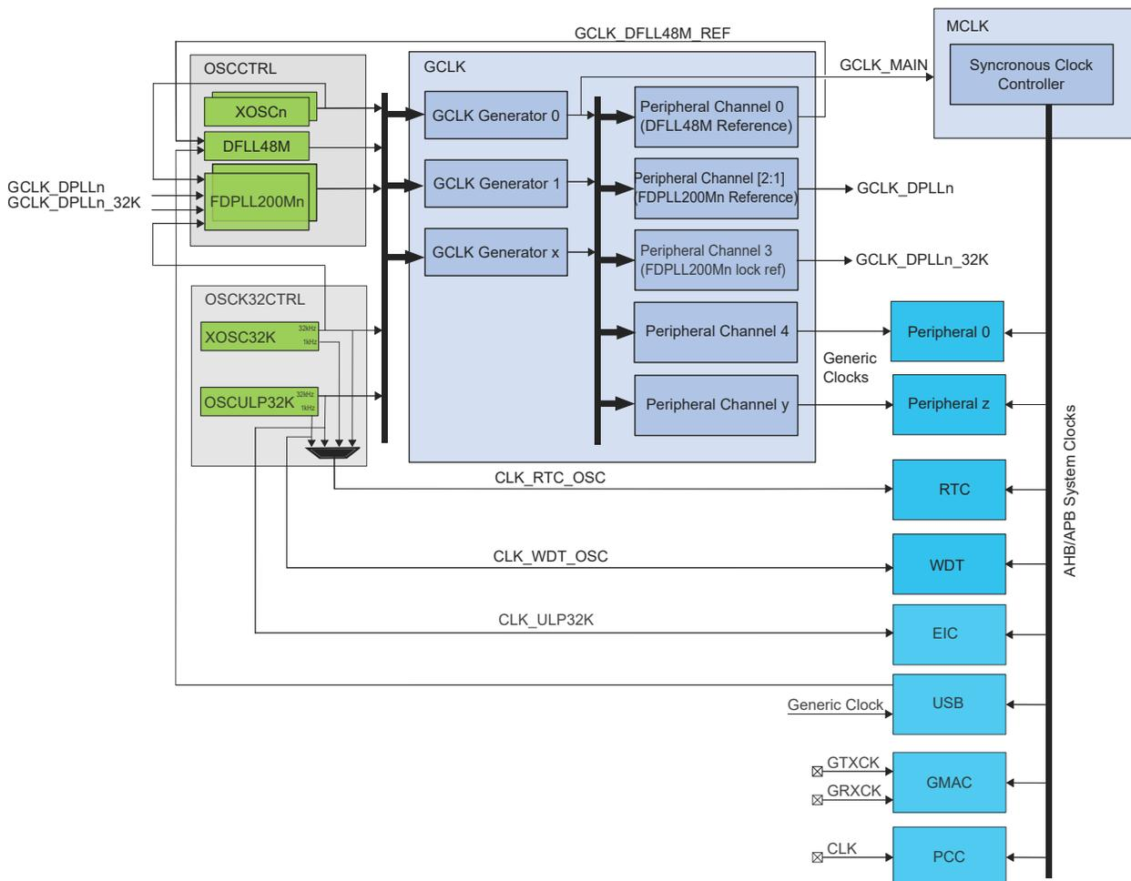
The SAM D5x/E5x clock system consists of:
