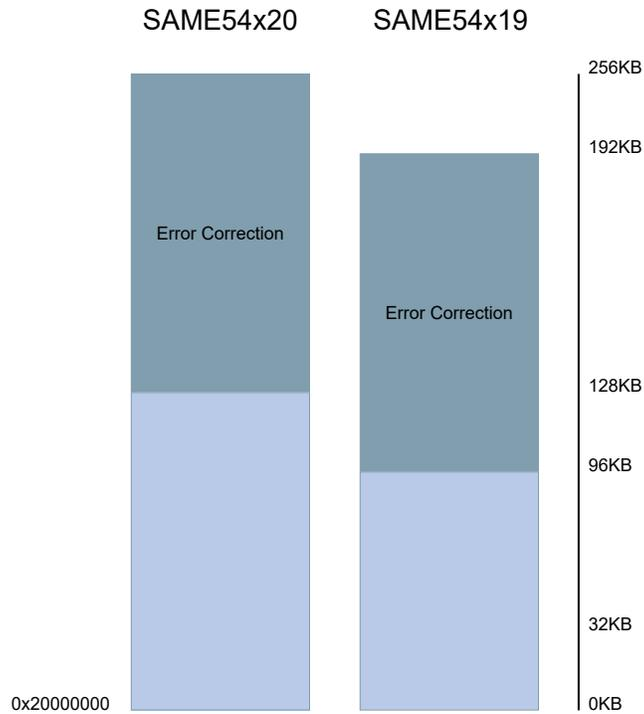
**Note:** If the ECC is used, full SRAM retention must be enabled.
