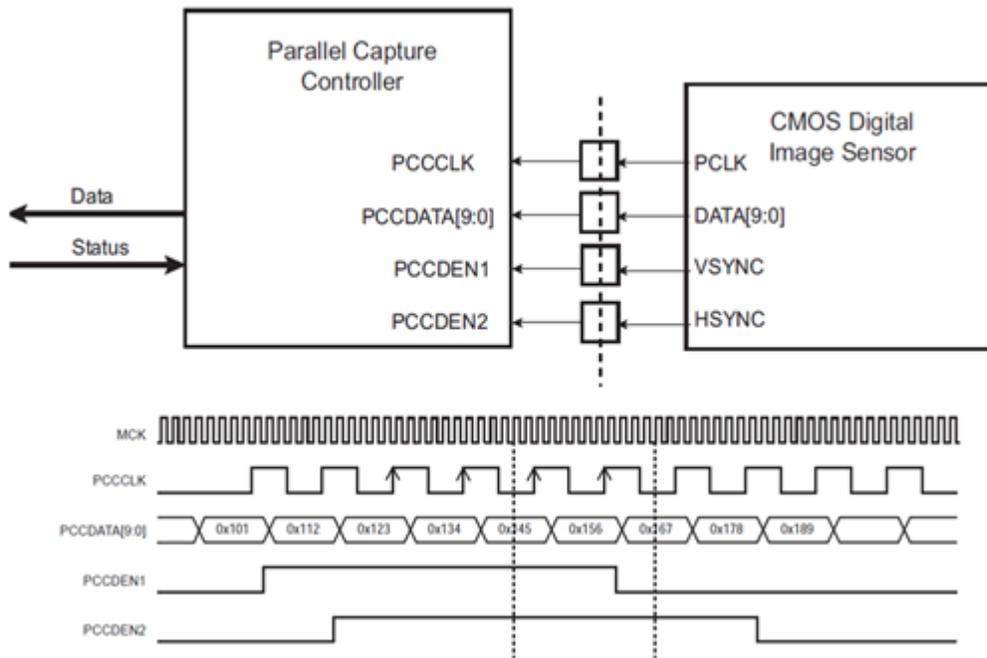
Figure 54-23. PCC - Peripheral Capture Controller Timing Diagrams
