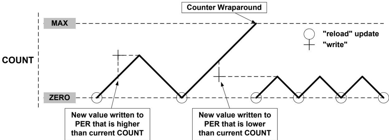
When double buffering is used, the buffer can be written at any time and the counter will still maintain correct operation. The period register is always updated on the update condition, as shown in Figure 49-13. This prevents wraparound and the generation of odd waveforms.
