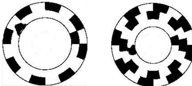
**Type 3 Error: Missing Angular Step Detection**
