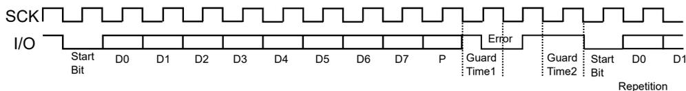
When the USART is the receiver and it detects a parity error, the parity error bit in the Status Register (STATUS.PERR) is set and the character is not written to the receive FIFO.
