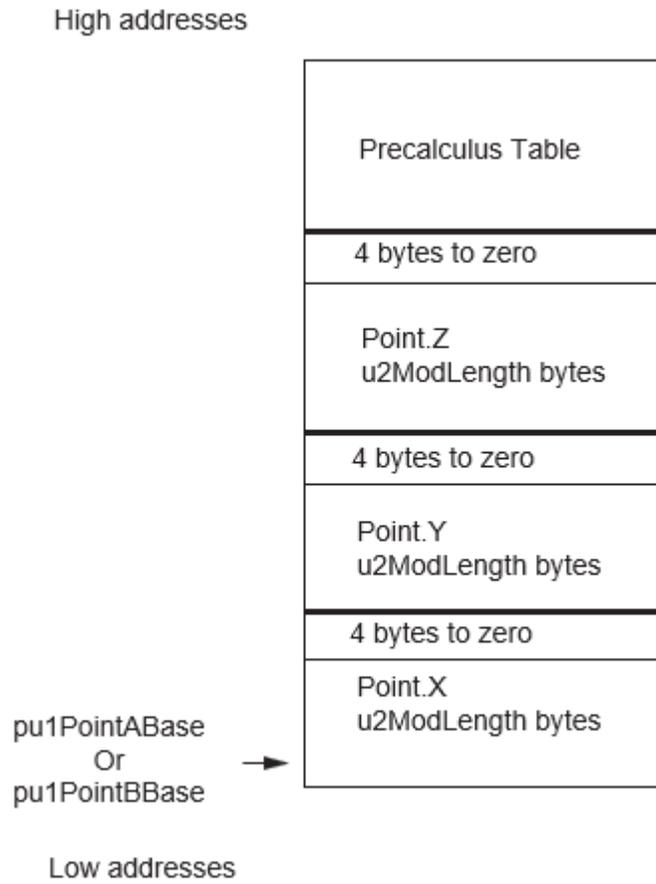
**Figure 43-9.** Scalars KA and KB {pu1KABBase, 2 \* u2KLength + 8}
