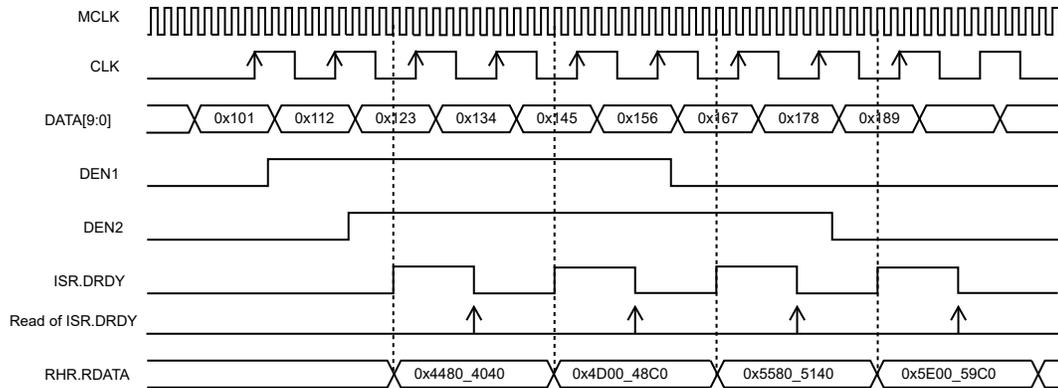
**Figure 52-9.** PCC Waveforms (DSIZE=4\_DATA, ALWAYS = 0, HALFS = 1, FRSTS = 0)
