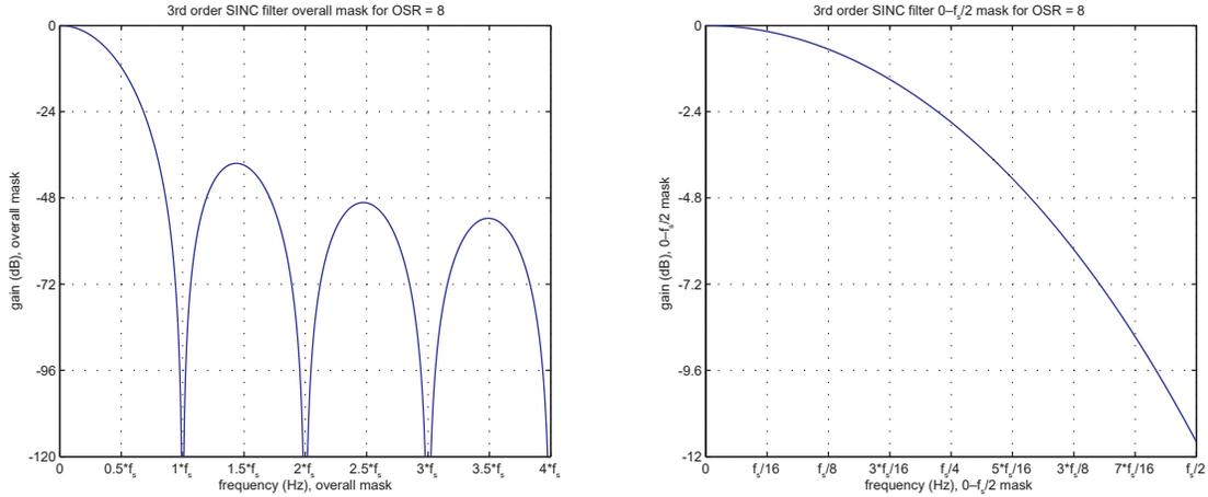
Figure 47-9. Interpolator Spectral Mask for 16x OSR
