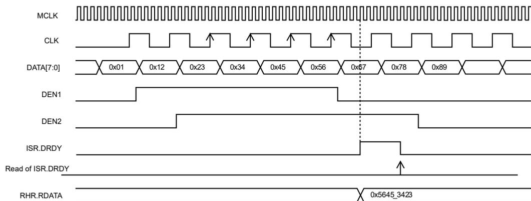
**Figure 52-4.** PCC Waveforms (ISIZE=10\_BITS, DSIZE=2\_DATA, ALWYS = 0, HALFS = 0, SCALE = 0)
