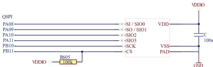
**Note:** Signal integrity can be improved by adding series resistors on each QSPI line. The resistor value should be based on the corresponding I/O pin drive strength (decided by PINCFGn.DRVSTR) and PCB trace impedance. It is recommended to do simulation using the device IBIS files to choose the correct termination and PCB trace impedance combination.
