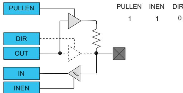
**Note:** When pull is enabled, the pull value is defined by the OUT value.
