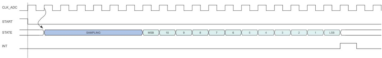
The ADC provides also offset compensation, see the following figure. The offset compensation is enabled by the Offset Compensation bit in the Sampling Control register (SAMPCTRL.OFFCOMP).
