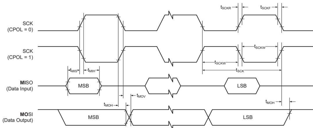
Figure 54-9. SPI Timing Requirements in Client Mode
