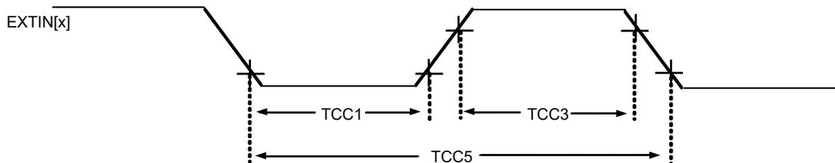
**Figure 54-27. TCCx Timer Compare Output Module Timing Diagrams**
