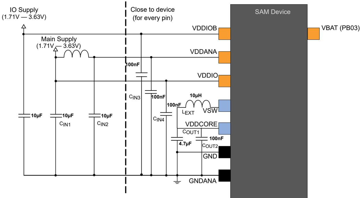
Figure 60-2. Power Supply Connection for Linear Mode Only
