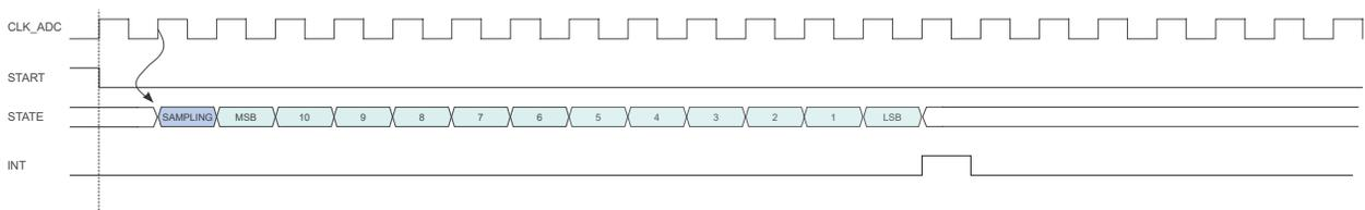
The sampling time can be increased by using the Sampling Time Length bit group in the Sampling Time Control register (SAMPCTRL.SAMPLEN). As example, the next figure is showing the timing conversion with sampling time increased to six CLK\_ADC cycles.
