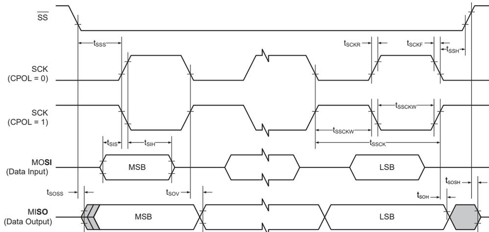
Table 54-56. SPI Timing Characteristics and Requirements<sup>(1)</sup>
