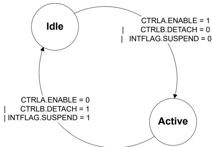
In Idle state, the pad is in Low Power Consumption mode.
