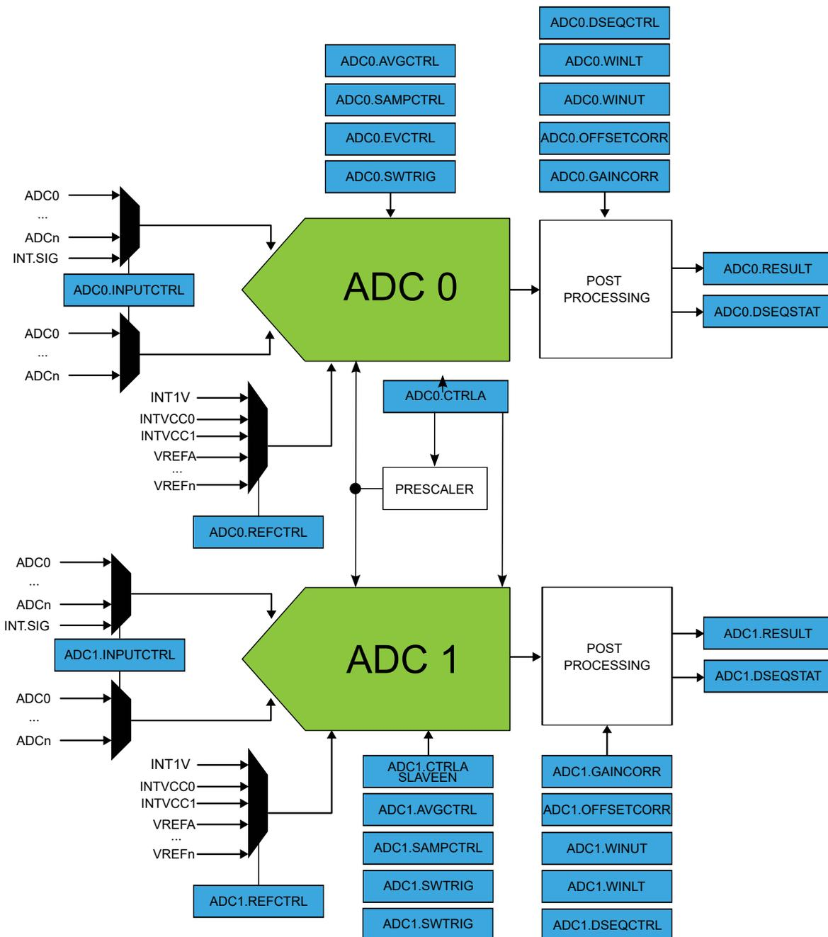
In this mode of operation, the Client ADC1 is enabled by accessing the CTRLA register of the Host ADC0. In the same way, the Host ADC event inputs will be automatically routed to the Client ADC, meaning that the input events configuration must be done in the Host ADC (ADC0.EVCTRL).
