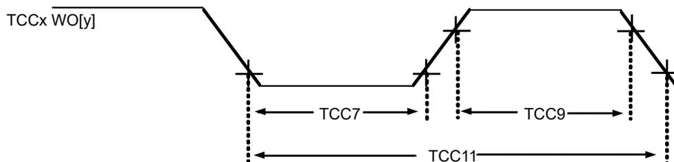
Figure 54-28. TCCx Timer Compare Fault Output Module Timing Diagrams
