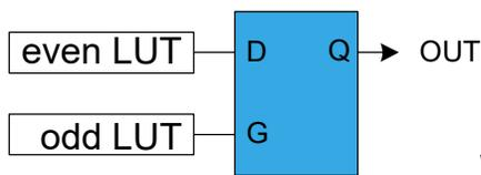
When the even LUT is disabled (LUTCTRL0.ENABLE=0 / LUTCTRL2.ENABLE=0), the latch output will be cleared. The G-input is forced enabled for one more APB clock cycle, and the D-input to zero. In all other cases, the latch output (OUT) is refreshed as shown in Table 41-4.
