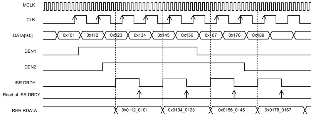
**Figure 52-8.** PCC Waveforms (ISIZE=10\_BITS, DSIZE=2\_DATA, ALWAYS = 1, HALFS = 0, SCALE = 1)
