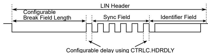
After header transmission is complete, the Client responds with 1-8 data bytes plus checksum.
