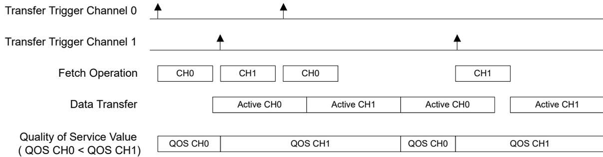
When a channel is stored in the Pre-Fetch or Active Channel, the corresponding PRICTRLx.QOS bits value is stored in the respective channel. As shown in Quality of Service, the DMAC will select the highest QOS value between Active and Pre-Fetch channels. This value will apply to all DMAC buses.
