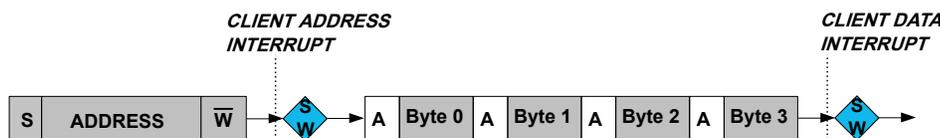
The LENGTH register can be written before the frame begins, or when the AMATCH interrupt is set. If the frame size is not LENGTH.LEN Bytes, the Length Error status bit (STATUS.LENERR) is raised. If LENGTH.LEN is not a multiple of 4 Bytes, the final INTFLAG.DRDY interrupt is raised when the last Byte is received for Host reads. For Host writes, the last data byte will be automatically NACKed. On address recognition, the internal length counter is reset in preparation for the incoming frame.
