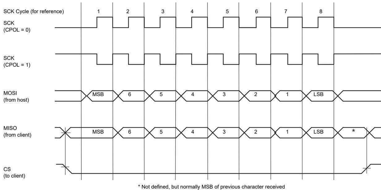
**Figure 37-4.** QSPI Transfer Modes (BAUD.CPHA = 1, 8-bit transfer)
