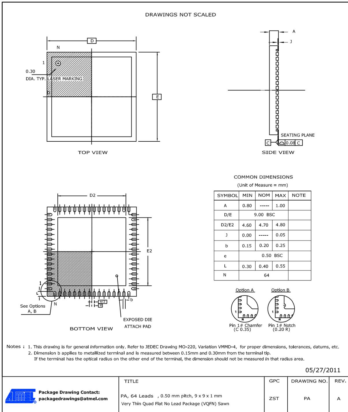
**Note:** The exposed die attach pad is not connected electrically inside the device. It is recommended that the exposed pad be connected to ground in the PCB.
