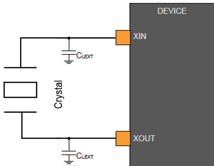
The user must choose a crystal oscillator where the crystal load capacitance  $C_L$  is within the range given in the Table. The exact value of  $C_L$  can be found in the crystal data sheet. The capacitance of the external capacitors ( $C_{LEXT}$ ) can then be computed as follows:
