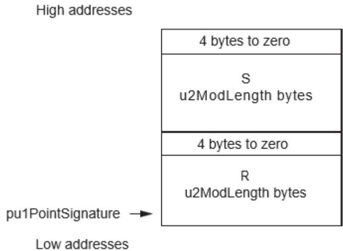
**Figure 43-14.** The a parameter and Workspace {pu1AWorkBase, 9\*u2ModLength + 48}
