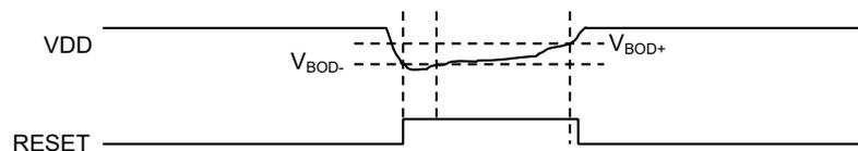
**Table 56-6.** BOD33 Characteristics on V<sub>DD</sub> and V<sub>BAT</sub> Monitoring in Normal Mode (During Power-up Phase and Active Mode)
