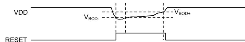
Enabling the BOD33 hysteresis by writing the Hysteresis bit field in the BOD33 register (BOD33.HYST) to a non-null value will add hysteresis to the BOD33 threshold level.
