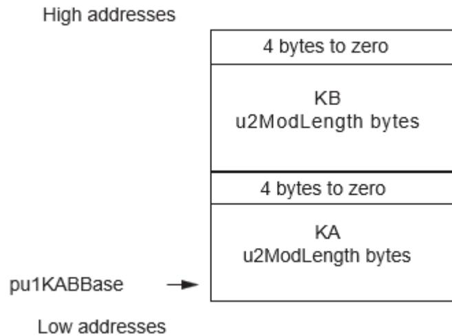
Figure 43-10. The a parameter and Workspace {pu1AWorkBase, 9\*u2ModLength + 48}
