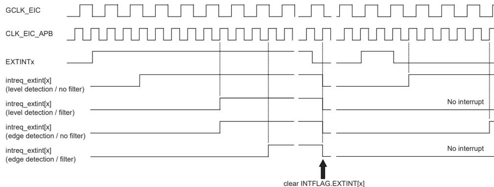
Detection latency depends on the detection mode.
