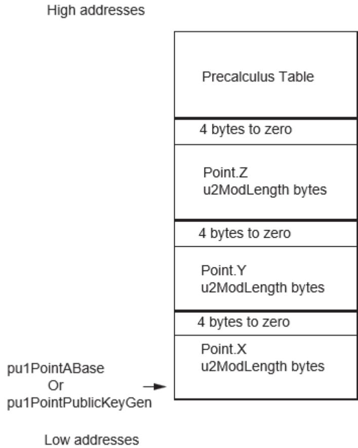
**Figure 43-13.** PointSignature {pu1PointSignature, 2 \* u2ScalarLength + 8}
