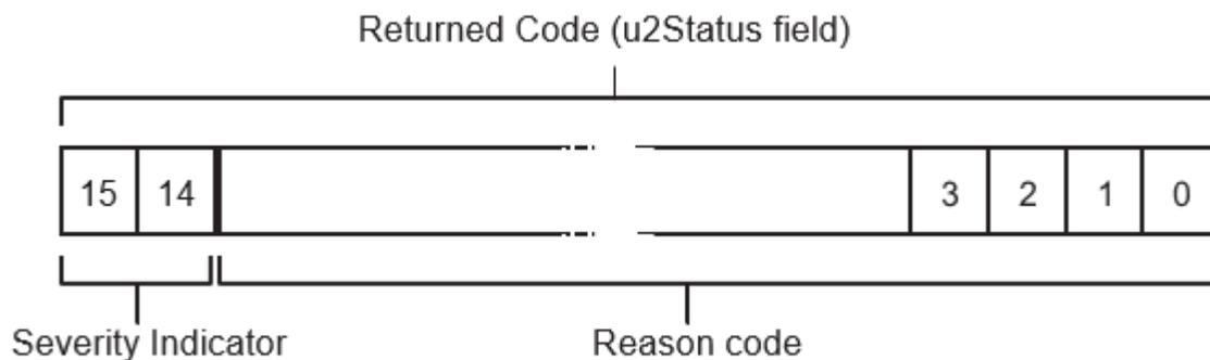
The following table shows how the severity indicators should be decoded.
