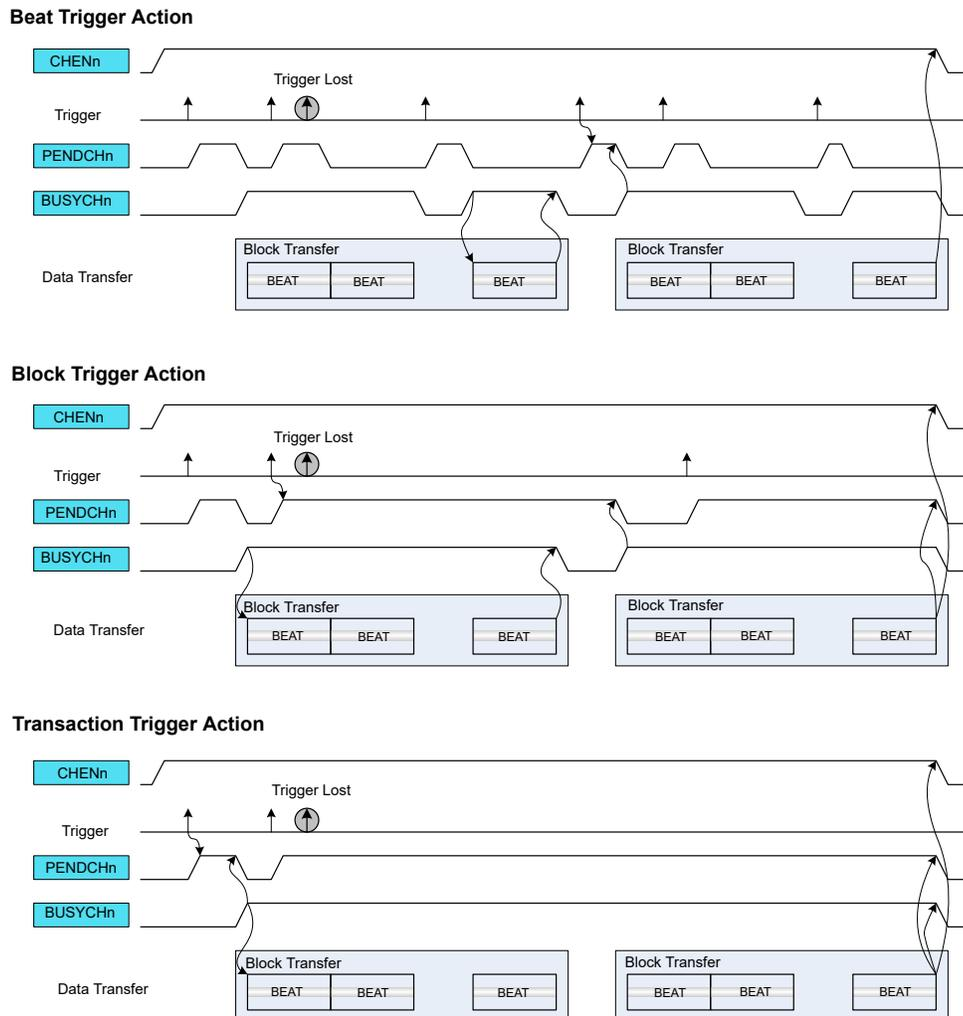
If the trigger source generates a transfer request for a channel during an ongoing transfer, the new transfer request will be kept pending (CHSTATUSn.PEND=1), and the new transfer can start after the ongoing one is done. Only one pending transfer can be kept per channel. If the trigger source
