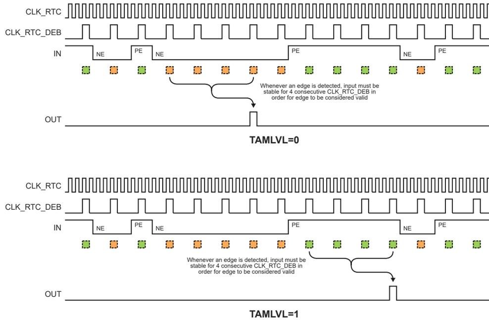
Figure 21-7. Edge Detection with Asynchronous Stability Debouncing
