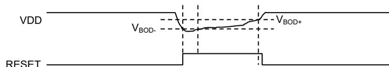
**Table 55-4.** BOD33 Characteristics on VDD and VBAT Monitoring in Normal Mode (During Power-up Phase and Active Mode)
