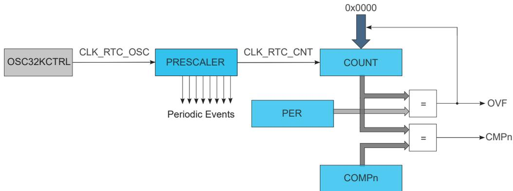
Figure 21-3. RTC Block Diagram (Mode 2 — Clock/Calendar)
