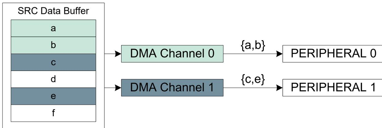
Incrementation for the destination address of a block transfer is enabled by setting the Destination Address Incrementation Enable bit in the Block Transfer Control register ( $BTCTRL.DSTINC = 1$ ). The step size of the incrementation is configurable by clearing  $BTCTRL.STEPSEL = 0$  and writing  $BTCTRL.STEPSIZE$  to the desired step size. If  $BTCTRL.STEPSEL = 1$ , the step size for the destination incrementation will be the size of one beat.
