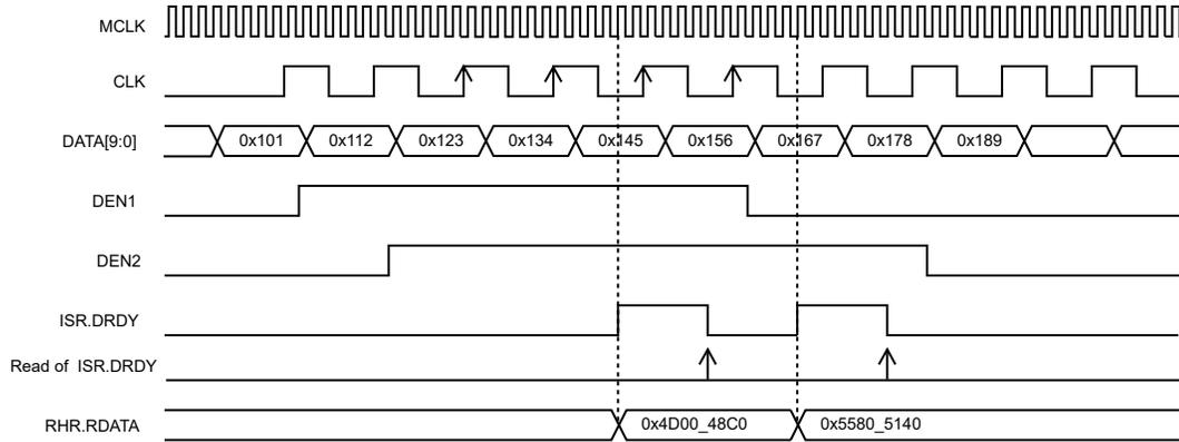
**Figure 52-6.** PCC Waveforms (DSIZE=4\_DATA, ALWAYS = 1, HALFS = 0)
