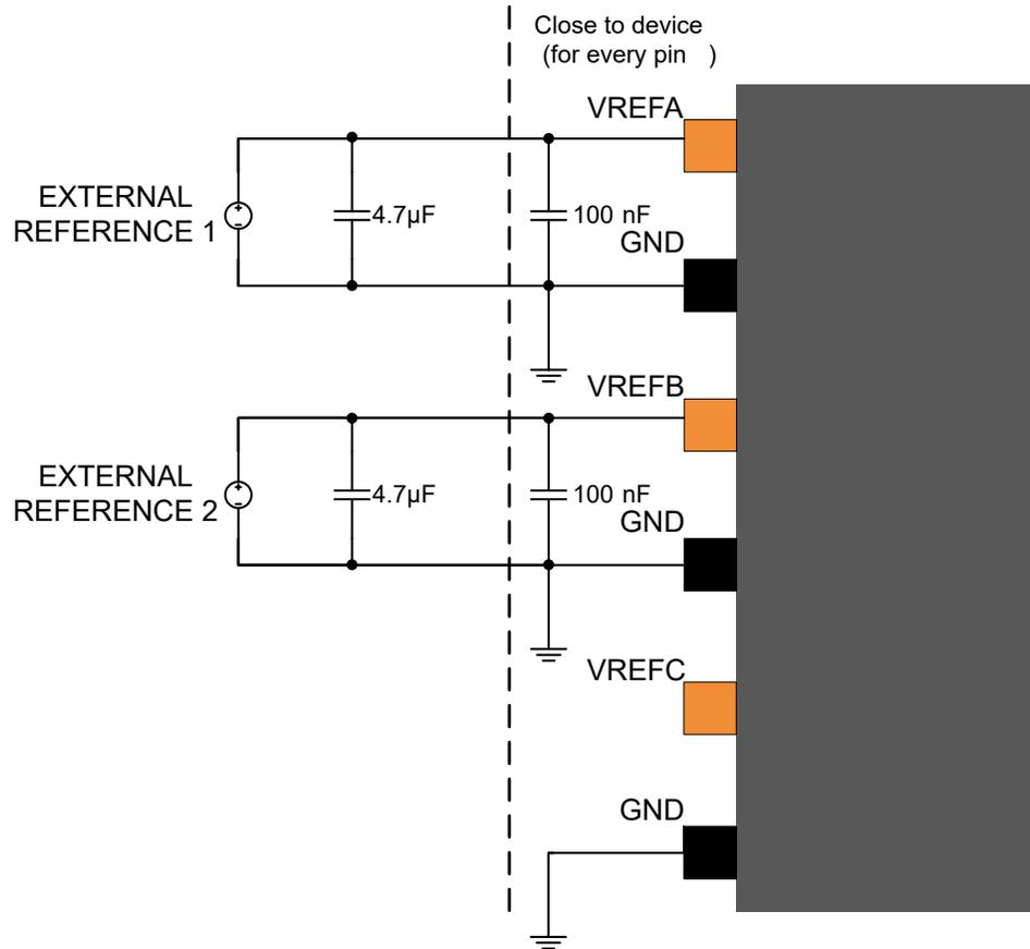
Figure 60-6. External Analog Reference Schematic With One Reference
