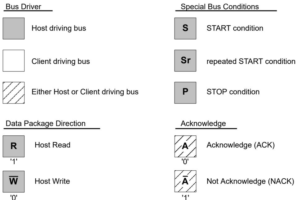
Figure 36-3. Basic I<sup>2</sup>C Transaction Diagram
