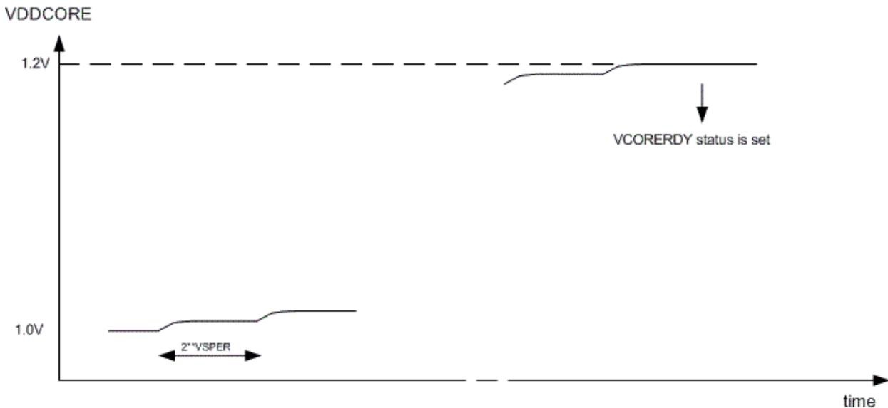
The STATUS.VCORERDY bit is set to '1' as soon as the VDDCORE voltage has reached the target voltage. During voltage transition, STATUS.VCORERDY will read '0'. The Voltage Ready interrupt (VCORERDY) can be used to detect a 0-to-1 transition of STATUS.VCORERDY, see also [19.5.5. Interrupts](#).
