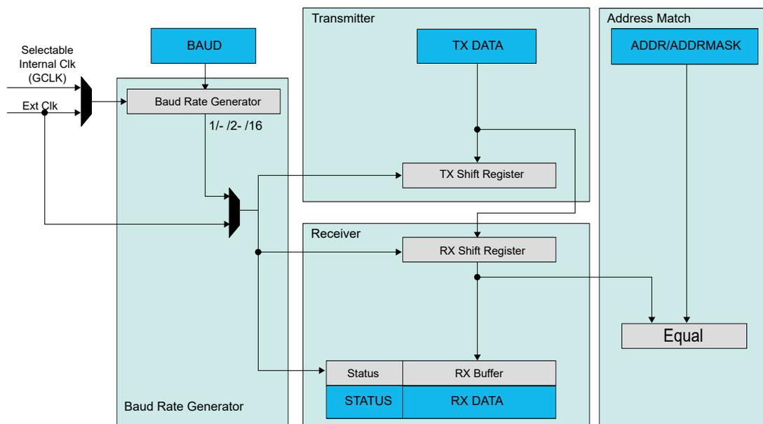
The transmitter consists of a single write buffer and a Shift register.
