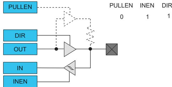
Figure 32-8. I/O Configuration - Output with Pull
