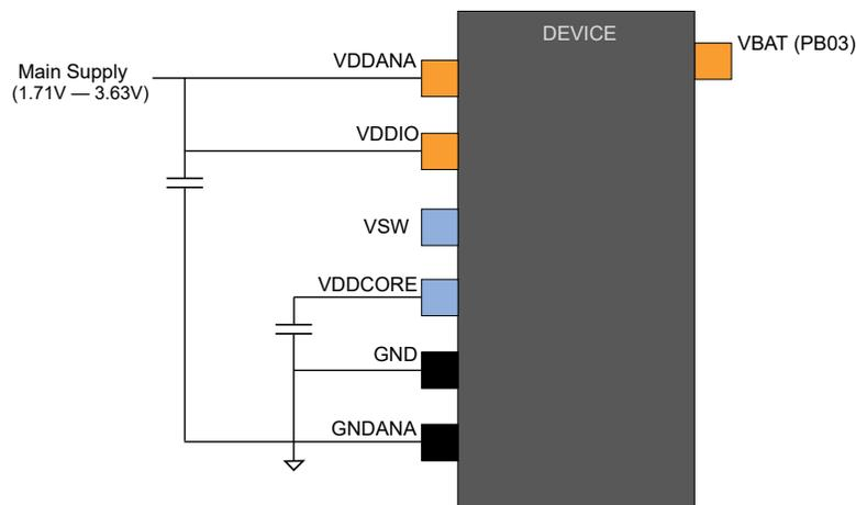
**Figure 7-3.** Power Supply Connection for Switching/Linear Mode
