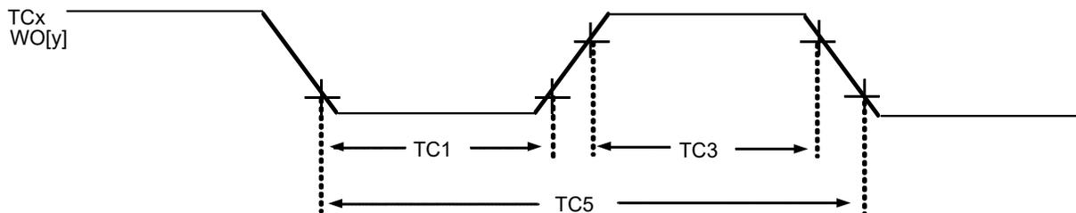
**Figure 54-25.** TCx Timer Compare Output Module Timing Diagrams
