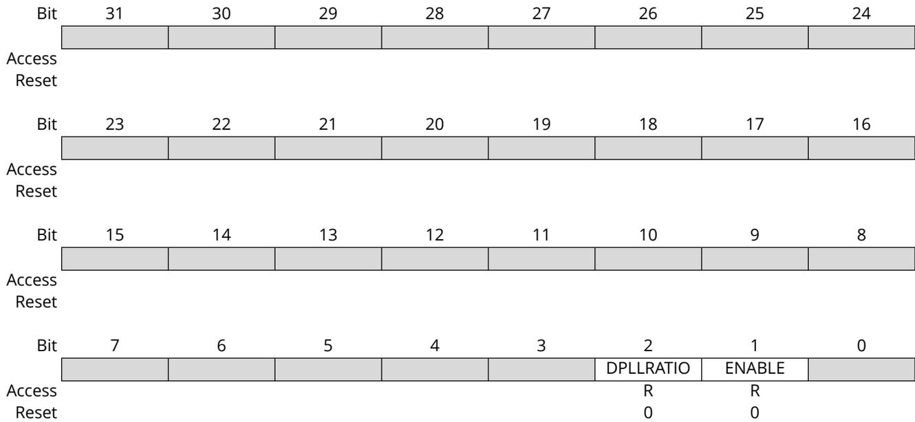
**Bit 2 - DPLLRRATIO** DPLL Loop Divider Ratio Synchronization Status
