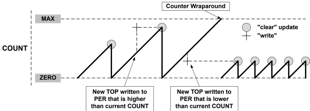
A counter wraparound can occur in any operation mode when up-counting without buffering, see [Figure 48-8](#).
