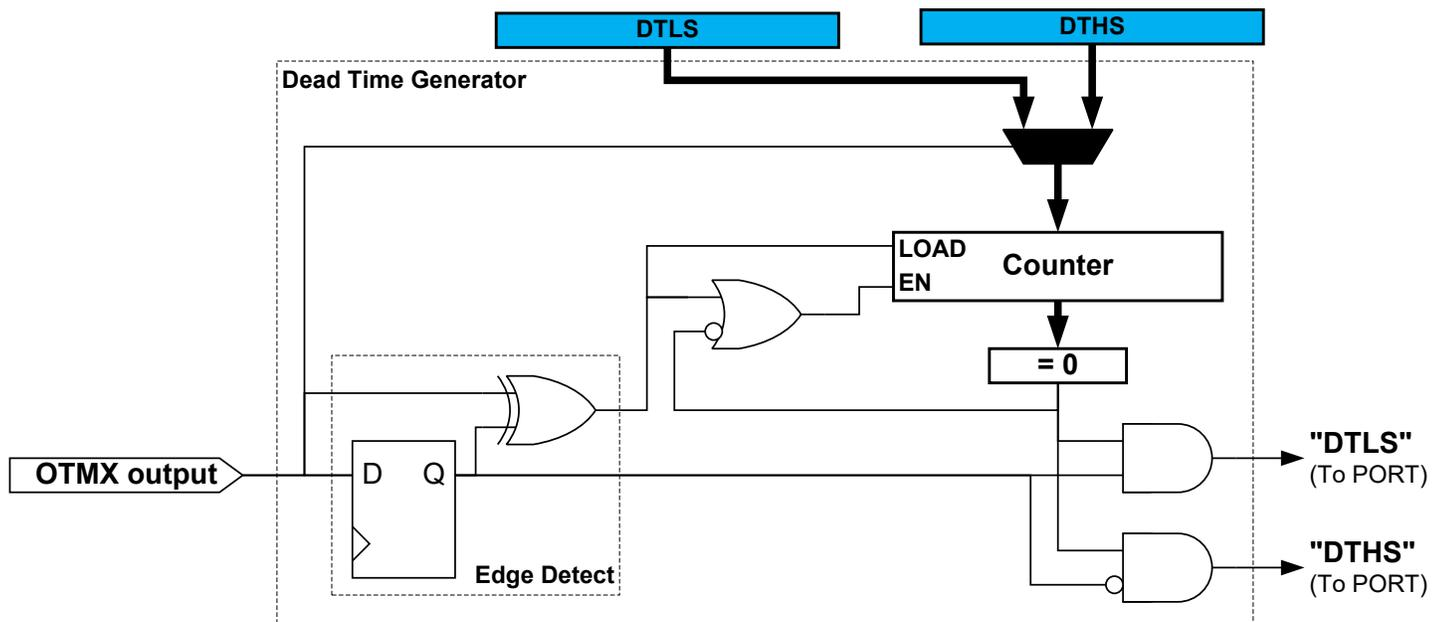
As shown in the following figure, the 8-bit dead-time counter is decremented by one for each peripheral clock cycle until it reaches zero. A non-zero counter value will force both the low side
