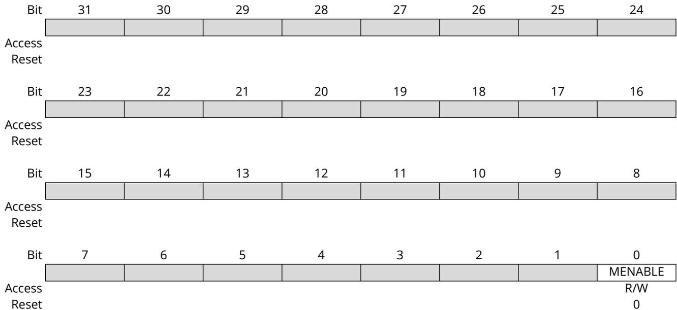
**Bit 0 - MENABLE** Cache Controller Monitor Enable
