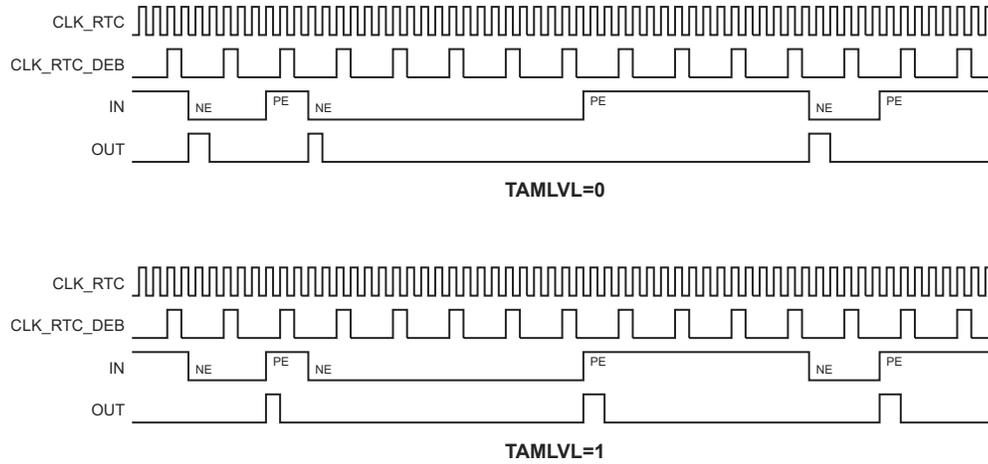
**Figure 21-6. Edge Detection with Synchronous Stability Debouncing**
