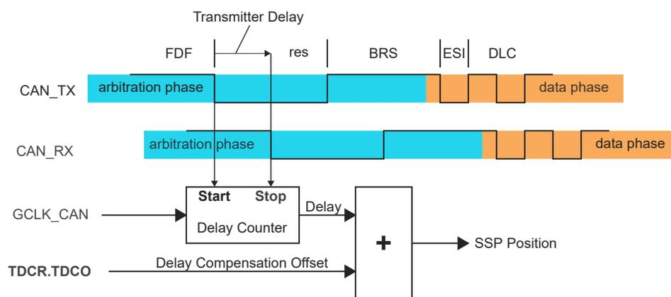
To avoid that a dominant glitch inside the received FDF bit ends the delay compensation measurement before the falling edge of the received res bit, resulting in a too early SSP position, the use of a transmitter delay compensation filter window can be enabled by programming TDCR.TDCF. This defines a minimum value for the SSP position. Dominant edges of CAN\_RX, that would result
