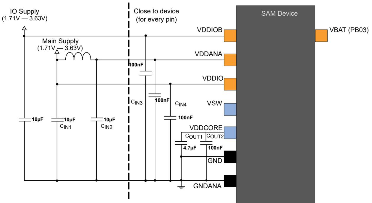
**Figure 60-3.** Power Supply Connection for Battery Backup
