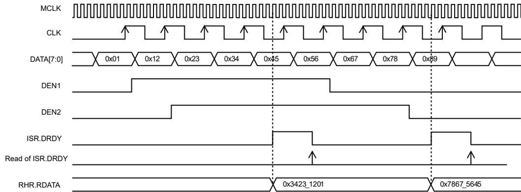
**Figure 52-7.** PCC Waveforms (ISIZE=10\_BITS, DSIZE=2\_DATA, ALWAYS = 1, HALFS = 0, SCALE = 0)
