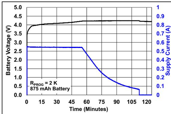
**FIGURE 6-2:** Typical Charge Profile (875 mAh Battery).
