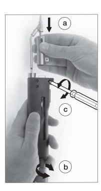
**Recommended**: Remove the lid in a vertical position to empty the tin residue and follow the cleaning guidelines in the tool and station manuals.
