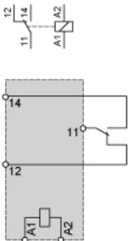
NOTE: For DC input, A1 have to be +, otherwise it would short circuit from protection module
