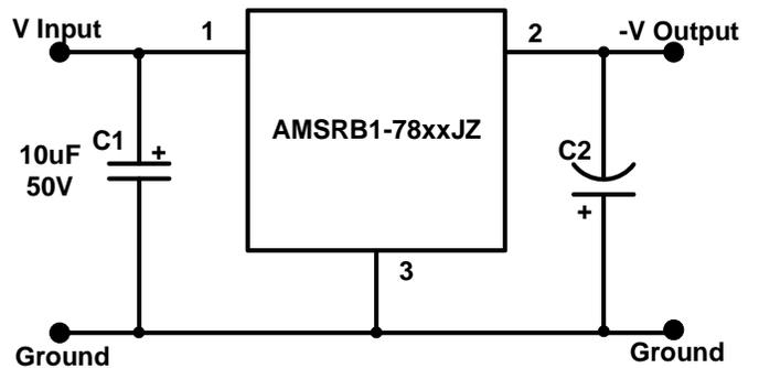
**Positive and Negative dual output application circuit**
