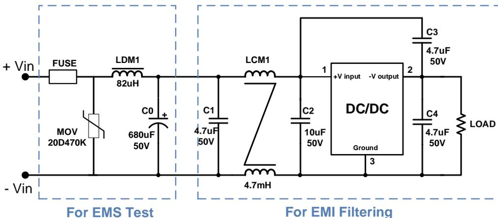
The part choice of the FUSE is based on actual input current.
