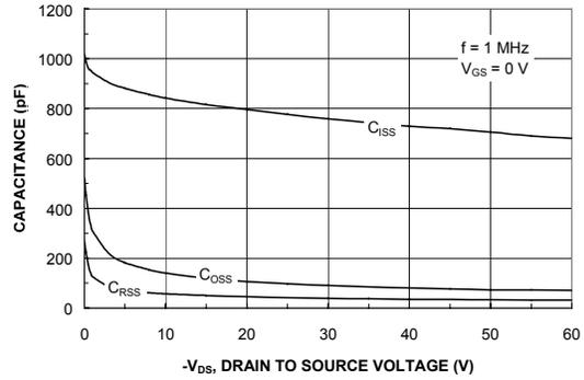
Figure 8. Capacitance Characteristics.
