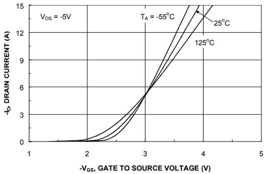
Figure 5. Transfer Characteristics.
