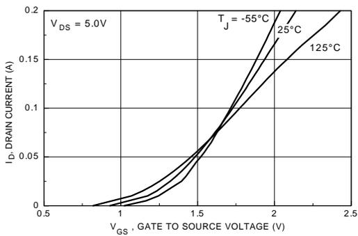
Figure 5. Transfer Characteristics.
