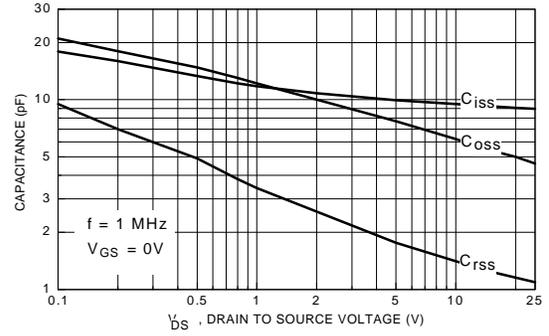
Figure 8. Capacitance Characteristics.
