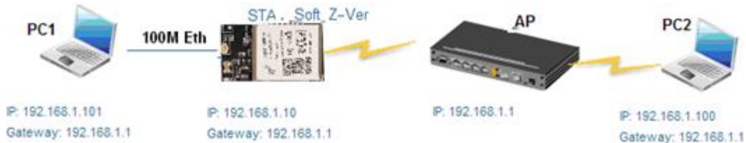
Figure 20. HF-A21-SMT Ethernet Interface Networking (As STA, Z-Ver)
