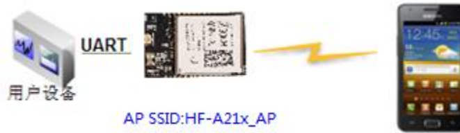
Figure 34. Wireless Control Application
