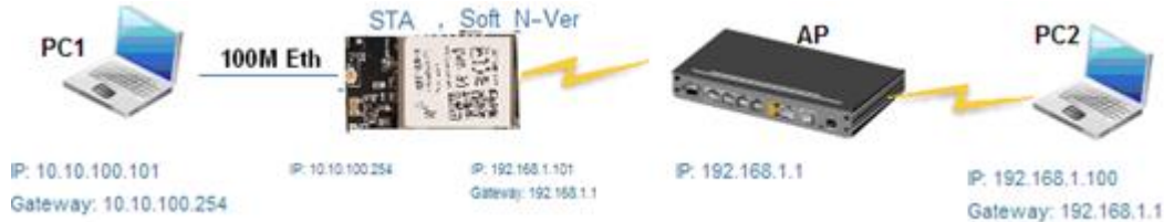
Figure 19. HF-A21-SMT Ethernet Interface Networking (As STA, N-Ver)
