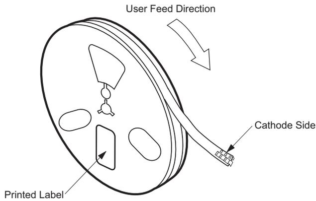
**NOTE:** Diameter ID should be bigger than 2.3 mm.
