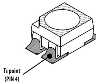
$T_S$  can be easily measured by mounting a thermocouple on the soldering joint as shown in preceding figure, while  $R_{\theta J-S}$  is provided in the data sheet. Verify the  $T_S$  of the LED in the final product to ensure that the LEDs are operating within all maximum ratings stated in the data sheet.
