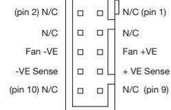
Signals Connector 10 way 2 mm pitch p/n JST B10B-PHDS5
