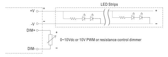
$\ensuremath{\,\%\,}$  DO NOT connect "DIM- to -V"
