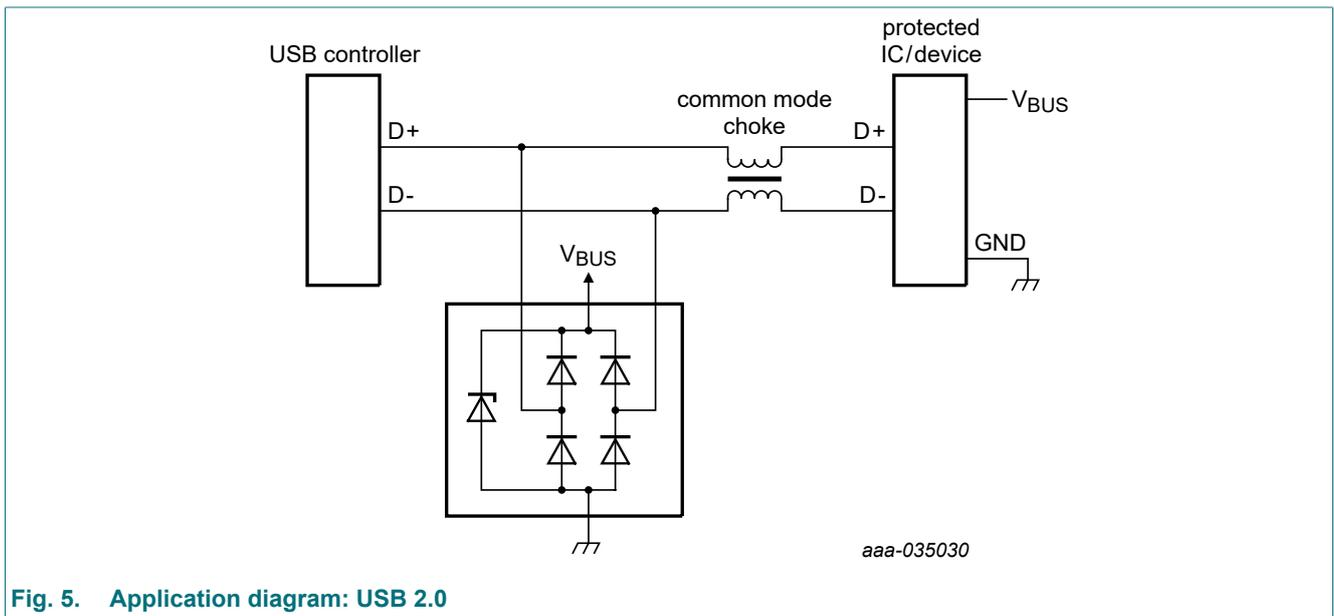
Fig. 5. Application diagram: USB 2.0
