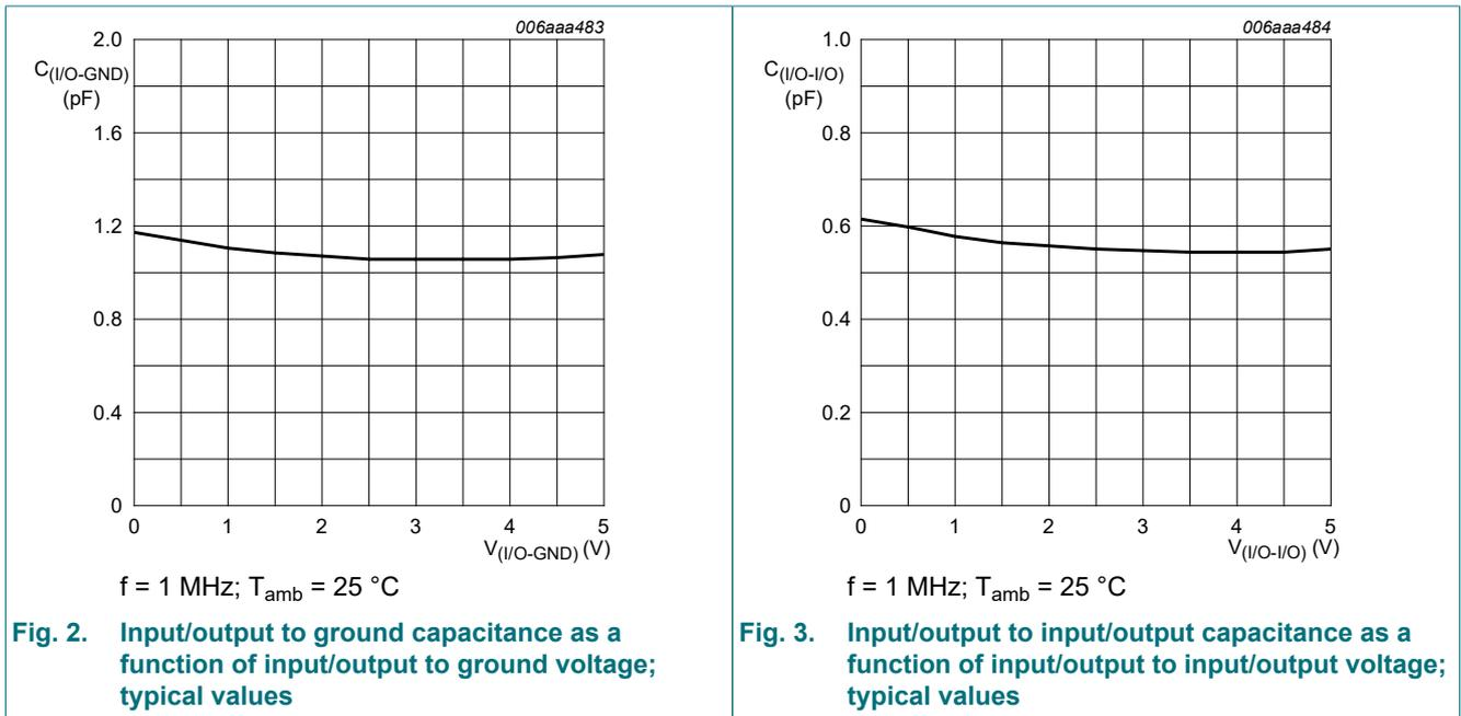
Ultra low capacitance double rail-to-rail ESD protection diode
