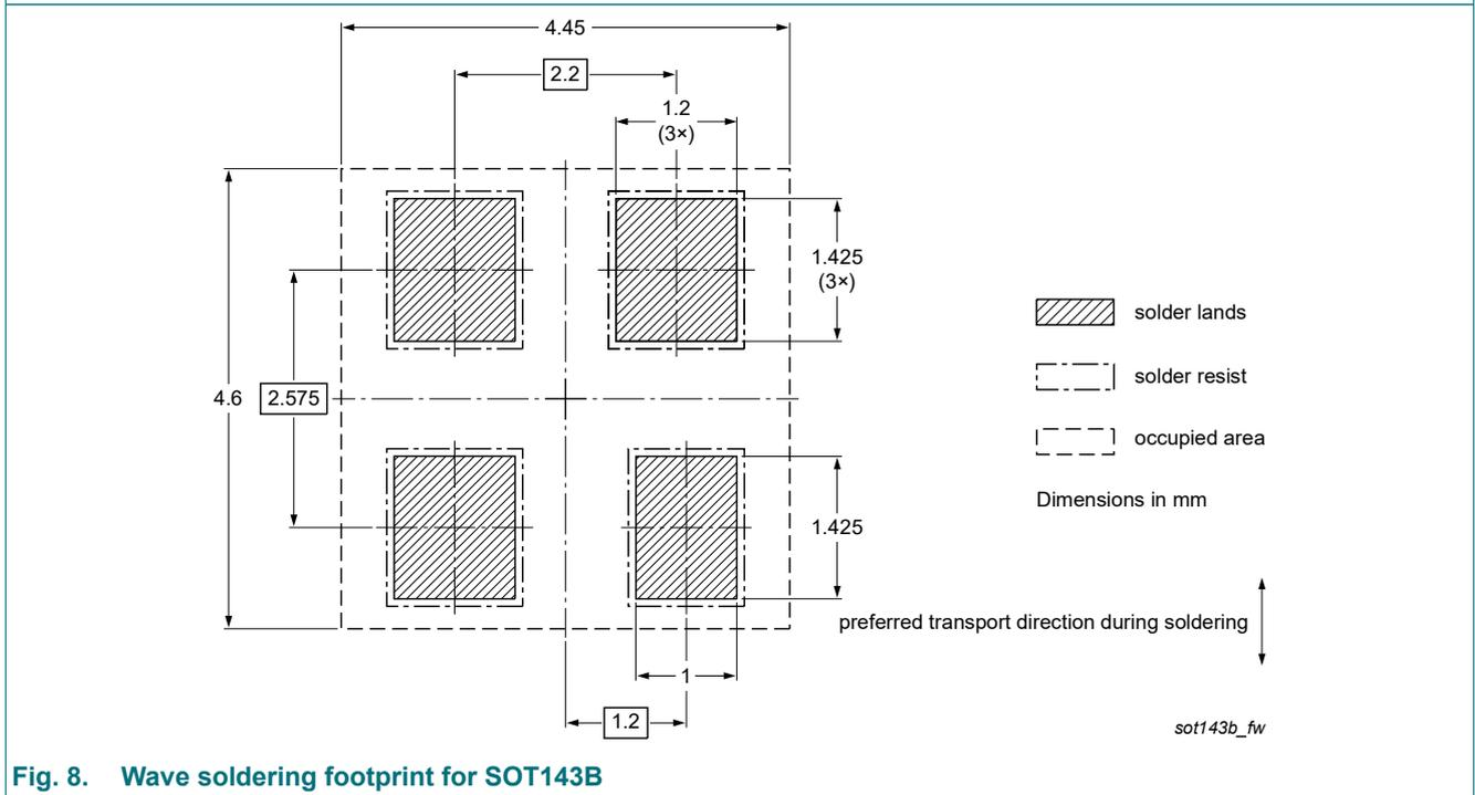
Fig. 8. Wave soldering footprint for SOT143B
