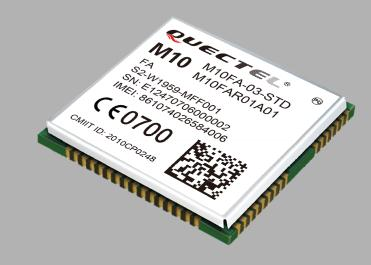
M10 is a Quad-band GSM/GPRS module in an LCC type which can be embedded in customer applications, offering the highest reliability and robustness. It adopts the laestest MTK chipset and features compact size of  $29 \times 29 \times 3.6$ mm, ultra low power consumption and extended temperature range.
