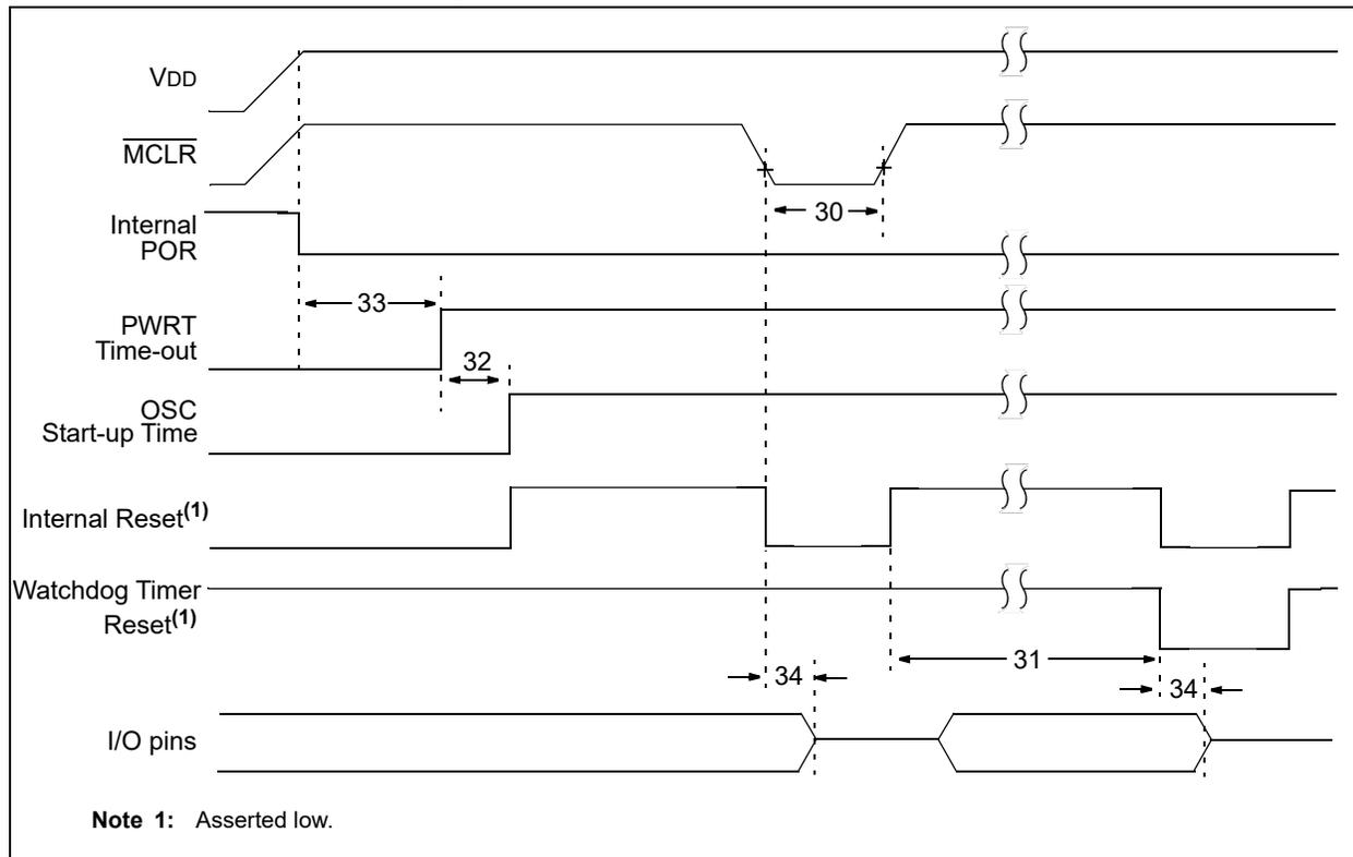
**TABLE 34-11: RESET, WATCHDOG TIMER, OSCILLATOR START-UP TIMER, POWER-UP TIMER AND BROWN-OUT RESET PARAMETERS**
