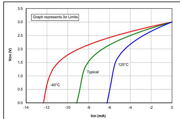
**FIGURE 35-53:**  $V_{OH}$  vs.  $I_{OH}$  Over Temperature,  $V_{DD} = 3.0V$ .
