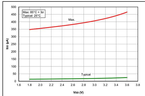
**FIGURE 35-47:**  $I_{DD}$ , ADC Nonconverting, PIC16LF1717/8/9 Only.
