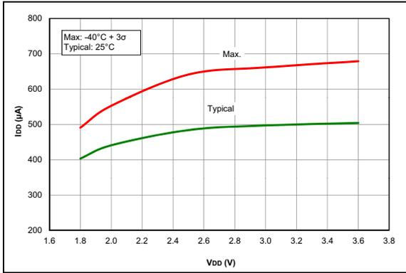
**FIGURE 35-49:**  $I_{PD}$ , Comparator, NP Mode ( $C_{xSP} = 1$ ), PIC16LF1717/8/9 Only.
