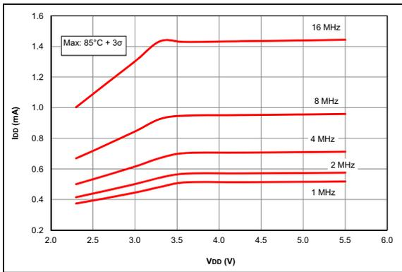
**FIGURE 35-26:**  $I_{DD}$  Maximum, HFINTOSC Mode, PIC16F1717/8/9 Only.
