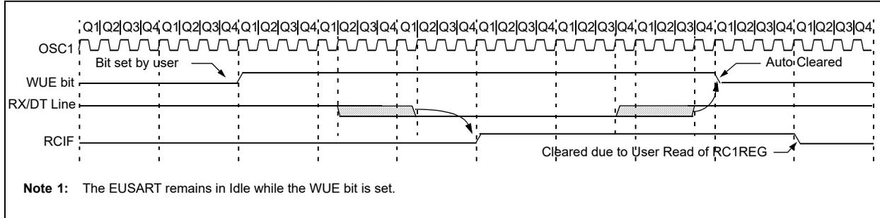
**FIGURE 31-8: AUTO-WAKE-UP (WUE) BIT TIMINGS DURING SLEEP**
