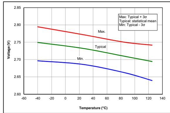
**FIGURE 35-65:** Brown-out Reset Voltage, High Trip Point ( $BORV = 0$ ).
