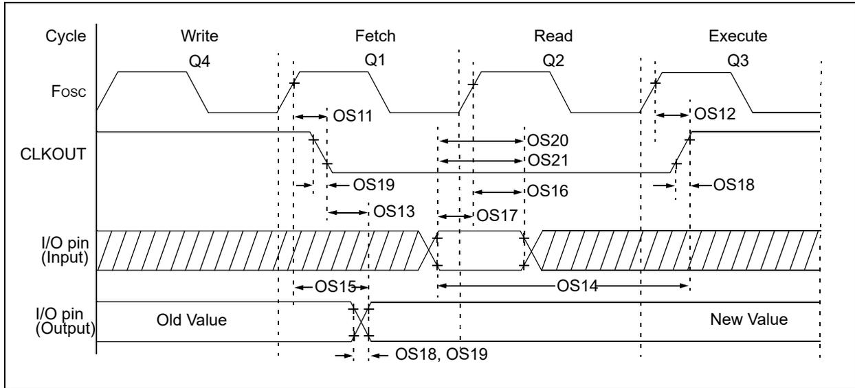
**TABLE 34-10: CLKOUT AND I/O TIMING PARAMETERS**
