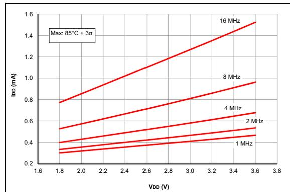
**FIGURE 35-24:**  $I_{DD}$  Maximum, HFINTOSC Mode, PIC16LF1717/8/9 Only.
