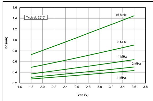
**FIGURE 35-23:**  $I_{DD}$  Typical, HFINTOSC Mode, PIC16LF1717/8/9 Only.
