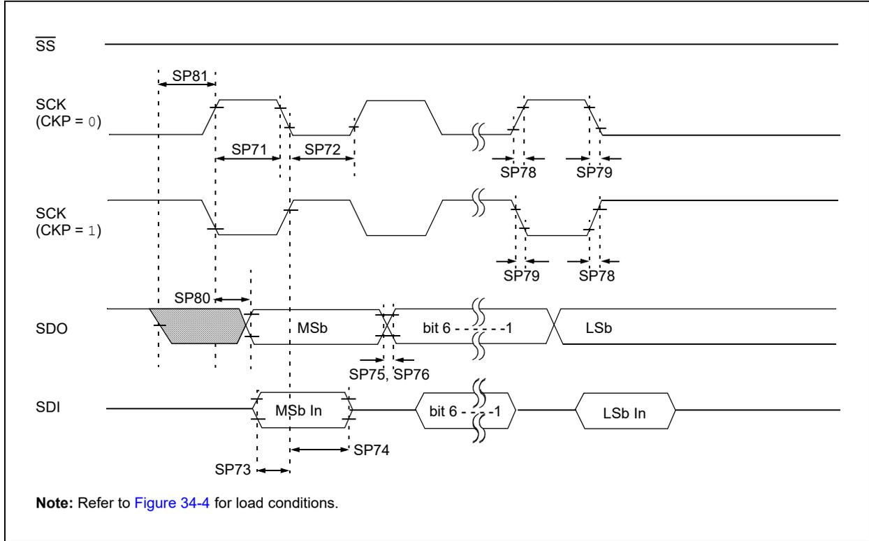
**FIGURE 34-18: SPI HOST MODE TIMING (CKE = 1, SMP = 1)**
