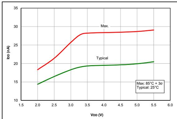
**FIGURE 35-38:**  $I_{PD}$ , Fixed Voltage Reference (FVR), PIC16F1717/8/9 Only.
