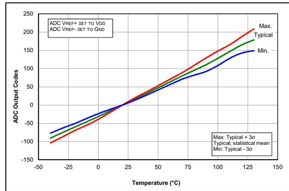
**FIGURE 35-89:** Temp. Indicator Slope Normalized to  $20^\circ\text{C}$ , High Range,  $V_{DD} = 3.0\text{V}$ , PIC16F1717/8/9 Only.
