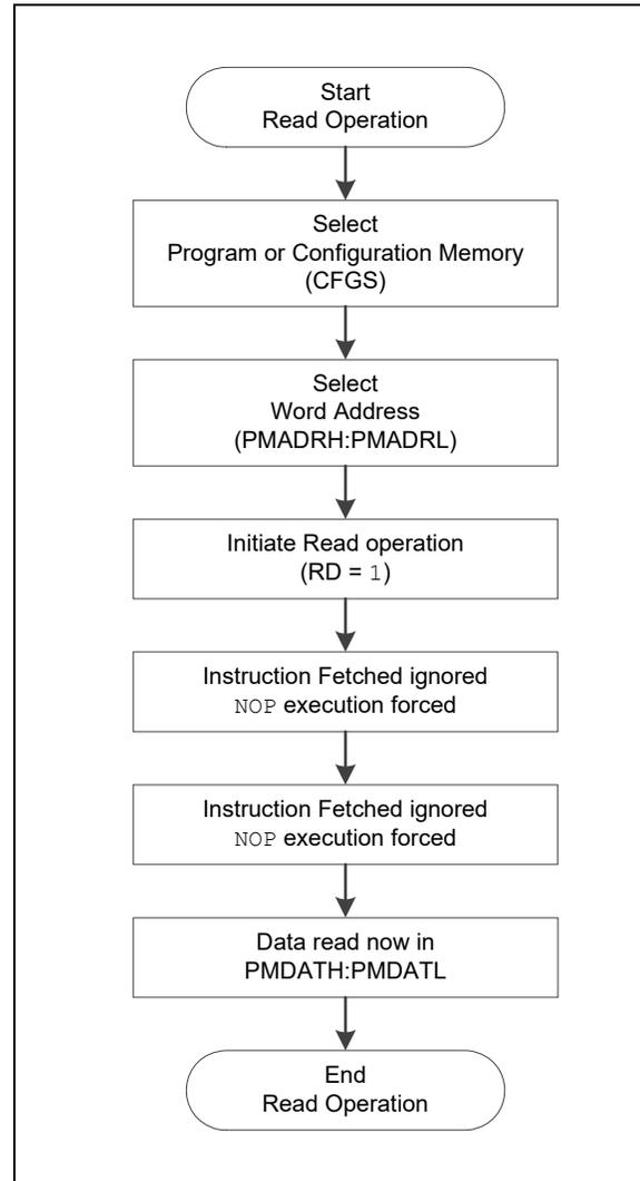
**FIGURE 10-2: FLASH PROGRAM MEMORY READ CYCLE EXECUTION**
