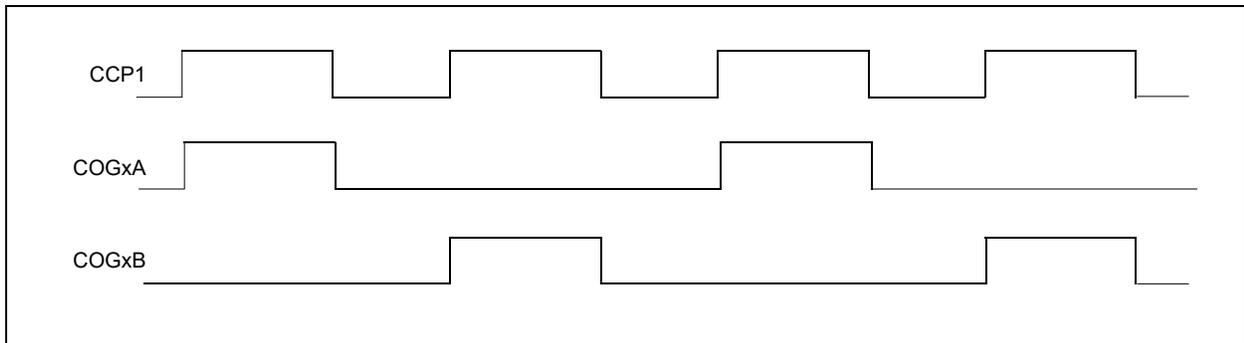
**FIGURE 18-12: FULL-BRIDGE FORWARD MODE COG OPERATION WITH CCP1**
