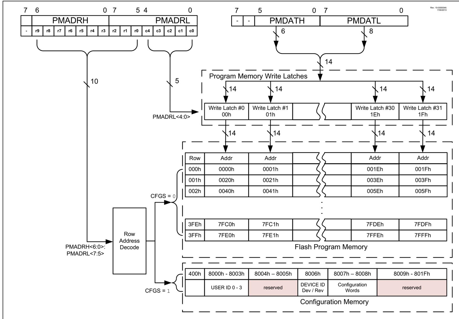
**FIGURE 10-6: FLASH PROGRAM MEMORY WRITE FLOWCHART**
