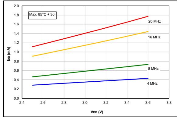
**FIGURE 35-28:**  $I_{DD}$  Maximum, HS Oscillator, PIC16LF1717/8/9 Only.
