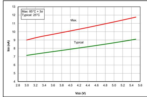
**FIGURE 35-40:**  $I_{PD}$ , Brown-out Reset (BOR), BORV = 1, PIC16F1717/8/9 Only.
