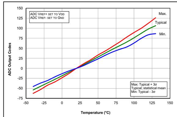
**FIGURE 35-90:** Temp. Indicator Slope Normalized to  $20^\circ\text{C}$ , Low Range,  $V_{DD} = 3.0\text{V}$ , PIC16F1717/8/9 Only.
