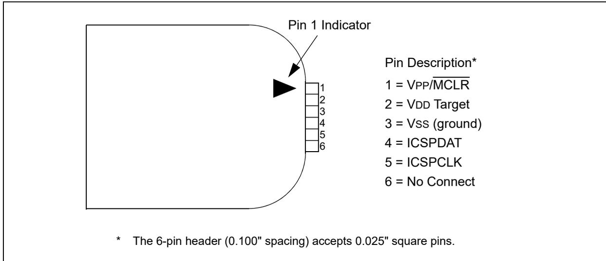
**FIGURE 32-3: TYPICAL CONNECTION FOR ICSP™ PROGRAMMING**
