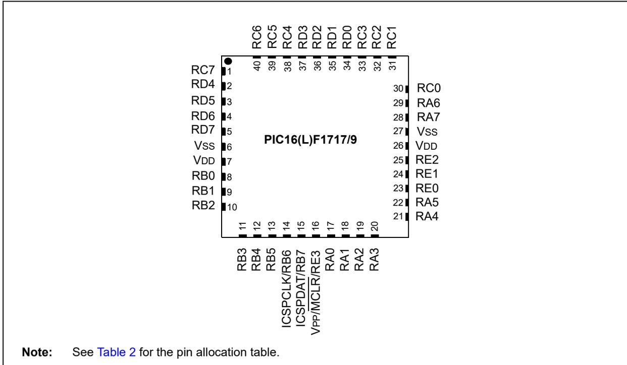
**FIGURE 5: 44-PIN TQFP (10X10)**
