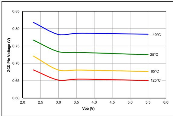
**FIGURE 35-115:** ZCD Pin Voltage, Typical Measured Values
