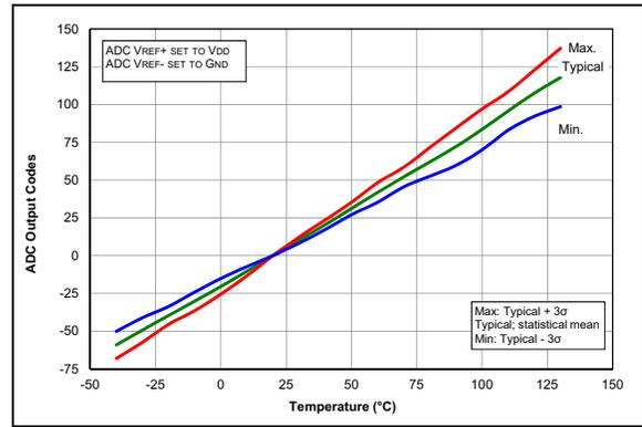
**FIGURE 35-88:** Temp. Indicator Slope Normalized to  $20^\circ\text{C}$ , High Range,  $V_{DD} = 5.5\text{V}$ , PIC16F1717/8/9 Only.
