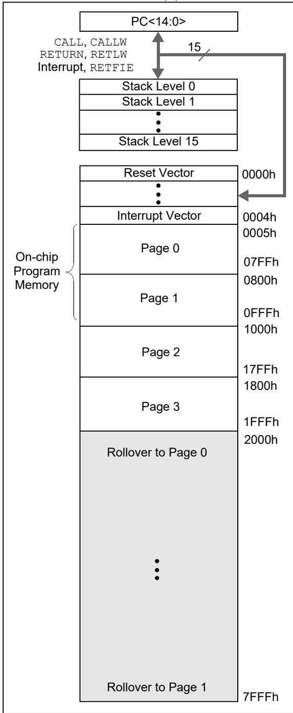
**FIGURE 3-2: PROGRAM MEMORY MAP AND STACK FOR PIC16(L)F1718/9**
