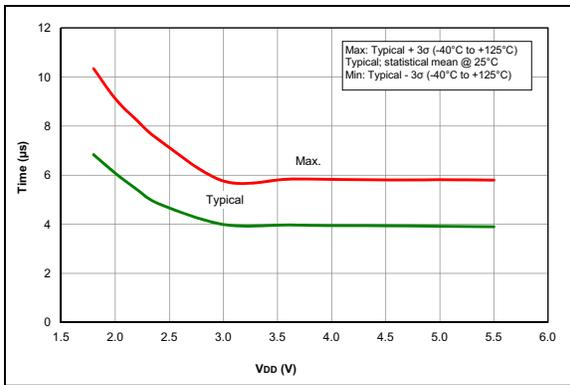
**FIGURE 35-74:** Wake From Sleep,  $V_{REGPM} = 0$ .
