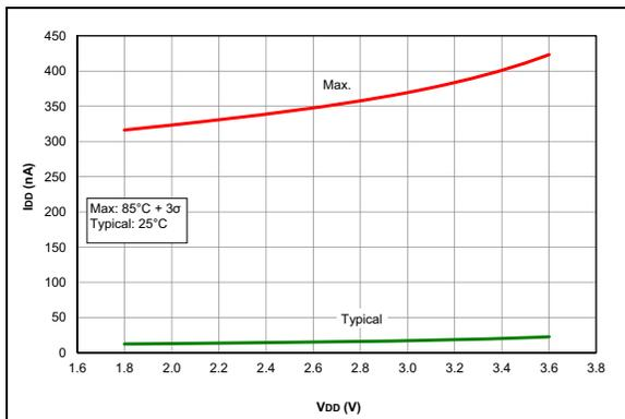
**FIGURE 35-33:**  $I_{PD}$  Base, LP Sleep Mode, PIC16F1717/8/9 Only.
