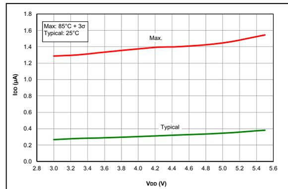
**FIGURE 35-42:**  $I_{PD}$ , LP Brown-out Reset (LPBOR = 0), PIC16F1717/8/9 Only.
