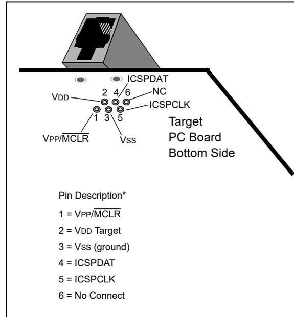
Another connector often found in use with the PICkit™ programmers is a standard 6-pin header with 0.1 inch spacing. Refer to [Figure 32-2](#).
