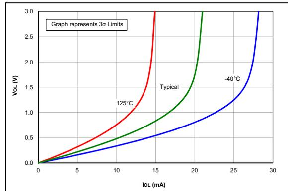
**FIGURE 35-54:**  $V_{OL}$  vs.  $I_{OL}$  Over Temperature,  $V_{DD} = 3.0V$ .
