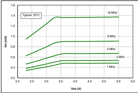
**FIGURE 35-25:**  $I_{DD}$  Typical, HFINTOSC Mode, PIC16F1717/8/9 Only.
