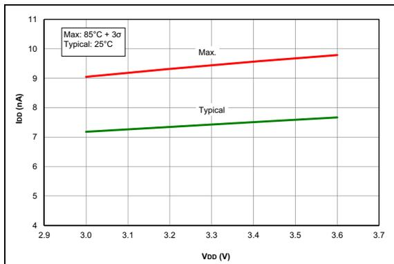
**FIGURE 35-39:**  $I_{PD}$ , Brown-out Reset (BOR), BORV = 1, PIC16LF1717/8/9 Only.
