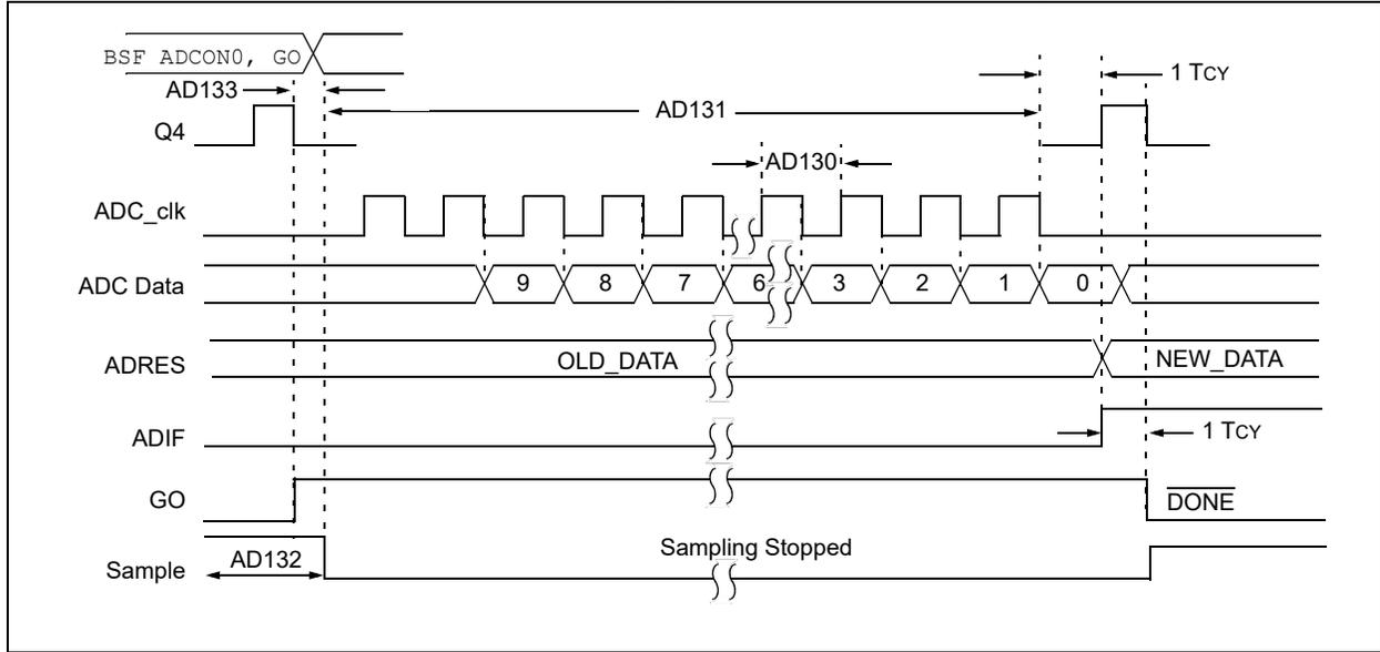
**FIGURE 34-14: ADC CONVERSION TIMING (ADC CLOCK FROM FRC)**
