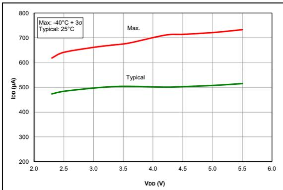
**FIGURE 35-50:**  $I_{PD}$ , Comparator, NP Mode ( $C_{xSP} = 1$ ), PIC16F1717/8/9 Only.
