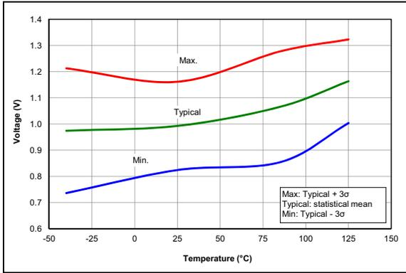
**FIGURE 35-73:** POR Rearm Voltage, NP Mode, PIC16LF1717/8/9 Only.
