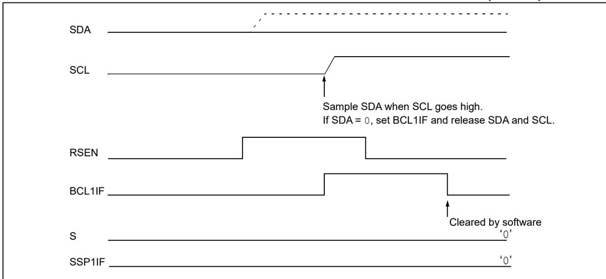
**FIGURE 30-37: BUS COLLISION DURING REPEATED START CONDITION (CASE 2)**
