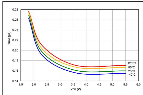
**FIGURE 35-119:** COG Dead-Band Delay,  $DBR/DBF = 32$ , Typical Measured Values
