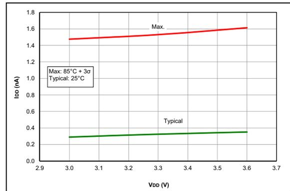
**FIGURE 35-41:**  $I_{PD}$ , LP Brown-out Reset (LPBOR = 0), PIC16LF1717/8/9 Only.
