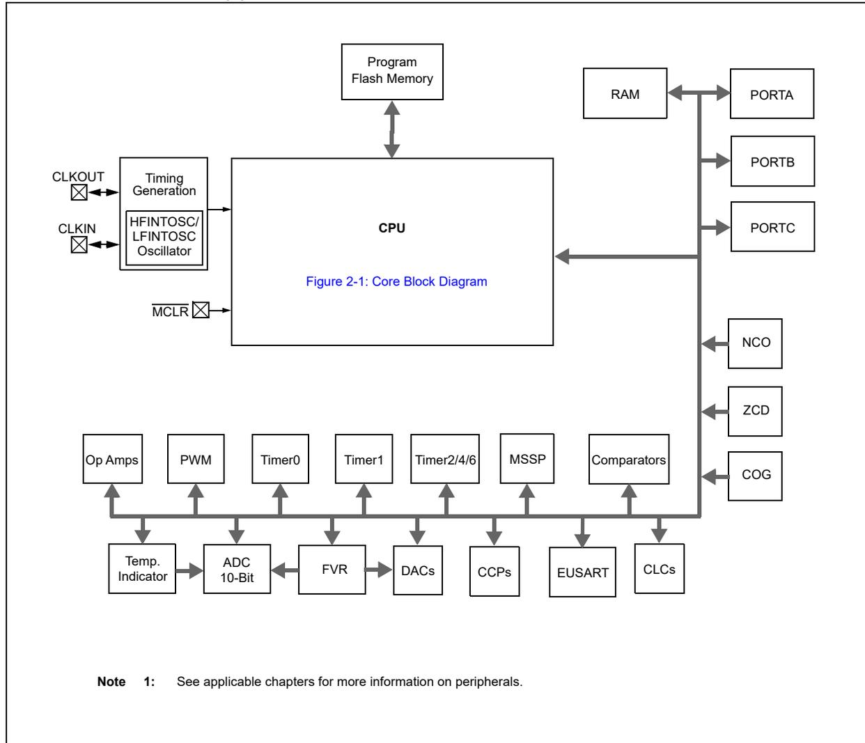
**FIGURE 1-2: PIC16(L)F1717/9 BLOCK DIAGRAM**
