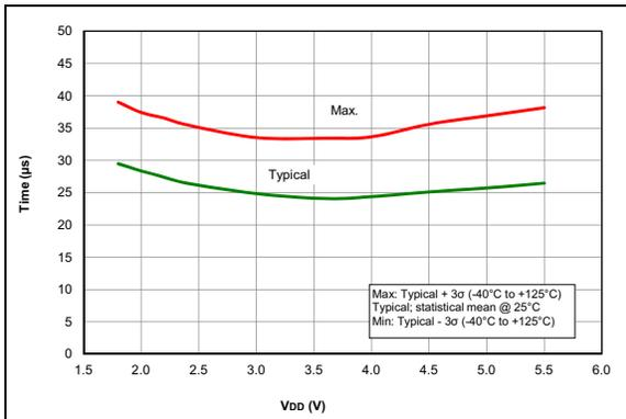
**FIGURE 35-75:** Wake From Sleep,  $V_{REGPM} = 1$ .
