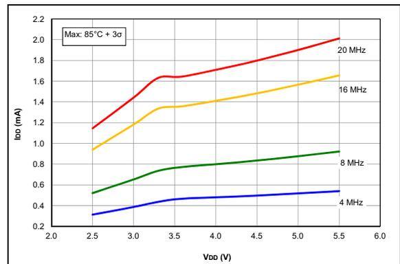
**FIGURE 35-30:**  $I_{DD}$  Maximum, HS Oscillator, PIC16F1717/8/9 Only.
