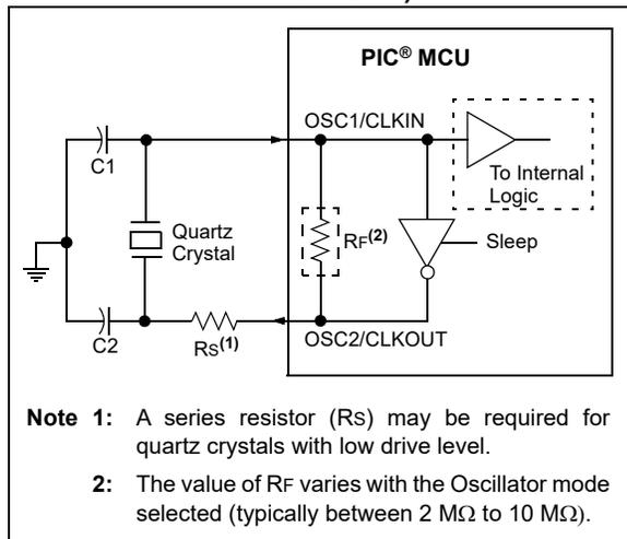
**Note 1:** Quartz crystal characteristics vary according to type, package and manufacturer. The user needs to consult the manufacturer data sheets for specifications and recommended application.
