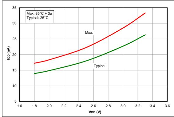
**FIGURE 35-37:**  $I_{PD}$ , Fixed Voltage Reference (FVR), PIC16LF1717/8/9 Only.
