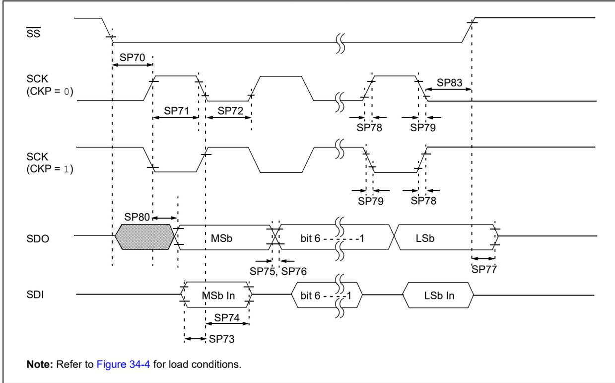
**FIGURE 34-20: SPI CLIENT MODE TIMING (CKE = 1)**
