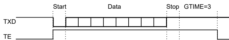
Figure 31-15. Example of TE Drive with Guard Time
