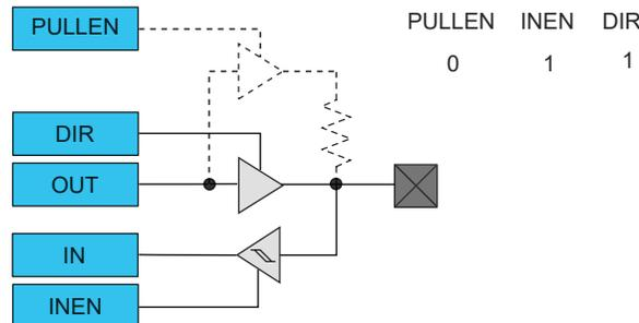
**Figure 23-8. I/O Configuration - Output with Pull**
