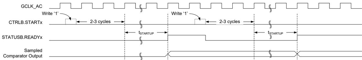
For low-power operation, event-triggered measurements can be performed during sleep modes. When the event occurs, the Power Manager will start CLK\_AC\_DIG. The comparator is enabled, and after the startup time has passed, a comparison is done and appropriate peripheral events and interrupts are also generated. The comparator and CLK\_AC\_DIG are then disabled again automatically, unless configured to wake up the system from sleep.
