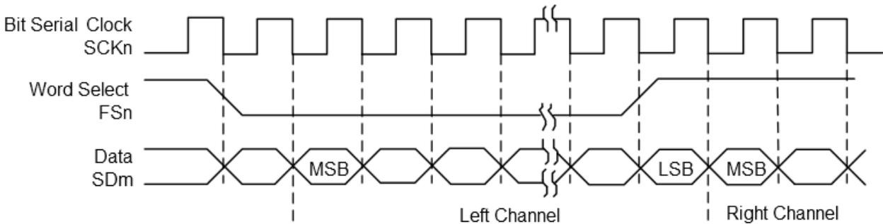
Data bits are sent on the falling edge of the Serial Clock and sampled on the rising edge of the Serial Clock. The Word Select line indicates the channel in transmission, a low level for the left channel and a high level for the right channel.
