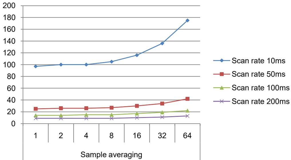
**Figure 41-9. Power Consumption [ $\mu\text{A}$ ]**
