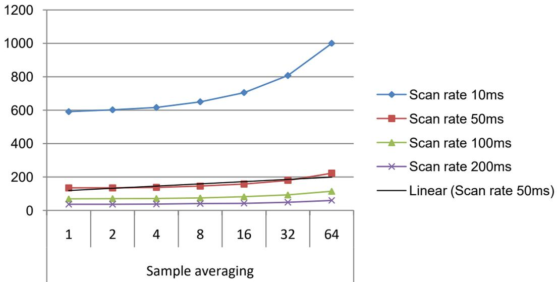
**Figure 37-10. Power Consumption [ $\mu$ A]**
