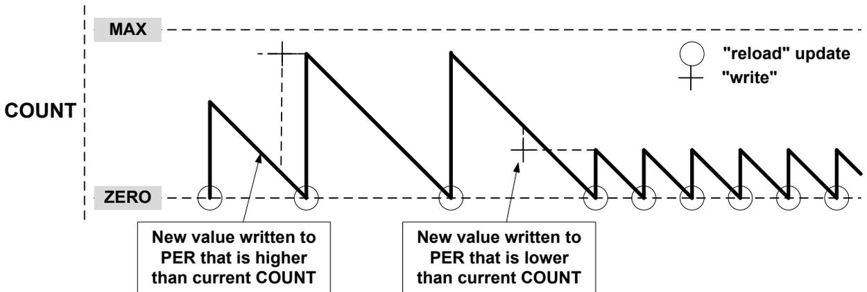
A counter wraparound can occur in any operation mode when up-counting without buffering, see [Figure 31-10](#). COUNT and TOP are continuously compared, so when a new value that is lower than the current COUNT is written to TOP, COUNT will wrap before a compare match.
