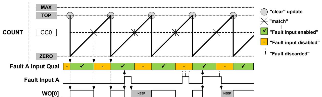
**Restart Action** This is enabled by writing the Fault n Restart bit in Recoverable Fault n Configuration register (FCTRLn.RESTART) to '1'. When enabled, the timer/counter will be restarted as soon as the corresponding fault condition is present. The ongoing cycle is stopped and the timer/counter starts a new cycle, see [Figure 31-26](#). In Ramp 1 mode, when the new cycle starts, the compare outputs will be clamped to inactive level as long as the fault condition is present.
