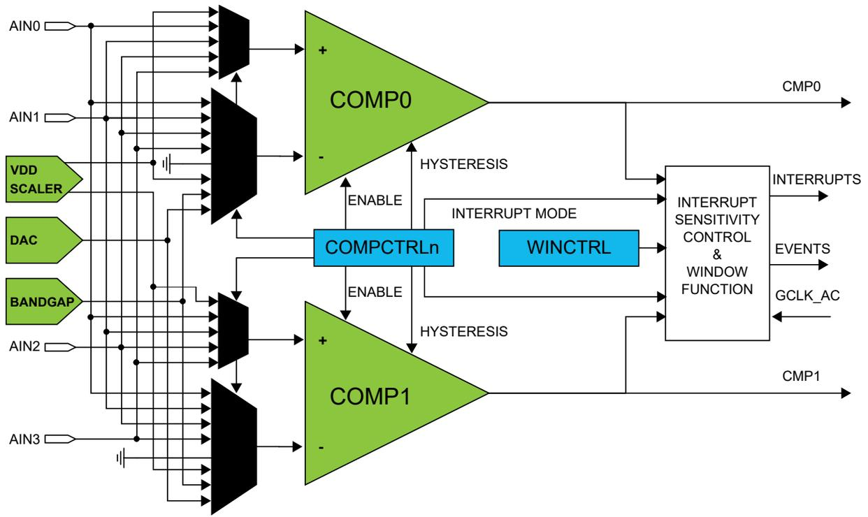
Figure 34-2. Analog Comparator Block Diagram (Second Pair)
