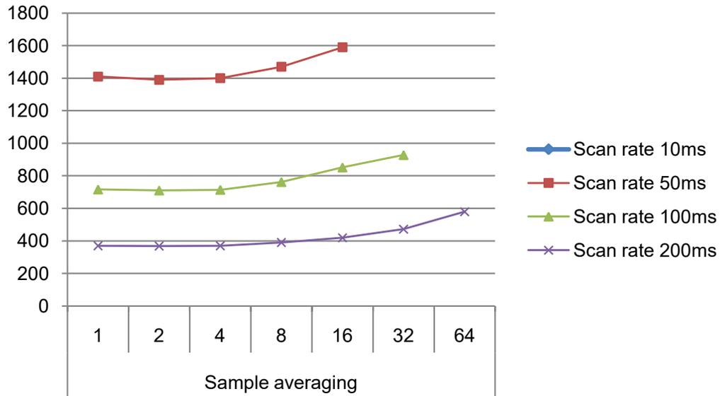
**Figure 37-13. CPU Utilization**
