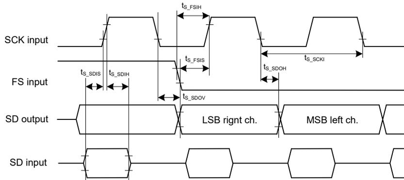
**Figure 41-26. I<sup>2</sup>S Timing PDM2 Mode**
