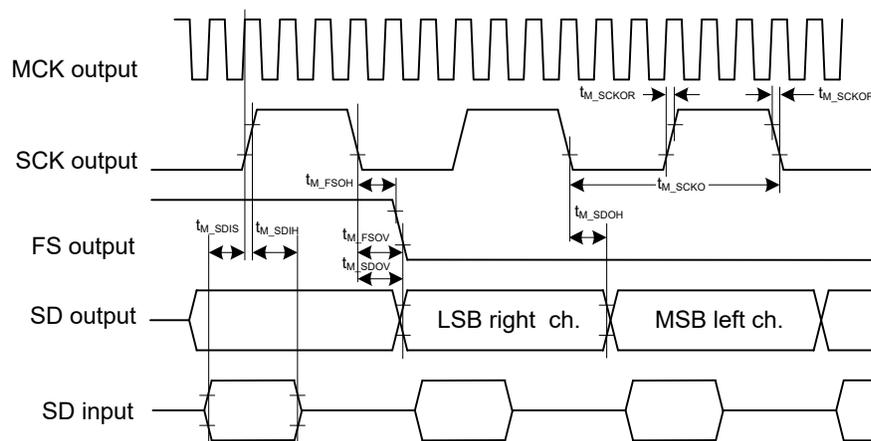
**Figure 41-25. I<sup>2</sup>S Timing Client Mode**
