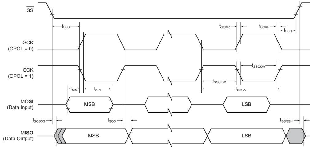
**Table 41-54. SPI Timing Characteristics and Requirements<sup>(1)</sup>**
