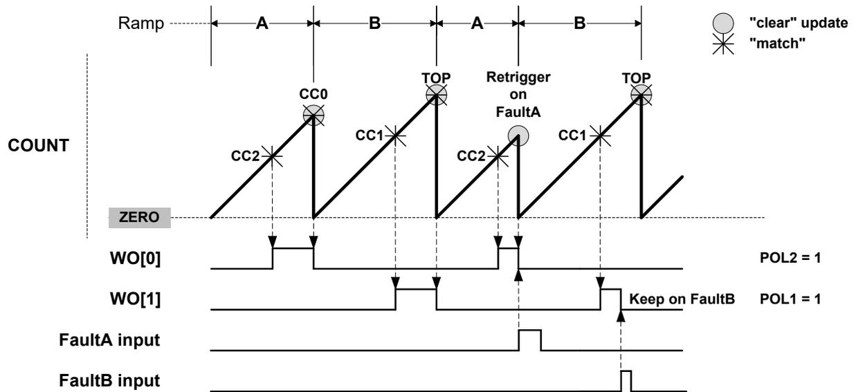
Figure 31-21. RAMP2 Critical Operation With 2 Channels
