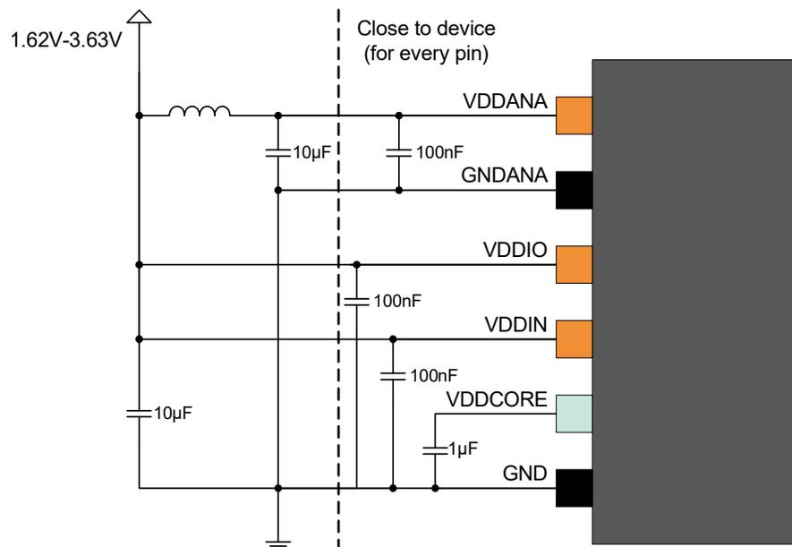
**Note:** 1. It is recommended to use a ceramic or solid tantalum capacitor with low ESR. Refer to table 37-18 in [37.11.1 Voltage Regulator Characteristics](#) for additional details on ESR.
