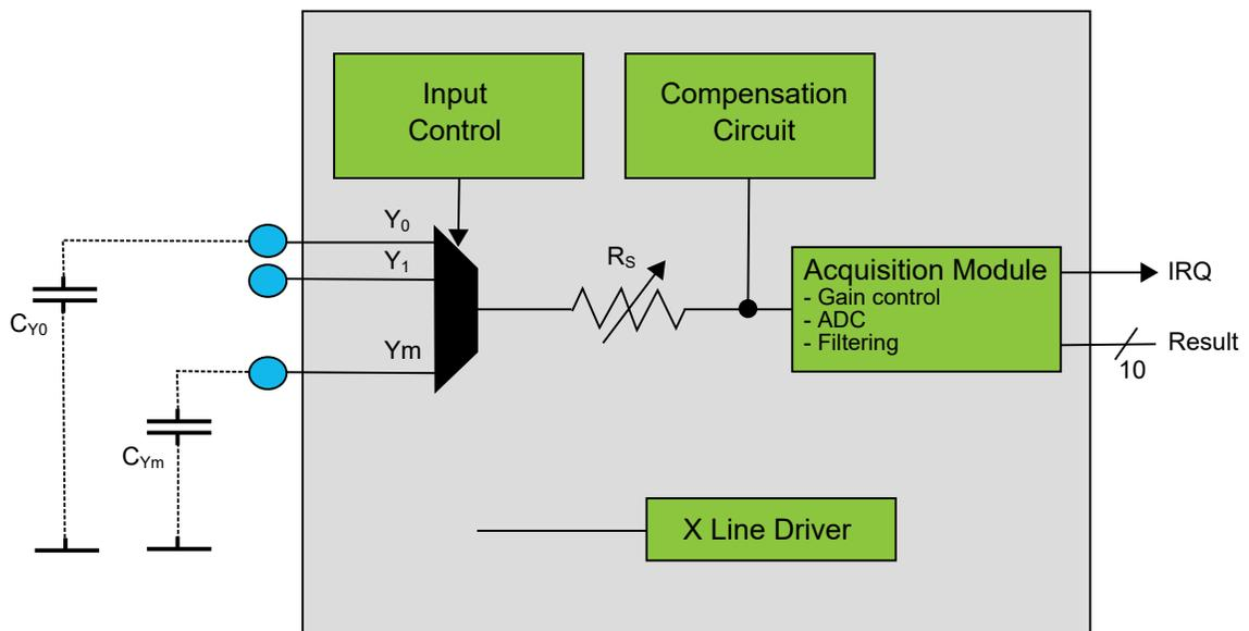
**Note:** For SAM D21 the  $R_S = 0, 20, 50, 100 \text{ K}\Omega$ .
