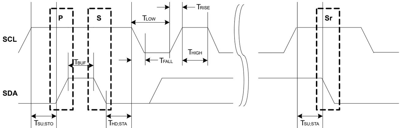
The following parameters are timed using the SCL low time period  $T_{LOW}$ . This comes from the Host Baud Rate Low bit group in the Baud Rate register (BAUD.BAUDLOW). When BAUD.BAUDLOW=0, or the Host Baud Rate bit group in the Baud Rate register (BAUD.BAUD) determines it.
