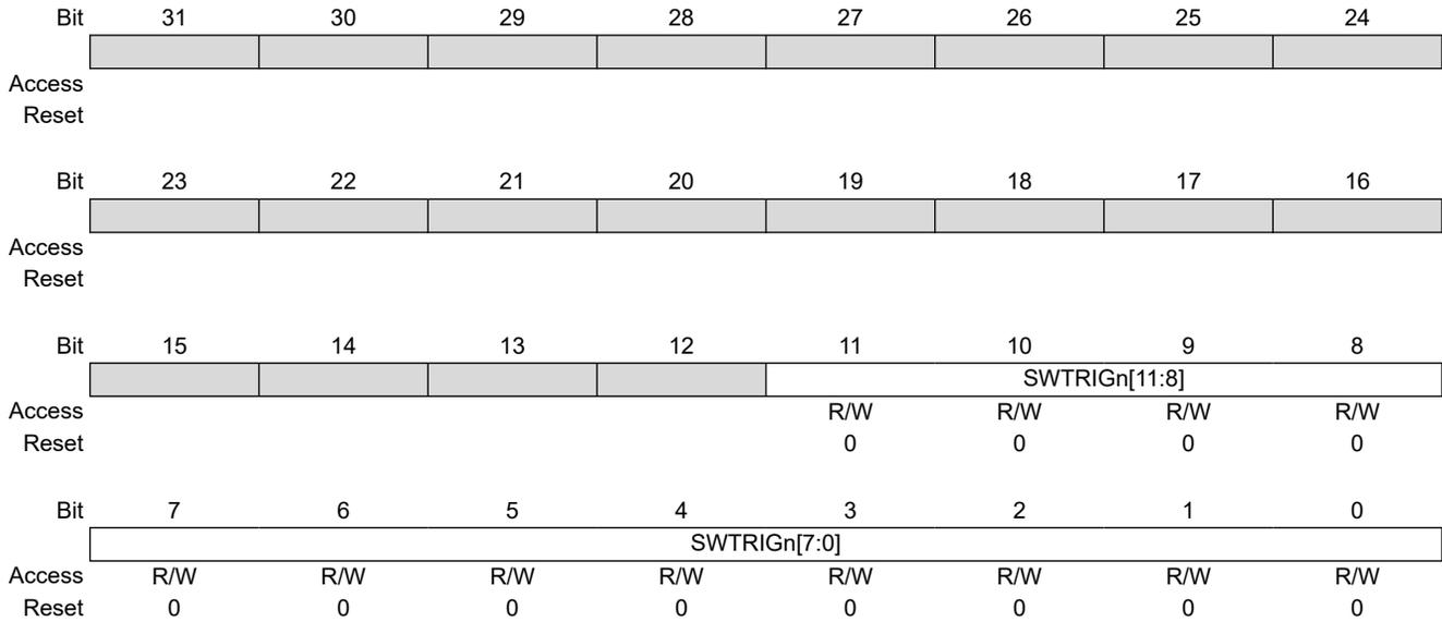
**Bits 11:0 – SWTRIGn[11:0]** Channel n Software Trigger [n = 11..0]
