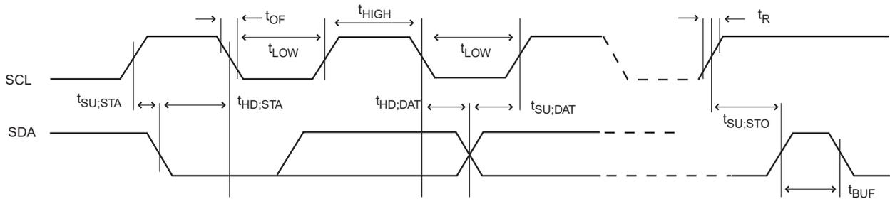
**Table 37-68. I<sup>2</sup>C Interface Timing (Device Variant A)**
