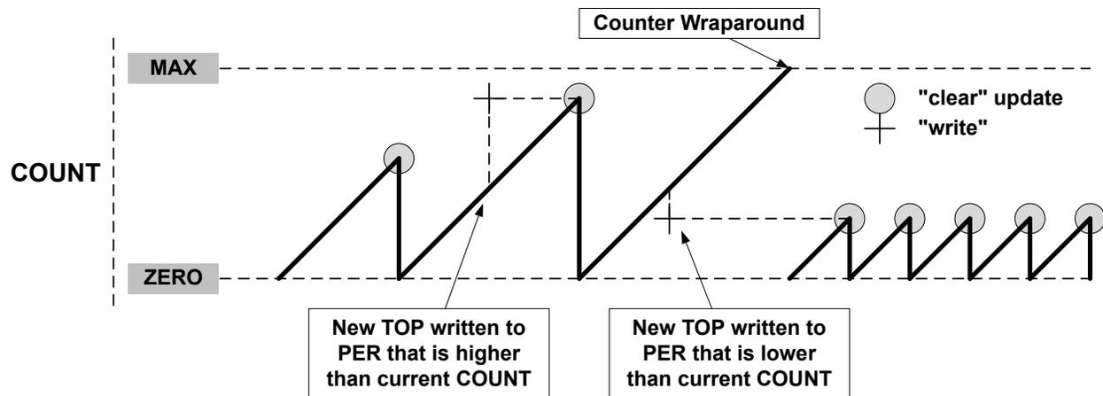
**Figure 30-8. Changing the Top Value with Down-Counting Operation**
