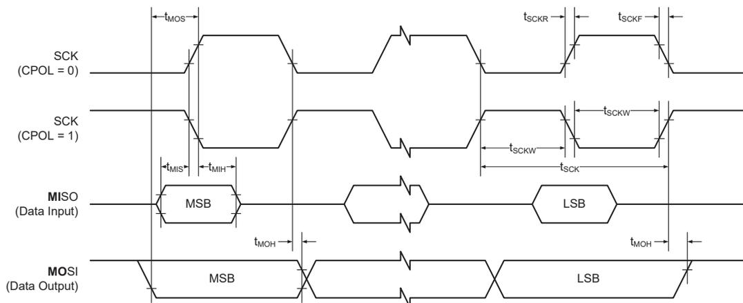
**Figure 41-21. SPI Timing Requirements in Client Mode**
