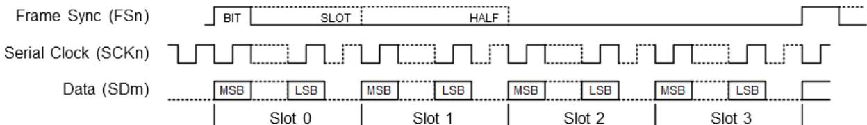
Data bits are sent on the falling edge of the Serial Clock and sampled on the rising edge of the Serial Clock. The FS<sub>n</sub> pin provides a frame synchronization signal, at the beginning of slot 0. The delay between the frame start and the first data bit is defined by writing the CLKCTRLn.BITDELAY field.
