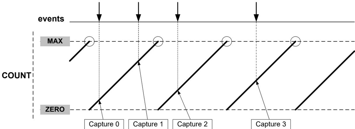
For input capture, the buffer register and the corresponding CCx act like a FIFO. When CCx is empty or read, any content in CCBx is transferred to CCx. The buffer valid flag is passed to set the CCx interrupt flag (IF) and generate the optional interrupt, event or DMA request. CCBx register value can't be read, all captured data must be read from CCx register.
