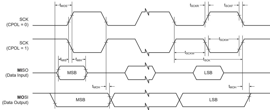
**Figure 37-21. SPI Timing Requirements in Client Mode**
