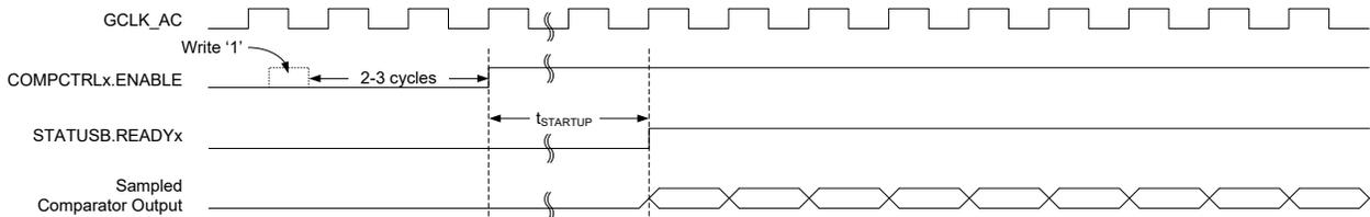
For low-power operation, comparisons can be performed during sleep modes without a clock. The comparator is enabled continuously, and changes of the comparator state are detected asynchronously. When a toggle occurs, the Power Manager will start CLK\_AC\_DIG to register the appropriate peripheral events and interrupts. The CLK\_AC\_DIG clock is then disabled again automatically, unless configured to wake up the system from sleep.
