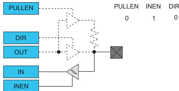
**Figure 23-5. I/O Configuration - Input with Pull**
