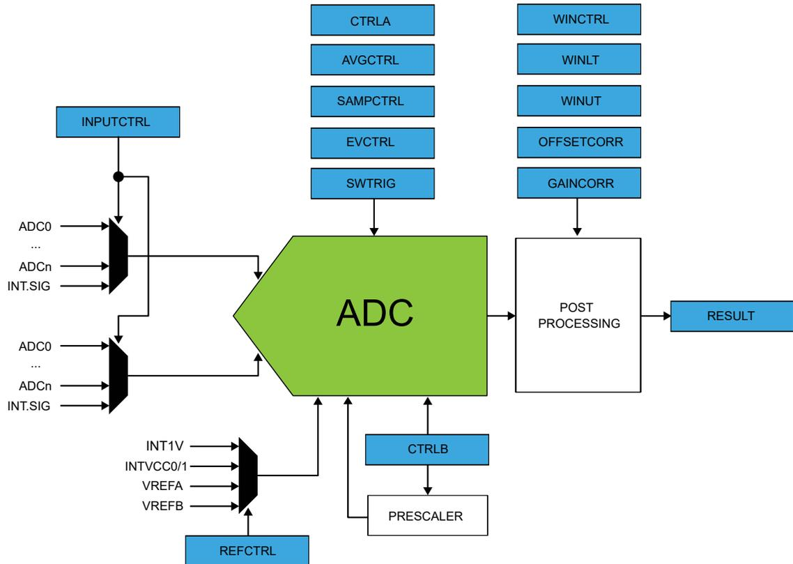
**Note:** INT1V is the buffered internal reference of 1.0V, derived from the internal 1.1V bandgap reference.
