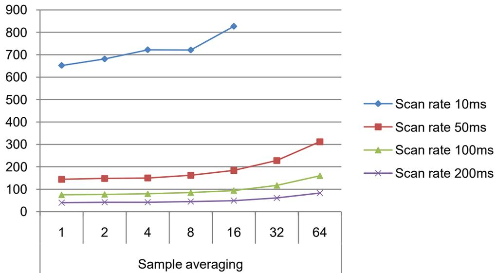
**Figure 41-11. Power Consumption [ $\mu\text{A}$ ]**
