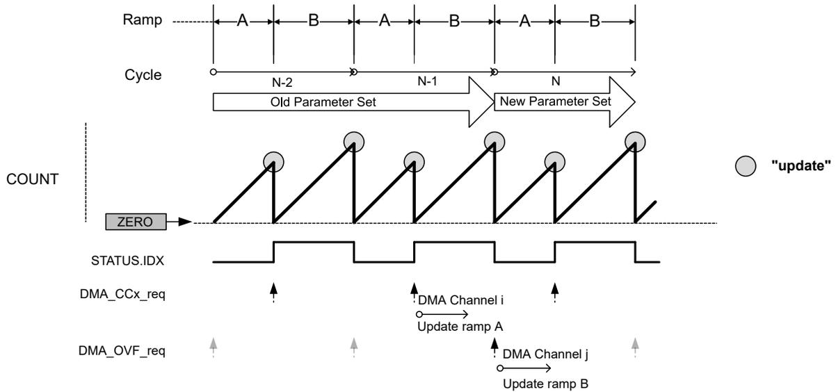
**DMA Operation with Circular Buffer in DS BOTH Mode**
