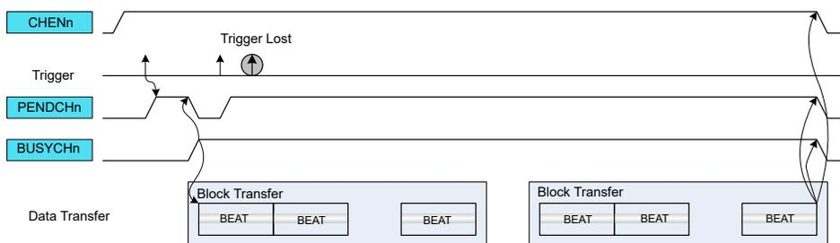
If the trigger source generates a transfer request for a channel during an ongoing transfer, the new transfer request will be kept pending ( $CHSTATUS.PEND=1$ ), and the new transfer can start after the ongoing one is done. Only one pending transfer can be kept per channel. If the trigger source generates more transfer requests while one is already pending, the additional ones will be lost. All channels pending status flags are also available in the Pending Channels register (PENDCH).
