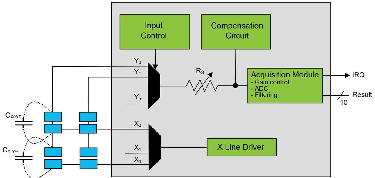
**Note:** For SAM D21 the  $R_S = 0, 20, 50, 100 \text{ K}\Omega$ .
