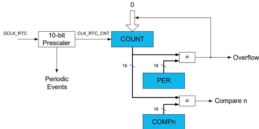
**Figure 19-3. RTC Block Diagram (Mode 2 — Clock/Calendar)**
