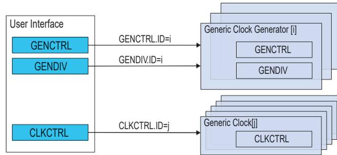
Writing these registers is done by setting the corresponding ID bit group. To read a register, the user must write the ID of the channel, *i*, in the corresponding register. The value of the register for the corresponding ID is available in the user interface by a read access.
