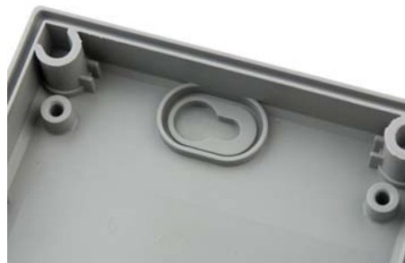
Prepared contour on the inside for wall mounting (can be penetrated with a standard tool).
