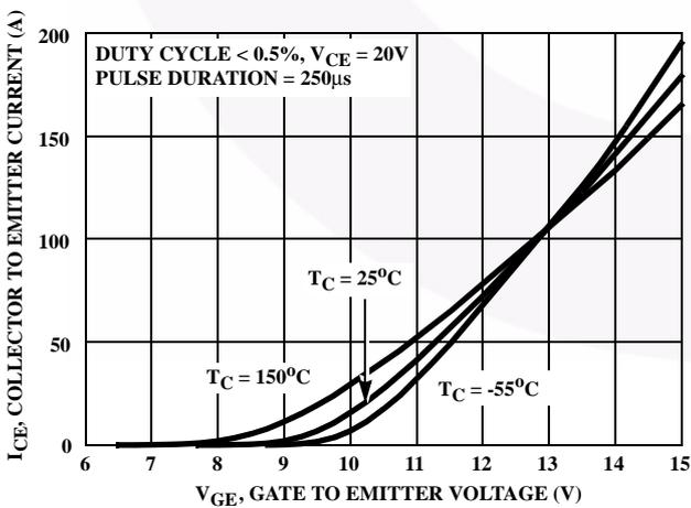
FIGURE 13. TRANSFER CHARACTERISTIC
